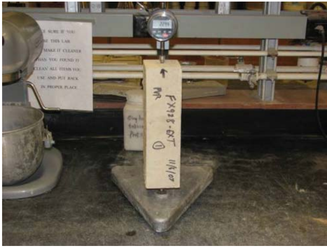
Figure 3.7 Free shrinkage measurements.
