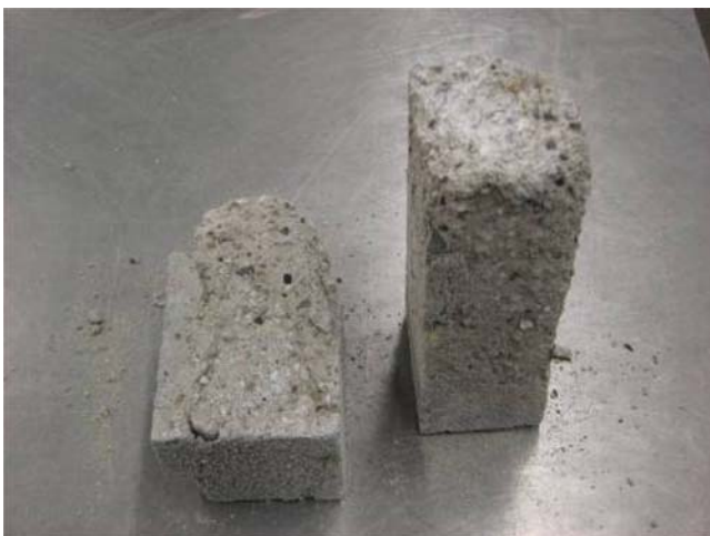
Figure 8.2 SET 45-R specimens after 30 F-T cycles.
