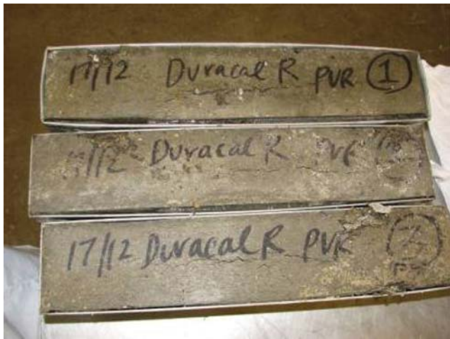
Figure 4.21 Appearance of Dur-R after 35 F-T cycles.
