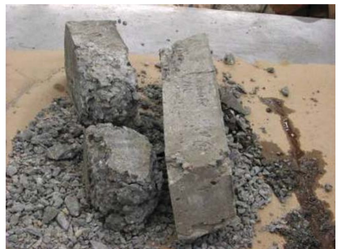
Figure 4.20 Appearance of TR after 35 F-T cycles.
