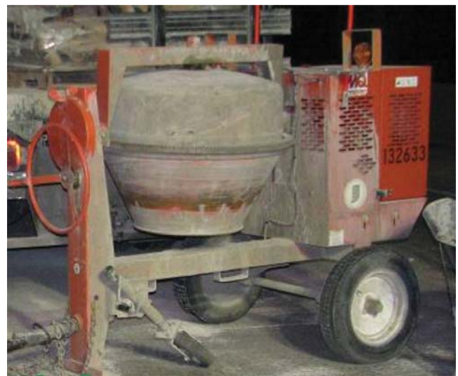
Figure 5.10 Drum mixer used on-site.
