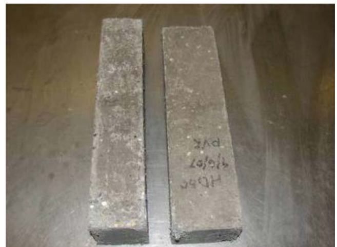
Figure 4.19 Appearance of HD after 300 F-T cycles.
