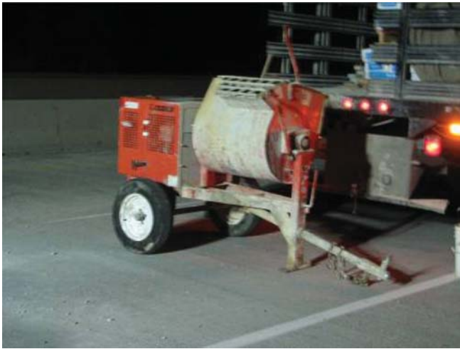
Figure 5.11 Mortar mixer used on-site for SET 45.
