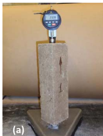
Figure 6.4 Free shrinkage measurement setup (a) and shrinkage results (b) for PCW mixtures with 31% of water.
