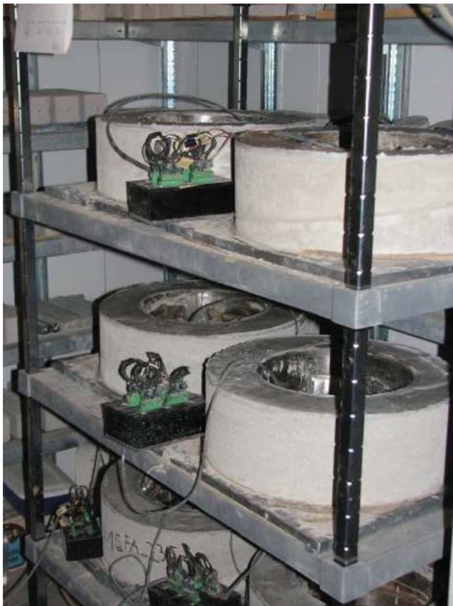
Figure 3.8 Restrained shrinkage test.
