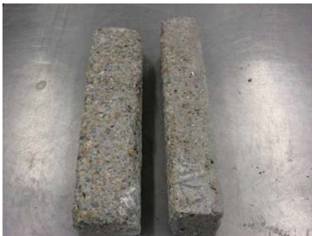
Figure 4.22 Appearance of Dur-AE after 35 F-T cycles.
