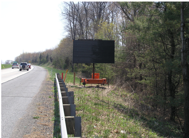
Portable VMS – Trailer-mounted on concrete pad
