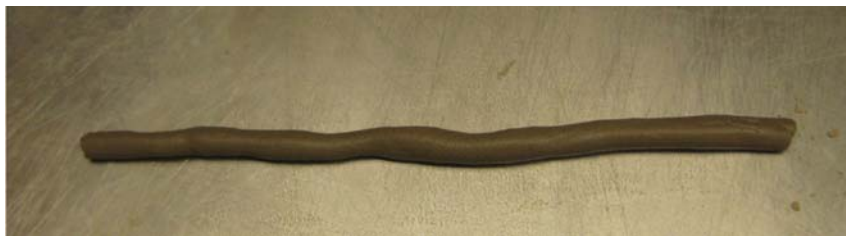
Figure 5.8 Photograph of a plastic limit test.
