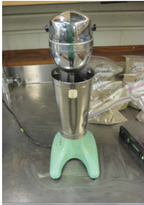
Figure 5.4 A photograph, on the left, of the soil solution being amalgamated with the electric mixer and a photograph, on the right, of the hydrometer placed in the soil solution.
