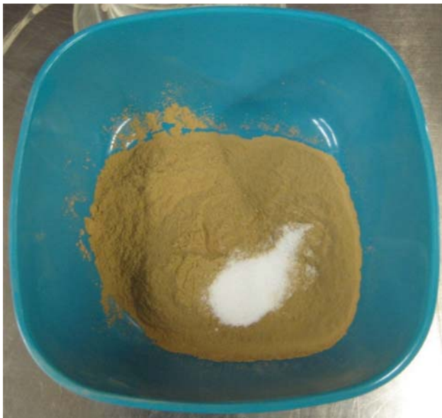
Figure 5.3 Photograph of 50 grams of soil passing a #200 sieve with 5 grams of anti-flocculation agent, Sodium Hexametaphosphate.
