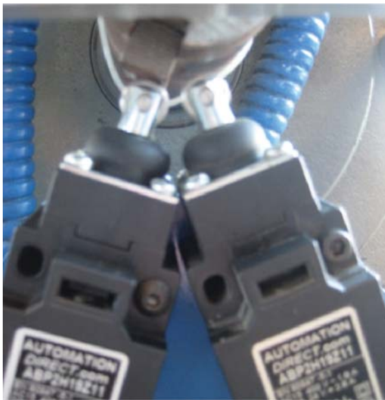
Figure 3.5 Original position limit switch engaged.
