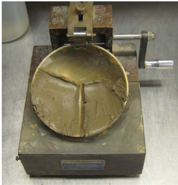
Figure 5.7 Photograph of a liquid limit test.
