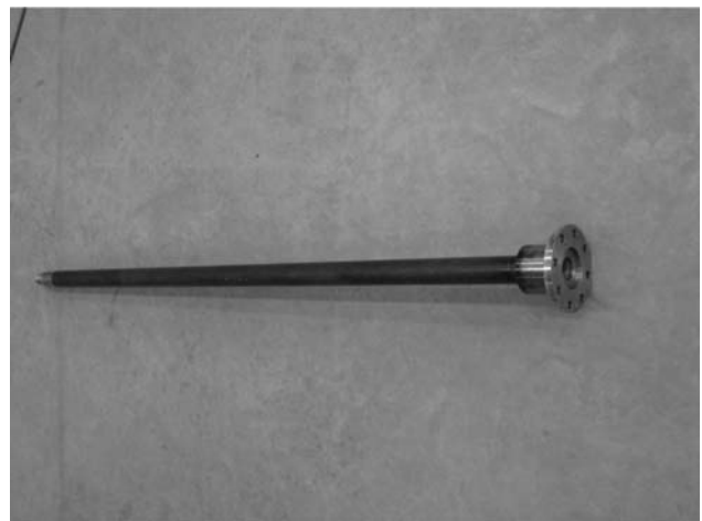
Figure 3.3 Drill rod adaptor.
