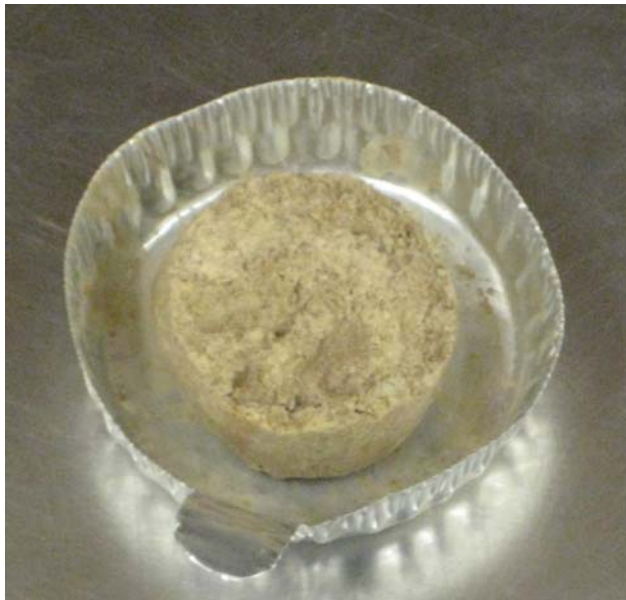
Figure 5.5 Photograph of a soil sample in a water content container.
