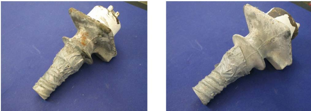
Figure 6.9: Underside View of Anchorage with Non-Galvanized Bearing Plate (Left) and Galvanized Bearing Plate (Right)
