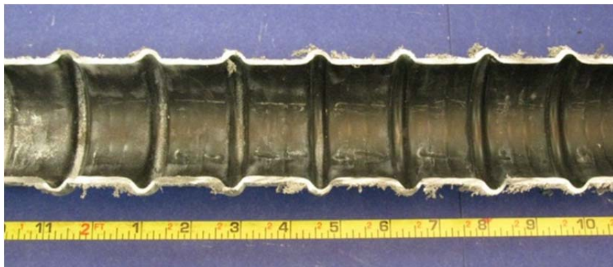
Figure 5.60: Specimen 3.4 Strand Gouging on Bottom of North Duct
