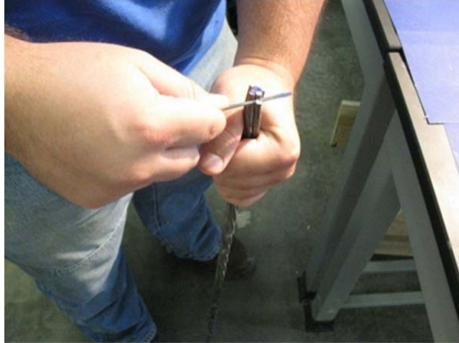
Figure 5.4: Using Screwdriver to Unravel Strand
