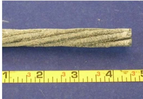
Figure 5.52: Specimen 3.2, Bubbles in Interstices of Galvanized Strand
