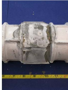
Figure 5.43: Specimen 3.1 Cement Paste and Large Aggregate Embedded in North Grout
