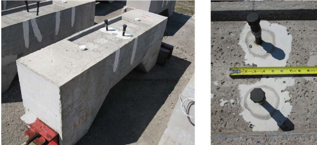
Figure 5.8: Specimen T.1 Overall (Right) and Grout Vents (Left)
