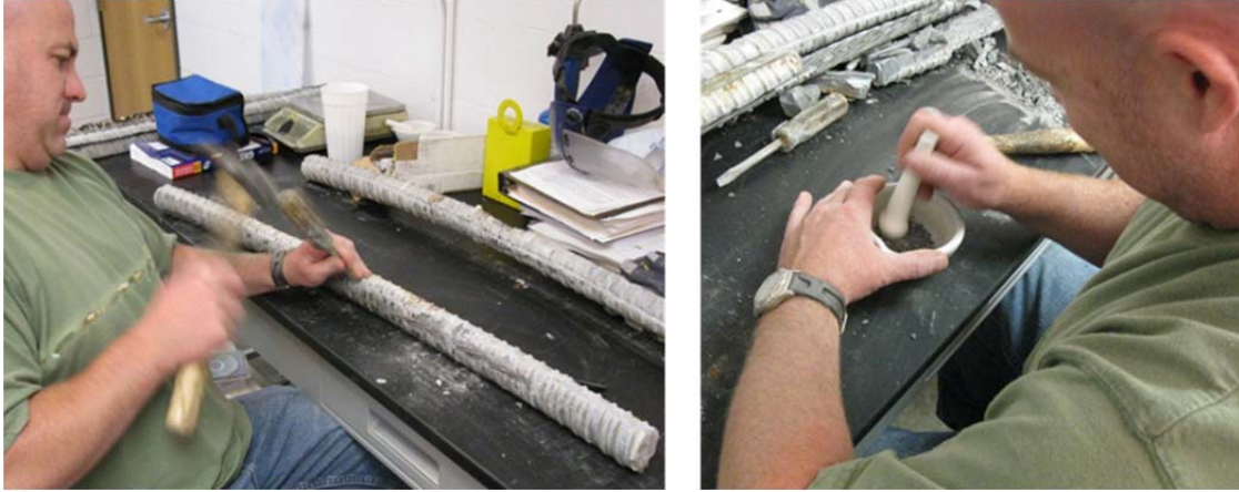
Figure 3.8: Grout Chloride Sample Extraction (Left) and Grinding (Right)
