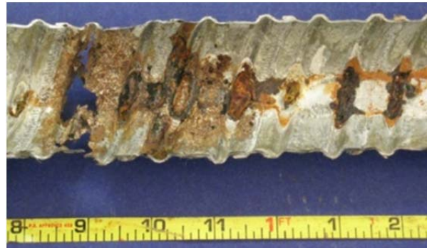
Figure 5.23: Specimen 1.2, Area Loss and Large Void on Top Inner Surface of North Duct
