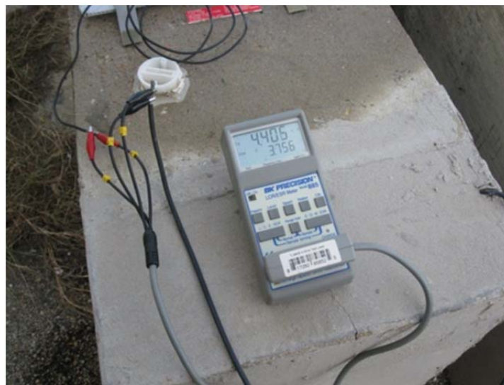
Figure 3.5: LCR Meter Connected to Specimen to Measure AC Impedance
