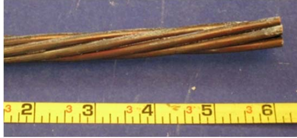
Figure 5.25: Specimen 1.2, Possible Dezincification
