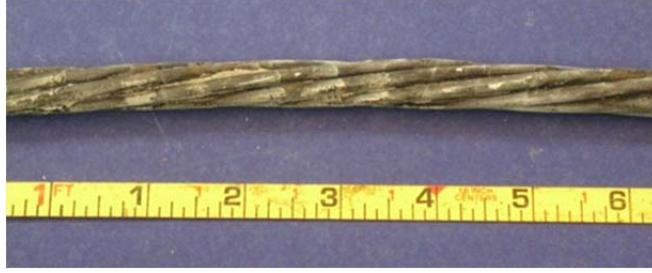
Figure 5.37: Specimen 2.4, Lines in Strand Discoloration
