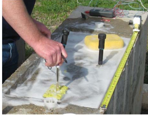
Figure 3.2: Half-Cell Potential Measurements in Progress
