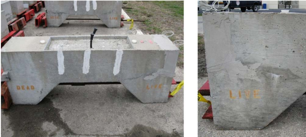
Figure 5.50: Specimen 3.2 Overall (Left) and Efflorescence at Live End Corbel Crack
