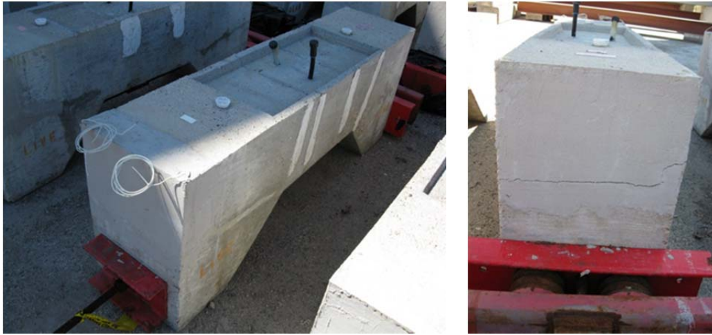
Figure 5.34: Specimen 2.4 Overall (Left) and Cracking at Dead End Pourback (Right)
