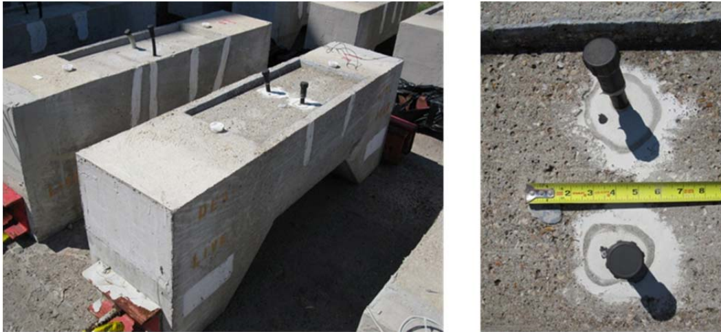
Figure 5.14: Specimen T.2 Overall (Left) and Grout Vents (Right)
