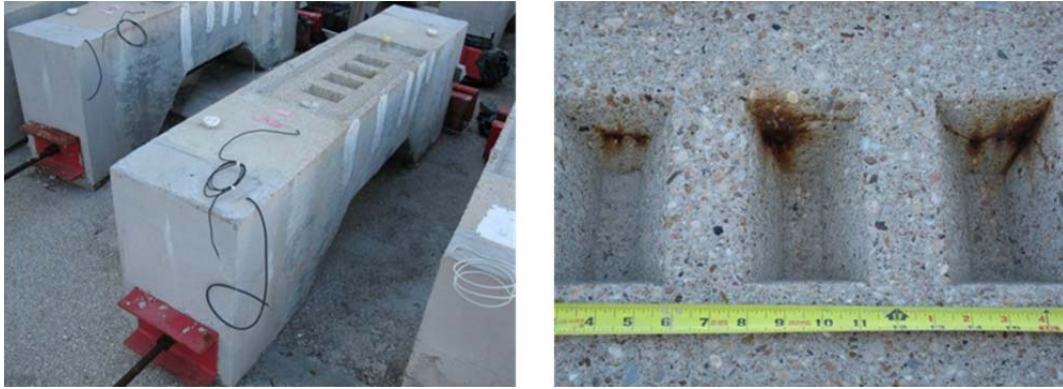
Figure 5.71: Specimen 7.1 Overall (Left) and Corrosion Staining in Saltwater Tray Wells (Right)
