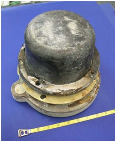
Figure 5.75: Specimen 7.1 Anchorage Components, from Top: Grout Cap, Retaining Ring, Insulation Plate, Bearing Plate
