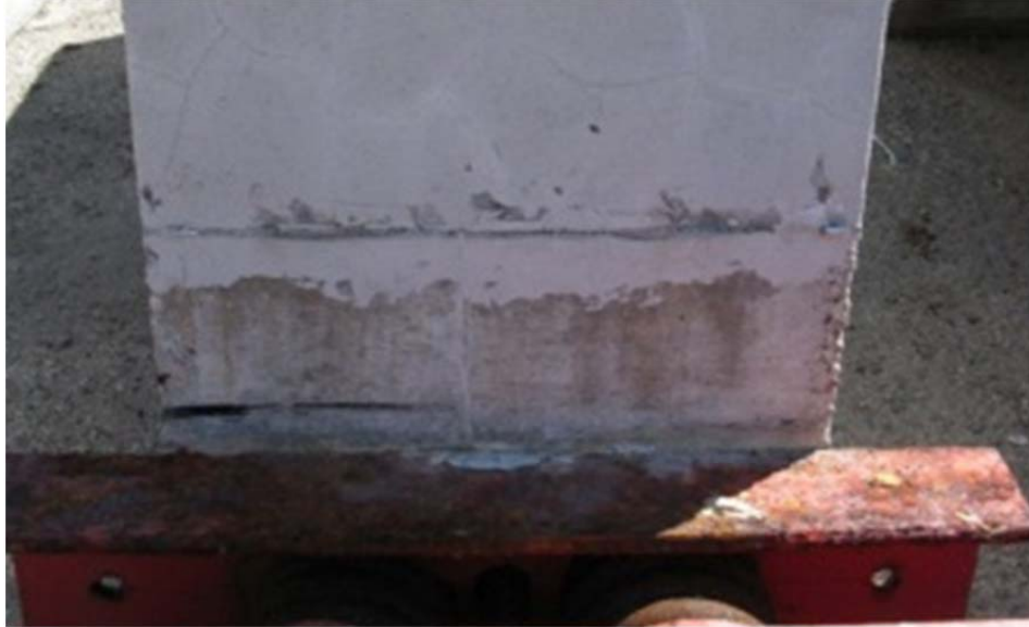
Figure 5.15: Specimen T.2, Separation and Delamination Around Dead End Pourback
