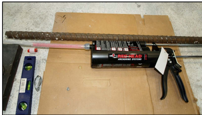
Figure 5.4: Redhead two-part epoxy application system
