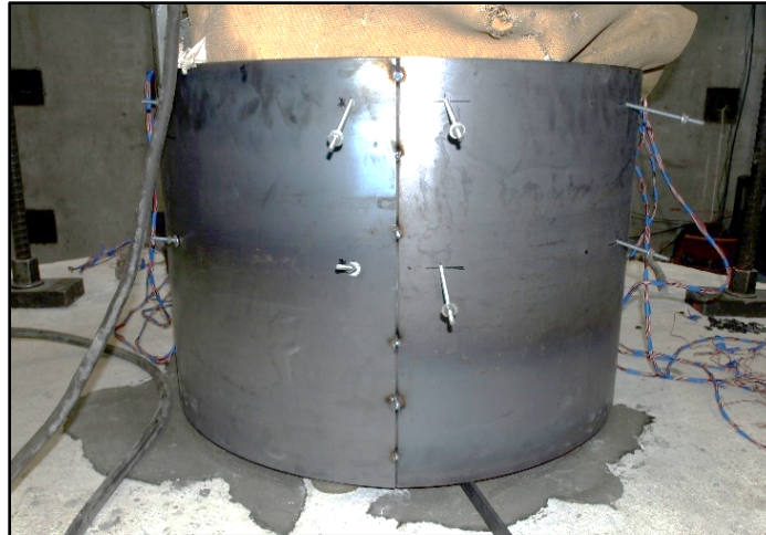
Figure 5.8: Tack welds along seam to hold sleeve and backer bar in place
