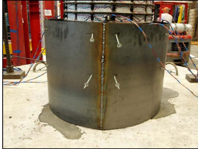
Figure 5.10: Completed butt weld on steel sleeve
