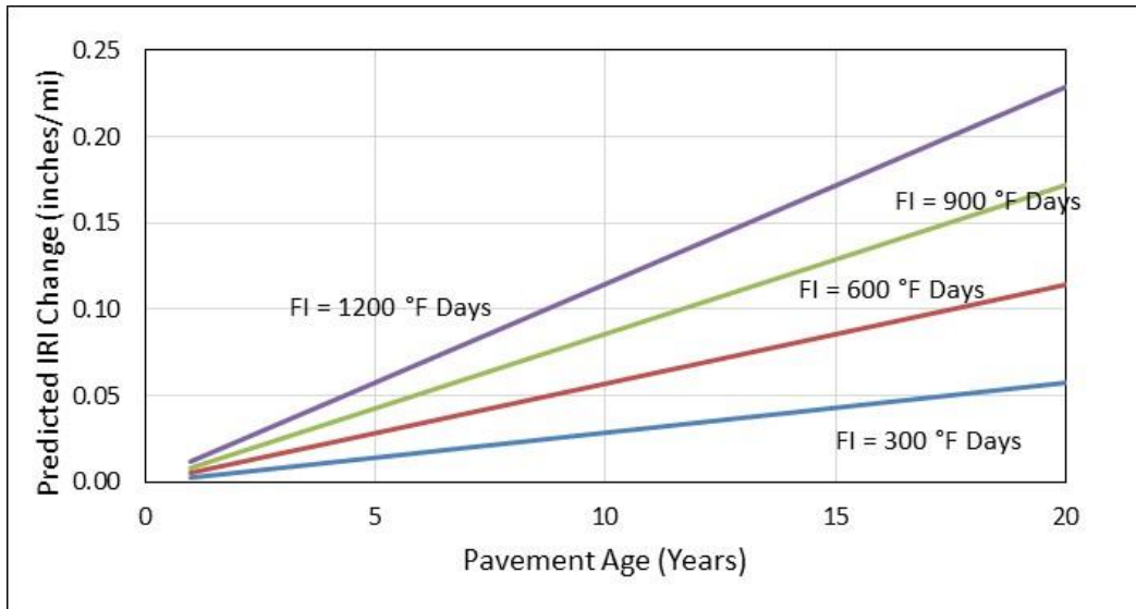
Figure 6. Graph. Increase in IRI due to FI predicted by the MEPDG model for four different average annual FI values.
