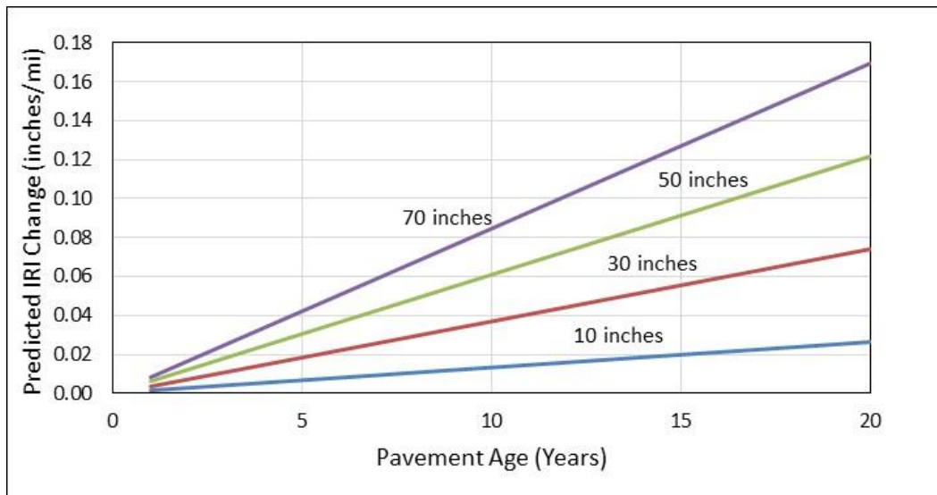
Figure 5. Graph. Increase in IRI due to precipitation predicted by the MEPDG model for four different annual precipitation levels.
