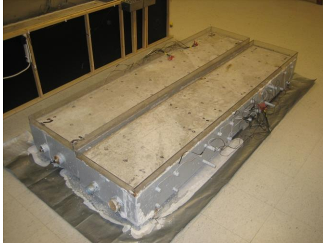
Figure 36. Photo. Concrete slabs with leaking ponding wells.
