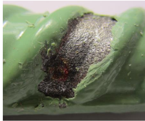
Figure 110. Photo. Extracted ECR from slab 2R with a 2-3 core ID ( [Cl]_{\text{interface@2-inch}} = 1,332 \text{ ppm} ).
