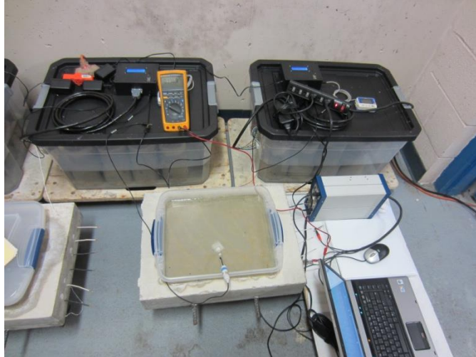
Figure 203. Photo. OCP and I_{macro-cell} measurements of slab #2 specimen.
