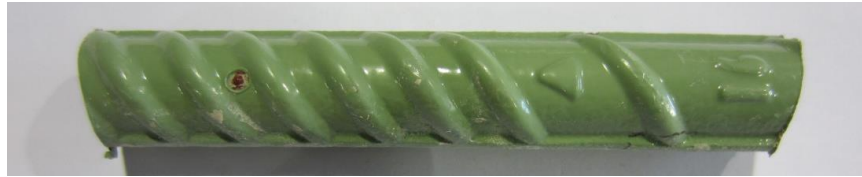
Figure 115. Photo. Extracted ECR from slab 3L with a 2-1 core ID ( [Cl^-]_{\text{interface@2-inch}} = 1,026 ppm).
