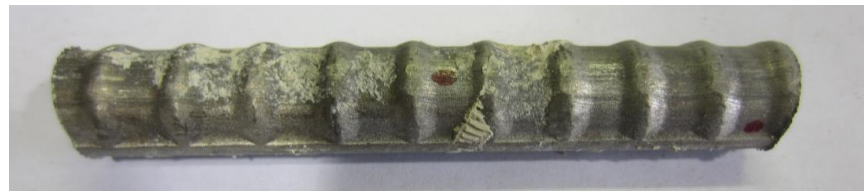
Figure 98. Photo. Extracted SCR1 from slab 2L with a 5-1 core ID ( [Cl^-]_{\text{interface@2-inch}} = 1,114 ppm).
