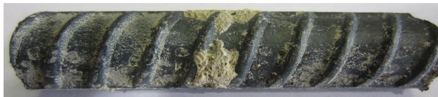
Figure 90. Photo. Extracted black bar from slab 1L with a 2-1 core ID ( [Cl^-]_{\text{interface@2-inch}} = 1,298 ppm).
