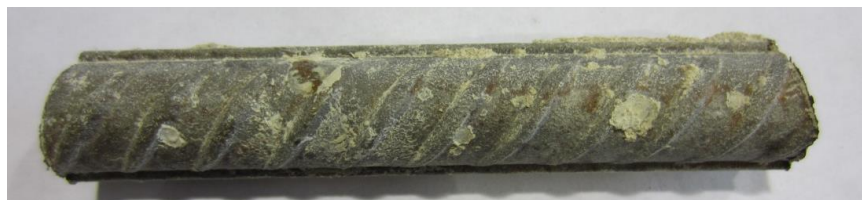
Figure 130. Photo. Extracted LSS2 from slab 4L with a 5-2 core ID ( [Cl^-]_{\text{interface@2-inch}} = 2,713 \text{ ppm} ).
