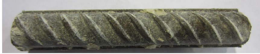
Figure 128. Photo. Extracted LSS2 from slab 4L with a 1-3 core ID ( [Cl^-]_{\text{interface@2-inch}} = 641 \text{ ppm} ).
