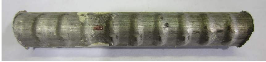
Figure 100. Photo. Extracted SCR1 from slab 2L with a 2-3 core ID ( [Cl^-]_{\text{interface@2-inch}} = 4,265 \text{ ppm} ).
