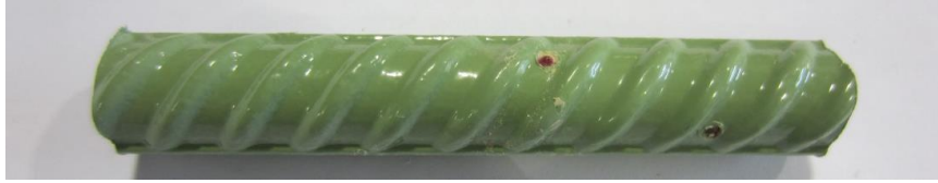
Figure 110. Photo. Extracted ECR from slab 2R with a 2-3 core ID ( [Cl]_{\text{interface@2-inch}} = 1,332 \text{ ppm} ).
