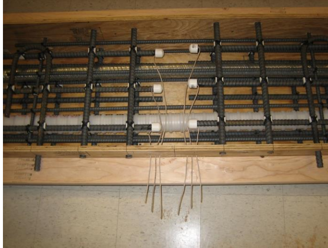
Figure 15. Photo. Electrical wires attached to longitudinal bars.
