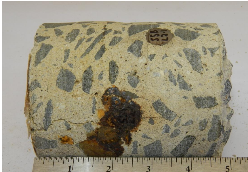
Figure 146. Photo. Cracked slab 5L with a 2-1 core ID ( [\text{Cl}^-]_{\text{interface@2-inch}} = 6,630 ppm).
