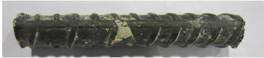
Figure 150. Photo. Extracted SSR1 from slab 5R with a 2-3 core ID ( [Cl^-]_{\text{interface@2-inch}} = 4,153 ppm).
