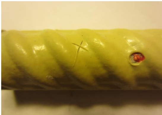
Figure 159. Photo. Extracted DCR from slab 6R with a 1-1 core ID ( [Cl^-]_{\text{interface@2-inch}} = 305 ppm).
