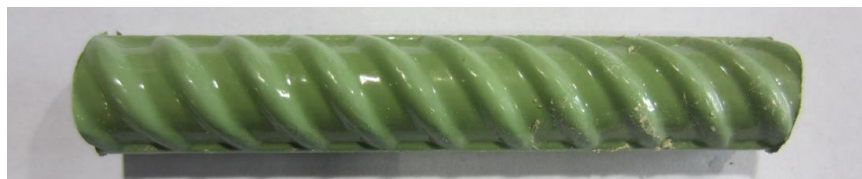
Figure 117. Photo. Extracted ECR from slab 3L with a 6-3 core ID ( [Cl^-]_{\text{interface@2-inch}} = 3,602 ppm).
