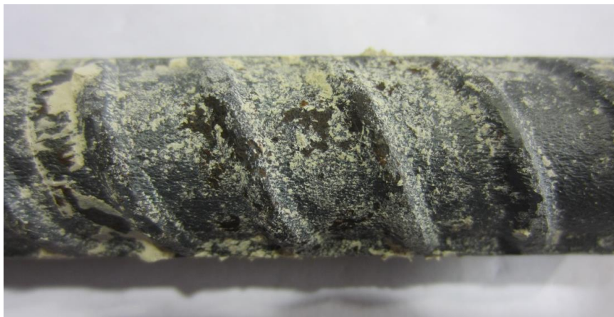
Figure 94. Photo. Extracted black bar from slab 8L with a 1-2 core ID ( [Cl^-]_{\text{interface@2-inch}} = 525 ppm).
