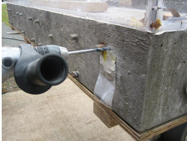
Figure 35. Photo. Chloride sampling at the top mat bar depth.
