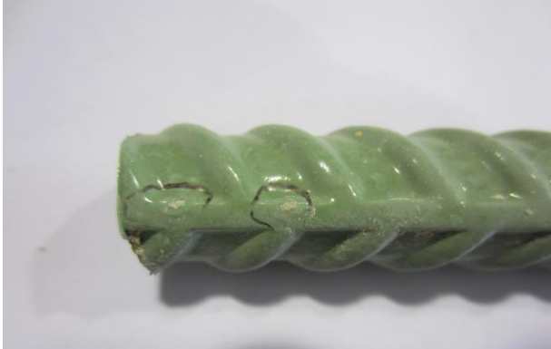
Figure 107. Photo. Extracted ECR from slab 2R with a 5-1 core ID ( [Cl^-]_{\text{interface@2-inch}} = 1,745 \text{ ppm} ).
