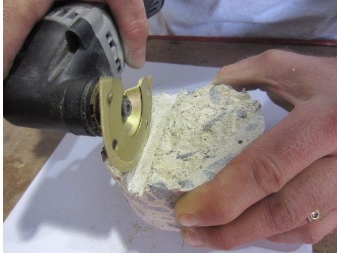
Figure 44. Photo. Concrete powder sampling from upper bar imprint of a core.
