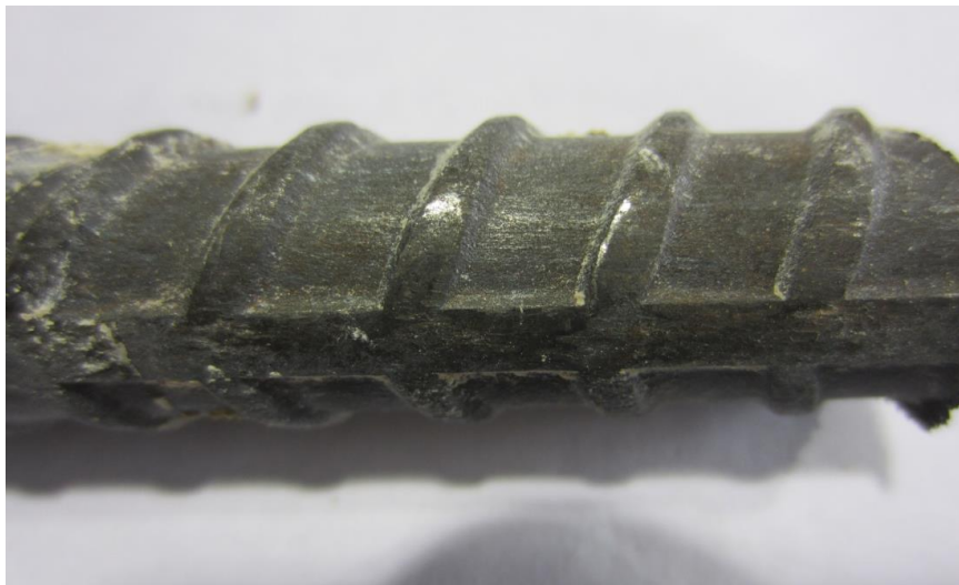
Figure 148. Photo. Extracted SSR1 from slab 5R with a 1-1 core ID ( [Cl^-]_{\text{interface@2-inch}} = 774 ppm).
