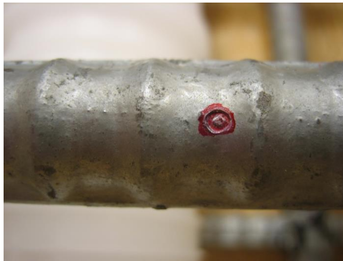
Figure 5. Photo. ECR samples with various types of coating damage.
