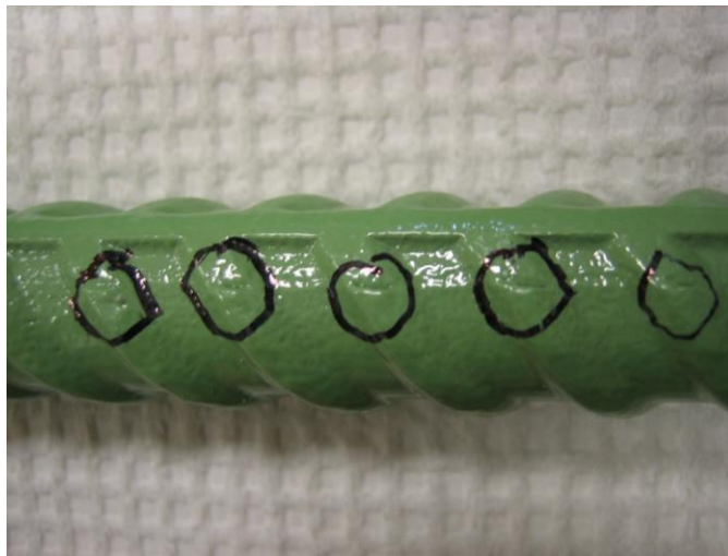
Figure 2. Photo. Example of as-received ECR defects.
