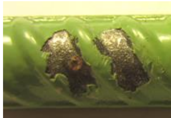
Figure 115. Photo. Extracted ECR from slab 3L with a 2-1 core ID ( [Cl^-]_{\text{interface@2-inch}} = 1,026 ppm).
