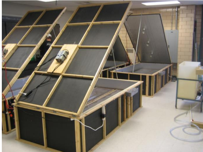
Figure 28. Photo. Opened heat tents during a wetting cycle.
