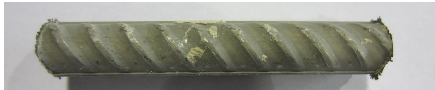
Figure 123. Photo. Extracted SCR2 from slab 3R with a 2-1 core ID ( [\text{Cl}^-]_{\text{interface@2-inch}} = 4,523 ppm).
