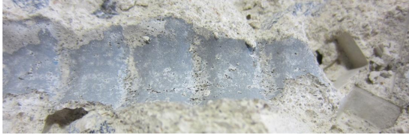
Figure 138. Photo. Bar imprint in slab 4R with a 2-1 core ID ( [Cl^-]_{\text{interface@2-inch}} = 854 \text{ ppm} ).
