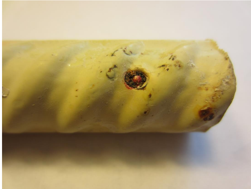
Figure 163. Photo. Extracted DCR from slab 6R with a 1-3 core ID ( [Cl^-]_{interface@2-inch} = 2,138 \text{ ppm} ).
