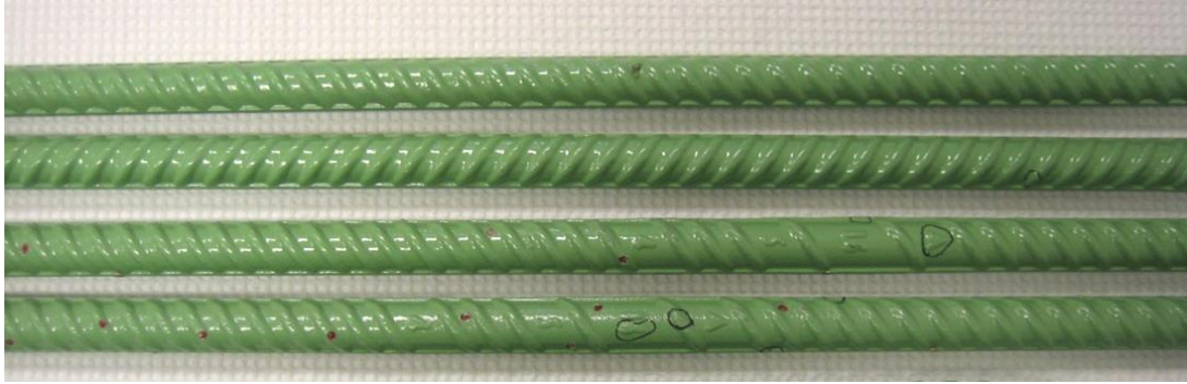
Figure 5. Photo. ECR samples with various types of coating damage.
