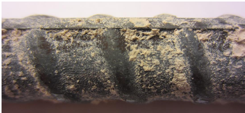
Figure 157. Photo. Extracted LSS1 from slab 6L with a 6-3 core ID ( [Cl^-]_{\text{interface@2-inch}} = 2,936 ppm).
