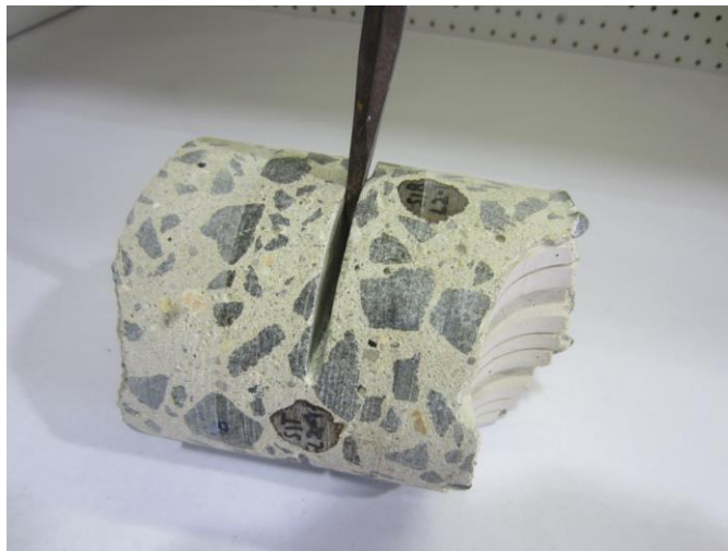
Figure 42. Photo. Splitting a core at the transverse bar depth.
