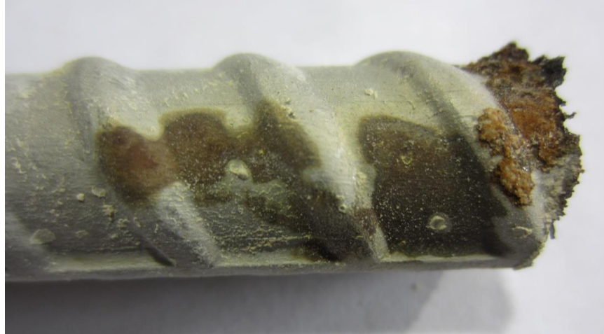
Figure 176. Photo. Powderous corrosion product on an SSR3 bar sample from slab 7R with a 2-3 core ID ( [Cl^-]_{\text{interface@2-inch}} = 4,012 \text{ ppm} ).
