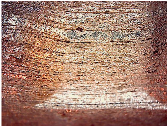
Figure 102. Photo. Rust spot and two pits observed on an SCR1 sample from slab 2L with a 6-1 core ID ( [Cl]_{\text{interface@2-inch}} = 1,578 ppm).
