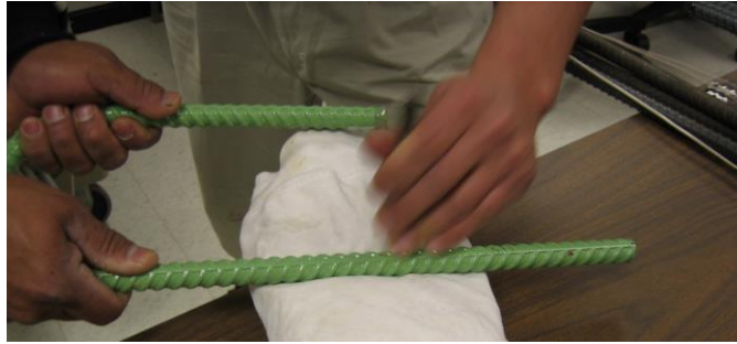
Figure 3. Photo. Creation of artificial coating damage.
