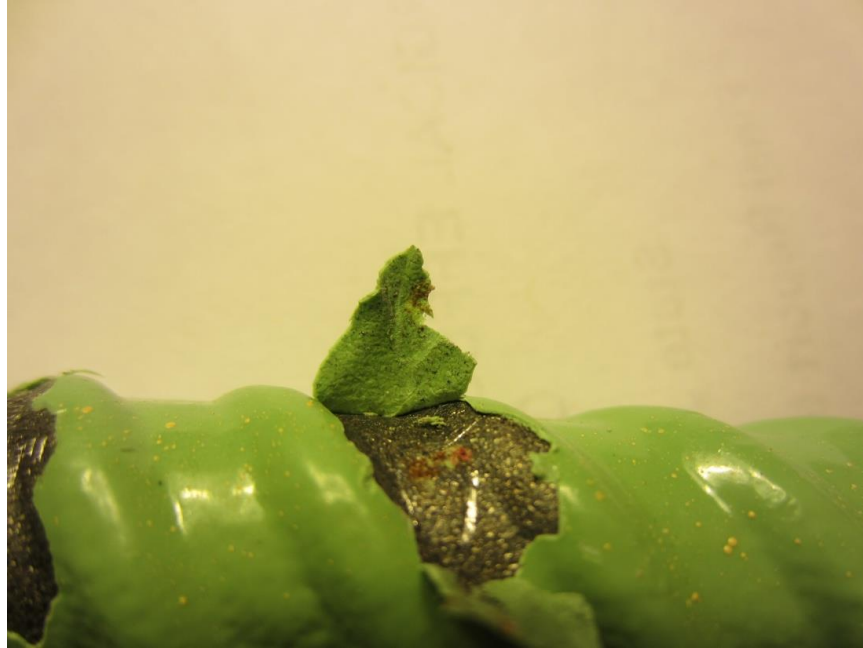
Figure 120. Photo. Coating backside of an ECR from slab 3L with a 5-2 core ID ( [Cl^-]_{\text{interface@2-inch}} = 2,153 ppm).
