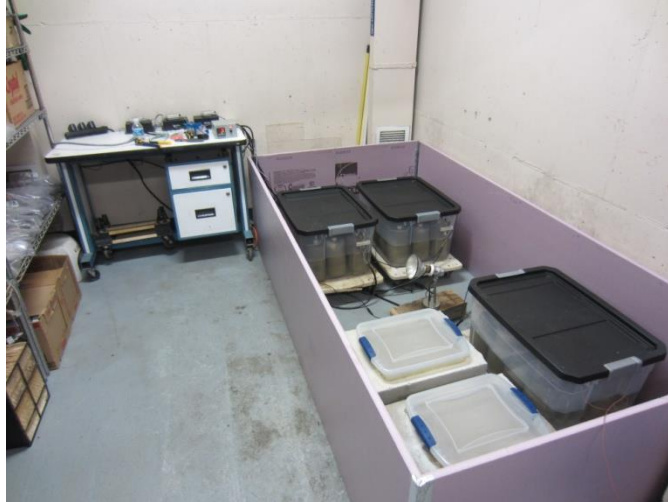
Figure 205. Photo. Arrangement of specimens in a temporary heat tent with lid removed.
