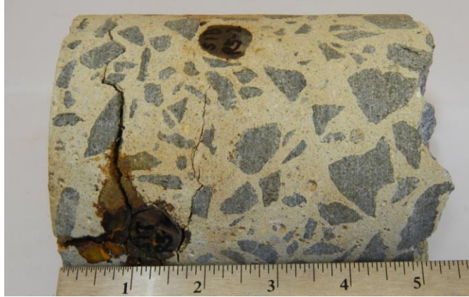
Figure 88. Photo. Corrosion-damaged slab 1R with a 5-2 core ID (black bar at 1-inch cover).
