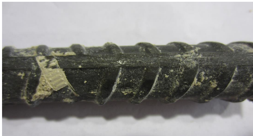
Figure 150. Photo. Extracted SSR1 from slab 5R with a 2-3 core ID ( [Cl^-]_{\text{interface@2-inch}} = 4,153 ppm).
