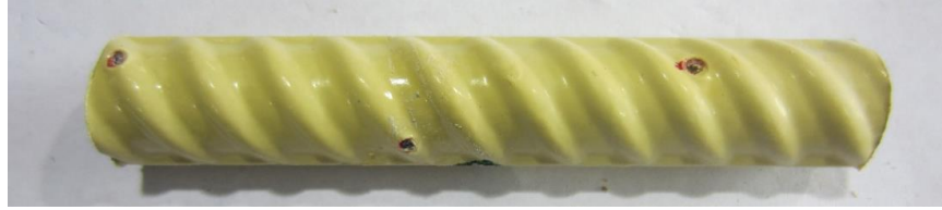
Figure 163. Photo. Extracted DCR from slab 6R with a 1-3 core ID ( [Cl^-]_{interface@2-inch} = 2,138 \text{ ppm} ).
