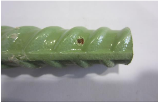
Figure 110. Photo. Extracted ECR from slab 2R with a 2-3 core ID ( [Cl]_{\text{interface@2-inch}} = 1,332 \text{ ppm} ).
