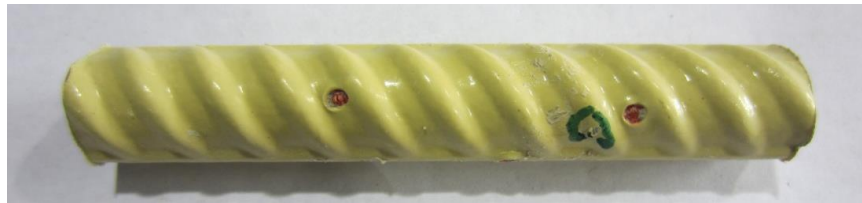
Figure 159. Photo. Extracted DCR from slab 6R with a 1-1 core ID ( [Cl^-]_{\text{interface@2-inch}} = 305 ppm).
