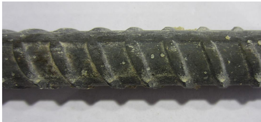
Figure 153. Photo. Corrosion of an SSR1 from slab 5R with a 1-2 core ID ( [Cl^-]_{\text{interface@2-inch}} = 1,841 ppm).
