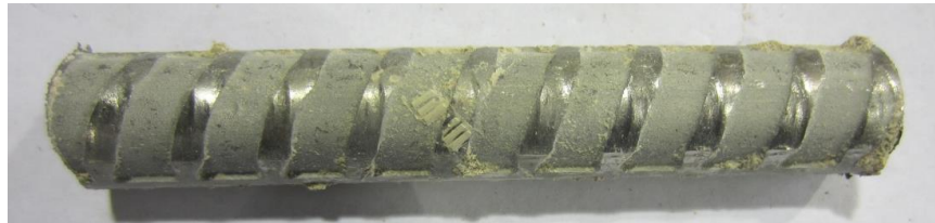
Figure 167. Photo. Extracted SSR2 from slab 7L with a 1-3 core ID ( [Cl^-]_{\text{interface@2-inch}} = 330 ppm).
