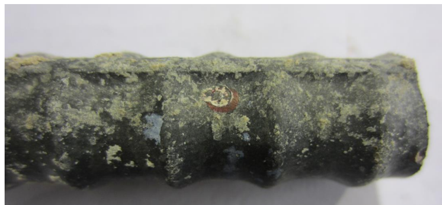
Figure 132. Photo. Extracted HDG from slab 4R with a 1-1 core ID ( [Cl^-]_{\text{interface@2-inch}} = 785 ppm).
