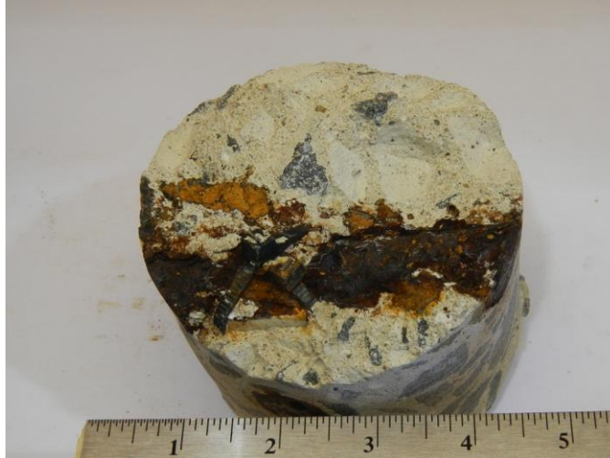
Figure 41. Photo. Documentation of a core's bottom showing a severely corroded black bar.
