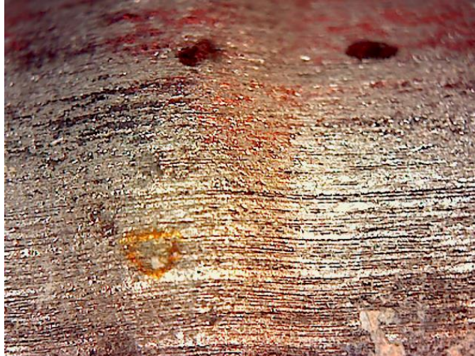
Figure 102. Photo. Rust spot and two pits observed on an SCR1 sample from slab 2L with a 6-1 core ID ( [Cl]_{\text{interface@2-inch}} = 1,578 ppm).
