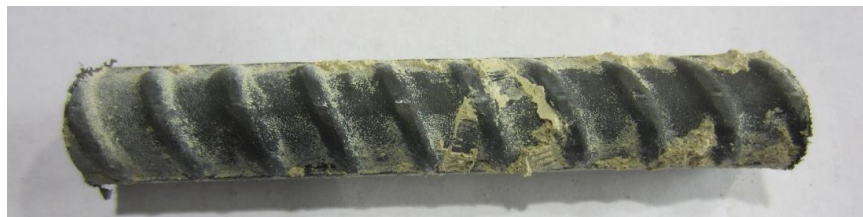
Figure 155. Photo. Extracted LSS1 from slab 6L with a 6-1 core ID ( [Cl^-]_{\text{interface@2-inch}} = 621 ppm).
