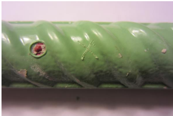
Figure 115. Photo. Extracted ECR from slab 3L with a 2-1 core ID ( [Cl^-]_{\text{interface@2-inch}} = 1,026 ppm).
