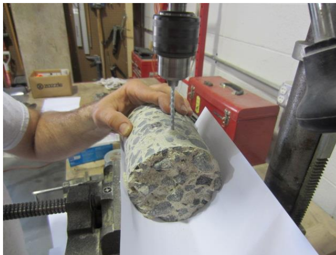
Figure 45. Photo. Concrete powder sampling by drilling.
