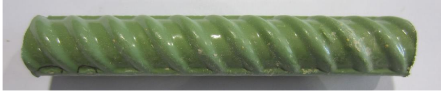
Figure 107. Photo. Extracted ECR from slab 2R with a 5-1 core ID ( [Cl^-]_{\text{interface@2-inch}} = 1,745 \text{ ppm} ).
