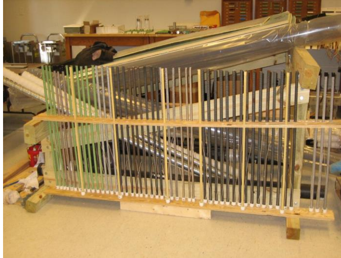
Figure 13. Photo. Encapsulating cut ends of top mat longitudinal bars.
