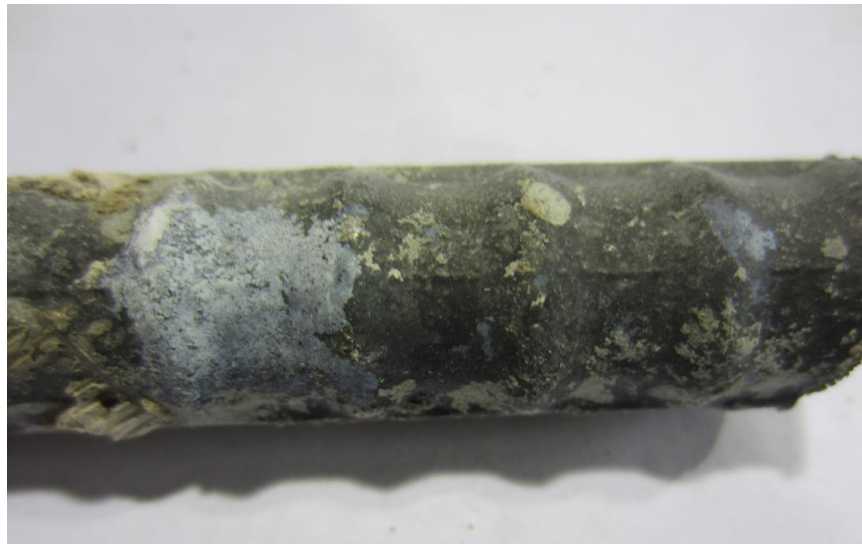
Figure 134. Photo. Extracted HDG from slab 4R with a 6-2 core ID ( [Cl^-]_{\text{interface@2-inch}} = 2,982 ppm).
