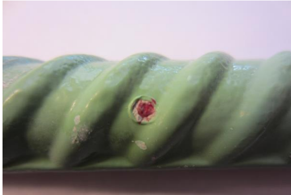
Figure 104. Photo. Extracted ECR from slab 2R with a 1-1 core ID ( [Cl^-]_{\text{interface@2-inch}} = 353 \text{ ppm} ).
