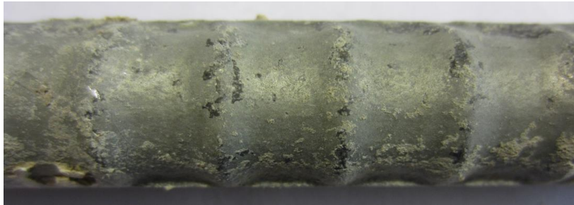
Figure 138. Photo. Bar imprint in slab 4R with a 2-1 core ID ( [Cl^-]_{\text{interface@2-inch}} = 854 \text{ ppm} ).
