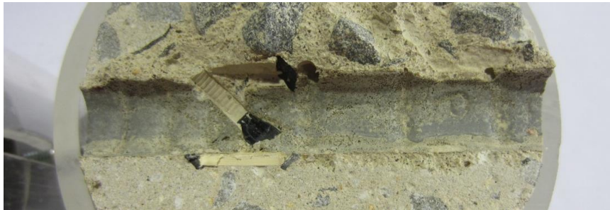
Figure 140. Photo. Rebar imprint in slab 4R with a 2-2 core ID ( [Cl^-]_{\text{interface@2-inch}} = 2,233 \text{ ppm} ).
