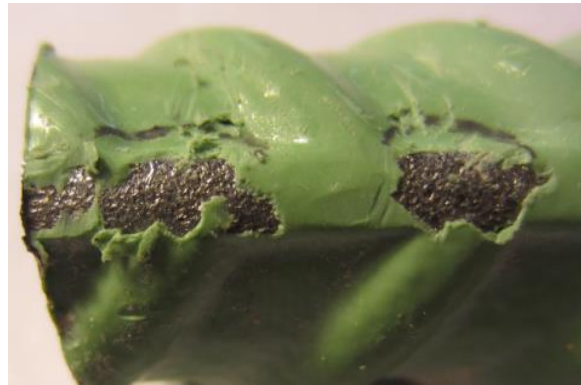
Figure 107. Photo. Extracted ECR from slab 2R with a 5-1 core ID ( [Cl^-]_{\text{interface@2-inch}} = 1,745 \text{ ppm} ).
