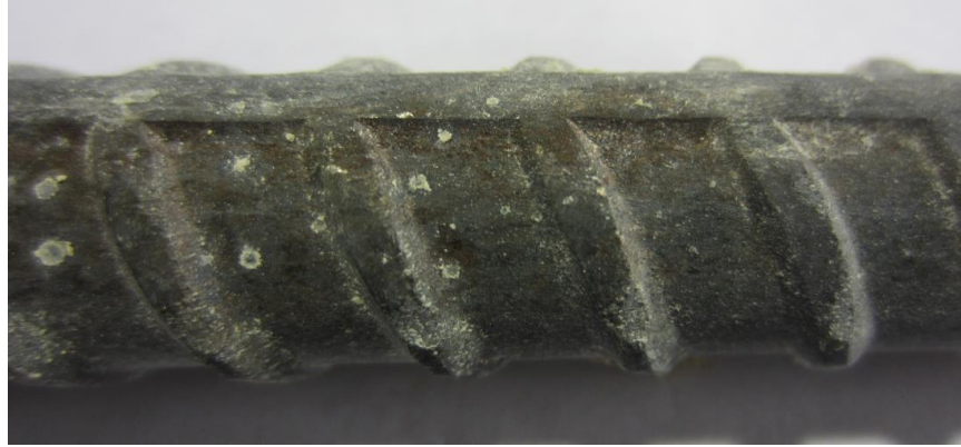
Figure 153. Photo. Corrosion of an SSR1 from slab 5R with a 1-2 core ID ( [Cl^-]_{\text{interface@2-inch}} = 1,841 ppm).
