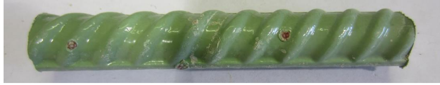
Figure 104. Photo. Extracted ECR from slab 2R with a 1-1 core ID ( [Cl^-]_{\text{interface@2-inch}} = 353 \text{ ppm} ).
