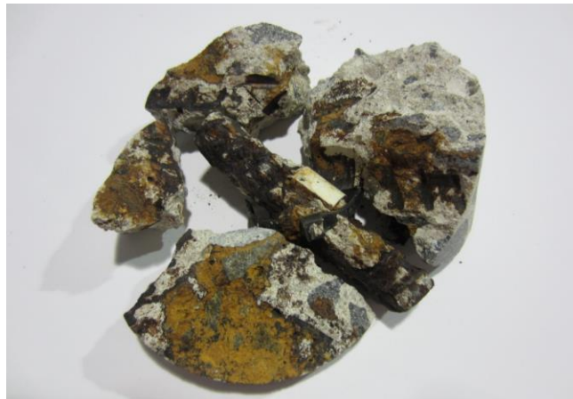
Figure 88. Photo. Corrosion-damaged slab 1R with a 5-2 core ID (black bar at 1-inch cover).
