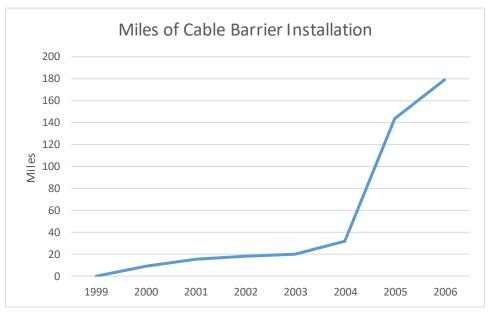
Figure 2. Graph. Miles of cable barrier installation in Missouri.<sup>(3)</sup>
