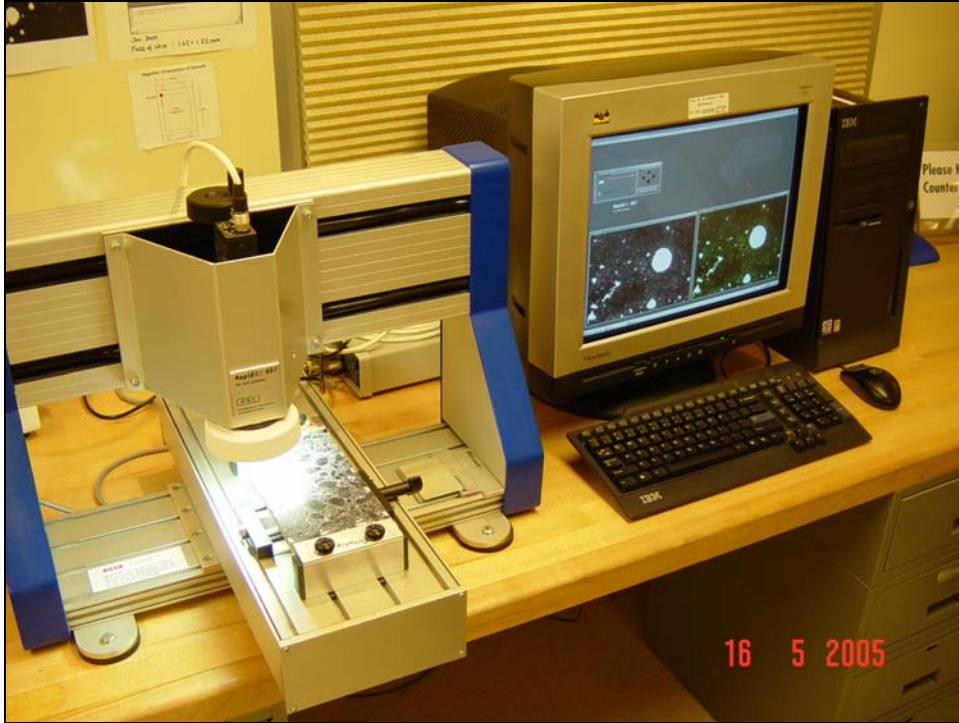
Figure 5-17. Concrete Experts International's RapidAir 457 system
