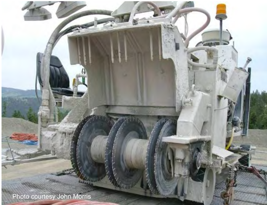
Figure A-11. Cutting equipment for three dowel bar slots per wheelpath.
