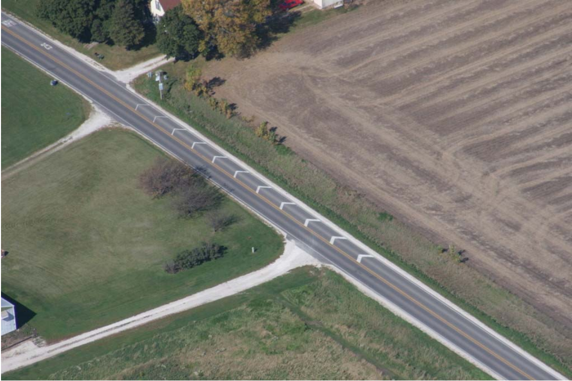
Figure 3.23. Use of converging chevrons in Roland, Iowa
