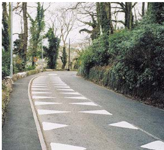
Figure 3.21. Dragon teeth (source: www.cornwall.gov.uk/Transport/trafcalm/calmhome.htm )
