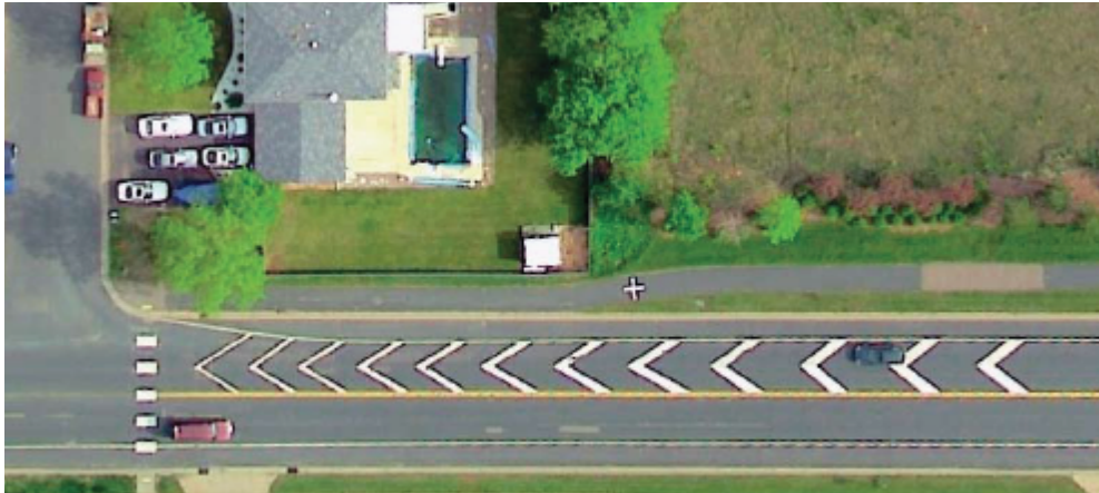
Figure 3.24. Aerial view of chevron lane markings in Eagan, MN (source: Corkle 2001)
