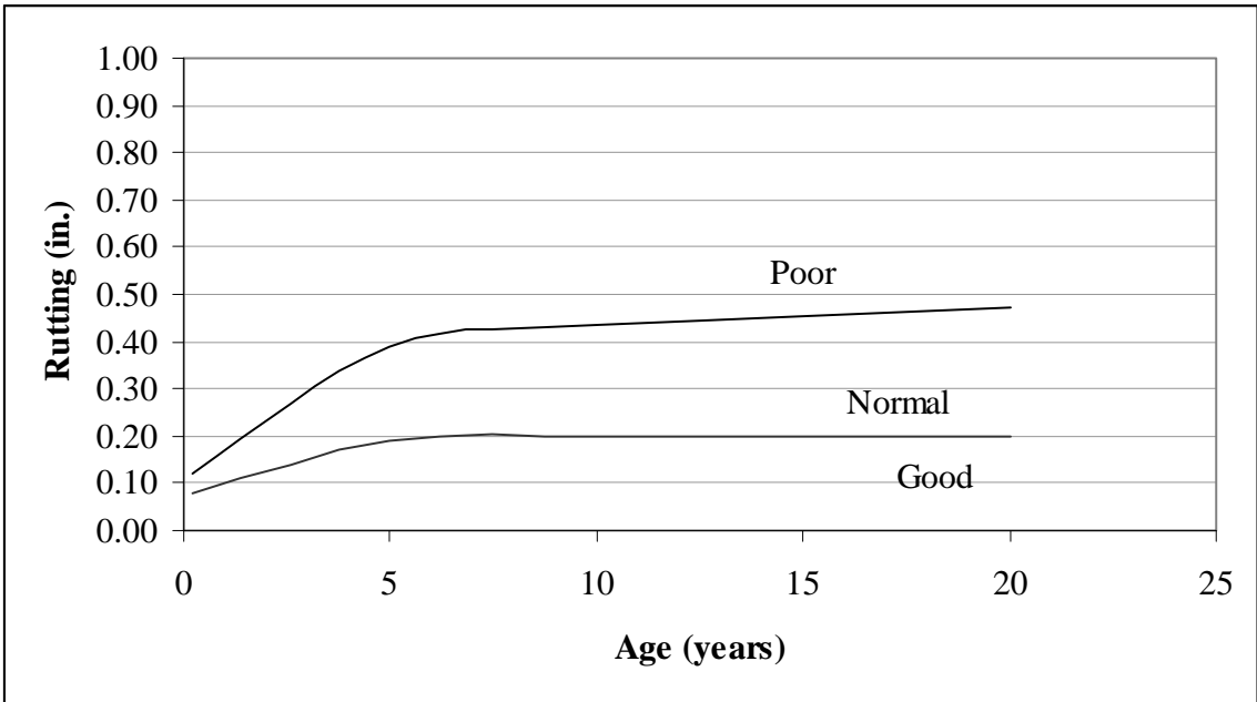
Figure 8.9. Performance criteria for Rutting
