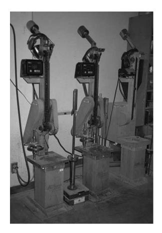
Figure 2.4 Marshall Mechanical Hammer and Pedestal
