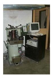
Figure 6.1 A Pine Superpave Gyratory Compactor
