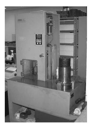
Figure 2.6 Superpave Gyratory Compactor
