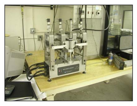
Figure 6.8: IPC UTM 21<sup>©</sup> Beam Fatigue Apparatus
