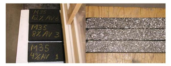
Figure 6.7: Compacted (M-35 Escanaba) and Cut (I-75 Grayling) HMA Samples
