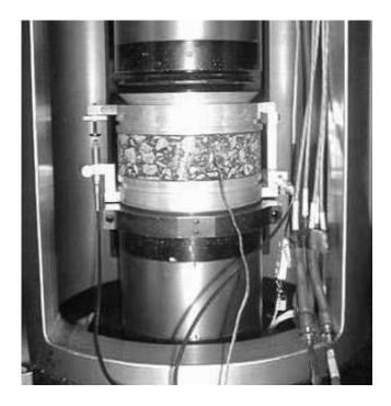
Figure 2.10 Superpave Shear Test Specimen
