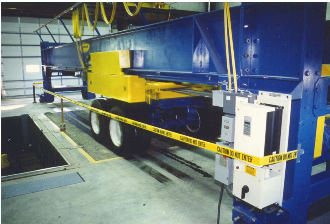
Figure 3.3 Wheel Assembly Completing One Repetition (photo taken by KSU Photographic Services)
