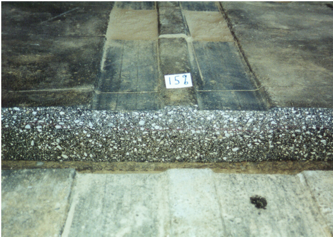
Figure 5.17 Side Wall of Cut Trench in SM-2A Test Section with 15% Sand
