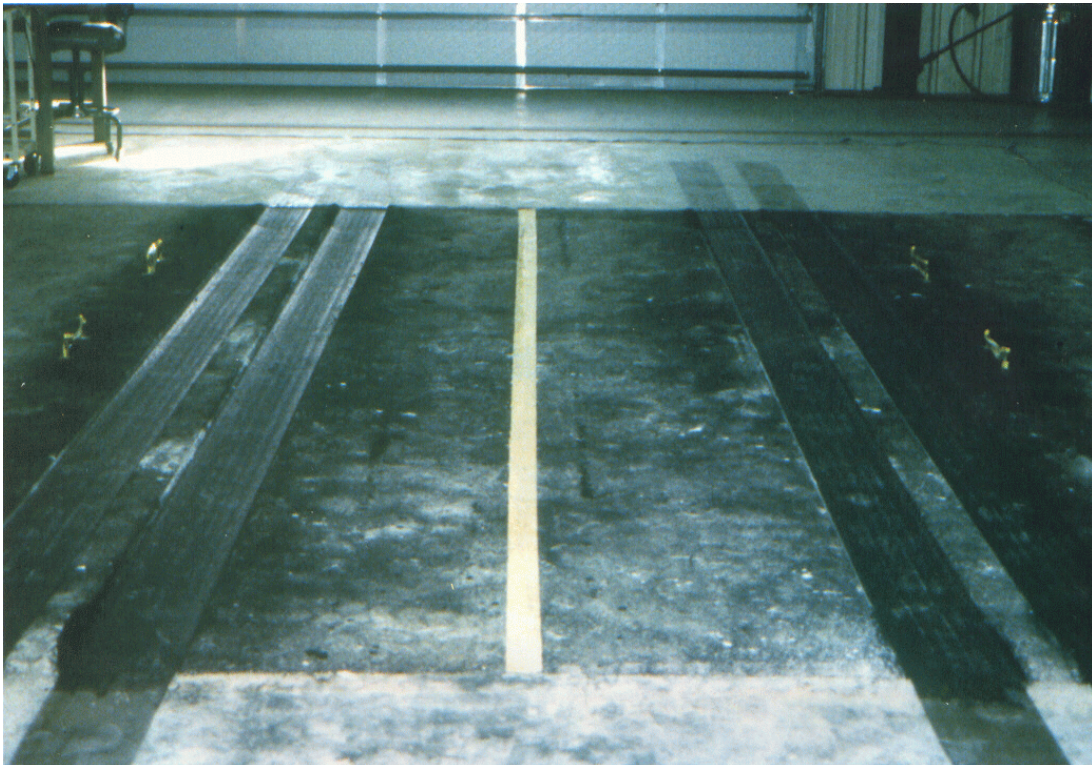
Figure 5.16 Wheel Marks on the Test Sections at the end of 80,000 Load Applications of the ATL 36 Kip-Tandem Axle.
