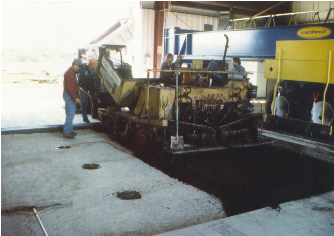
Figure 4.5 Placement of Asphalt Concrete Specimen in Middle Pit of K-ATL
