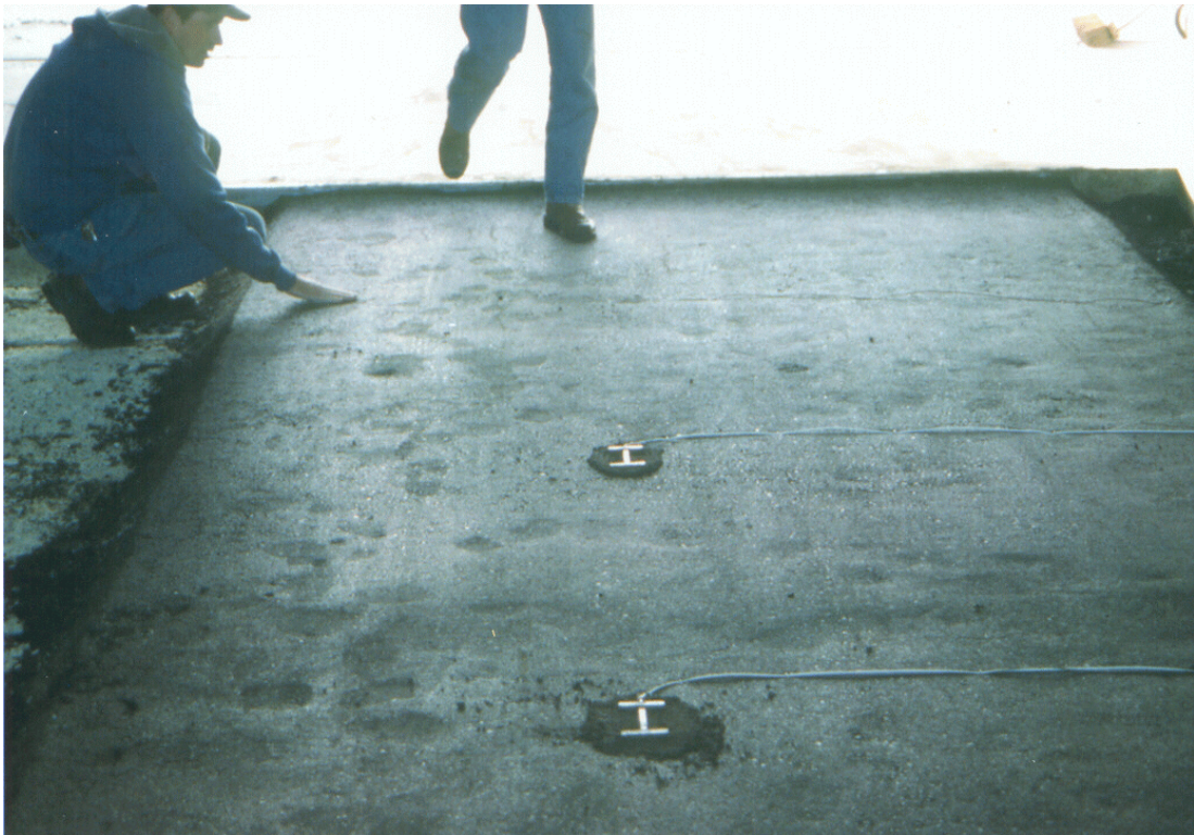
Figure 4.10 Installed Strain Gages at Mid-Depth of Slab
