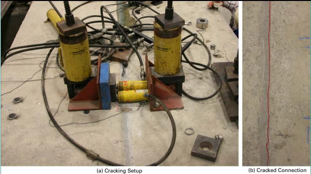
concrete with an exposed aggregate surface finish, failure is likely to occur in the concrete instead of at the interface or in UHPC. This is not true for conventionally grouted connections, as failure often occurs in the interface.
