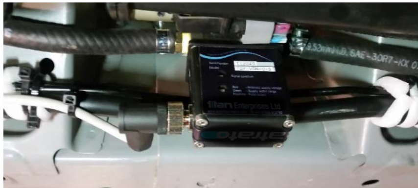
Figure 7. Fuel meter installed at vehicle fuel line.
