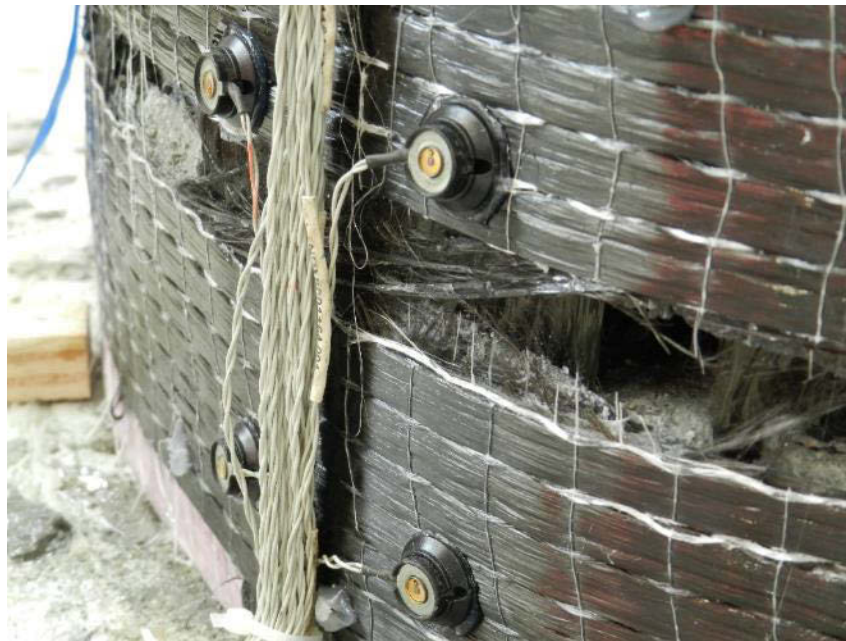
Figure 4.19: Splitting Failure in the Anchor on the Compression Side
