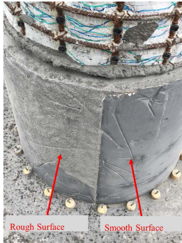
Figure 5.19: Grout Surface Before and After Roughening
