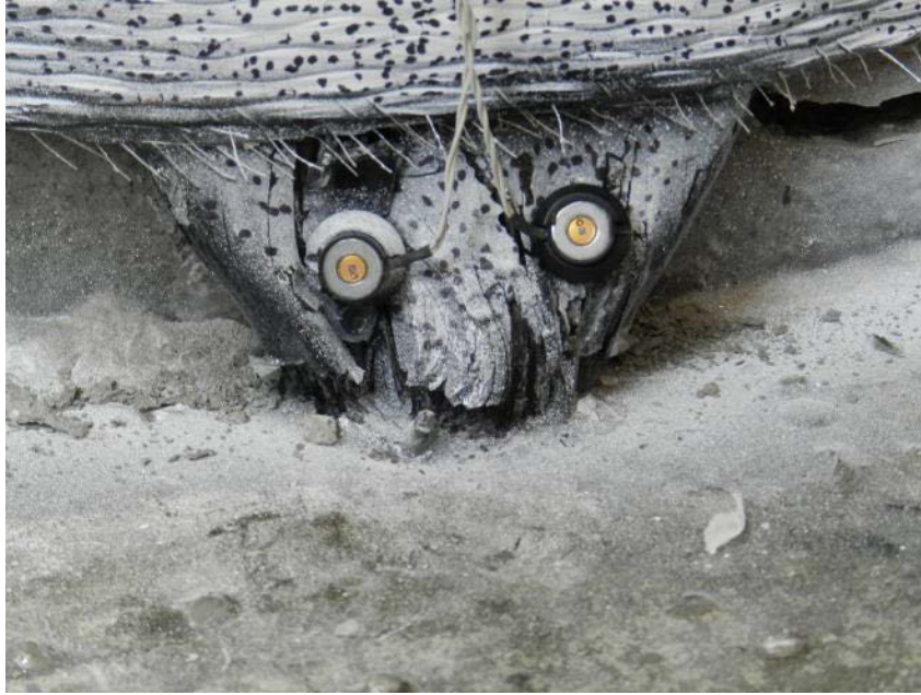
Figure 4.23: Fiber Rupture in the CF Anchor
