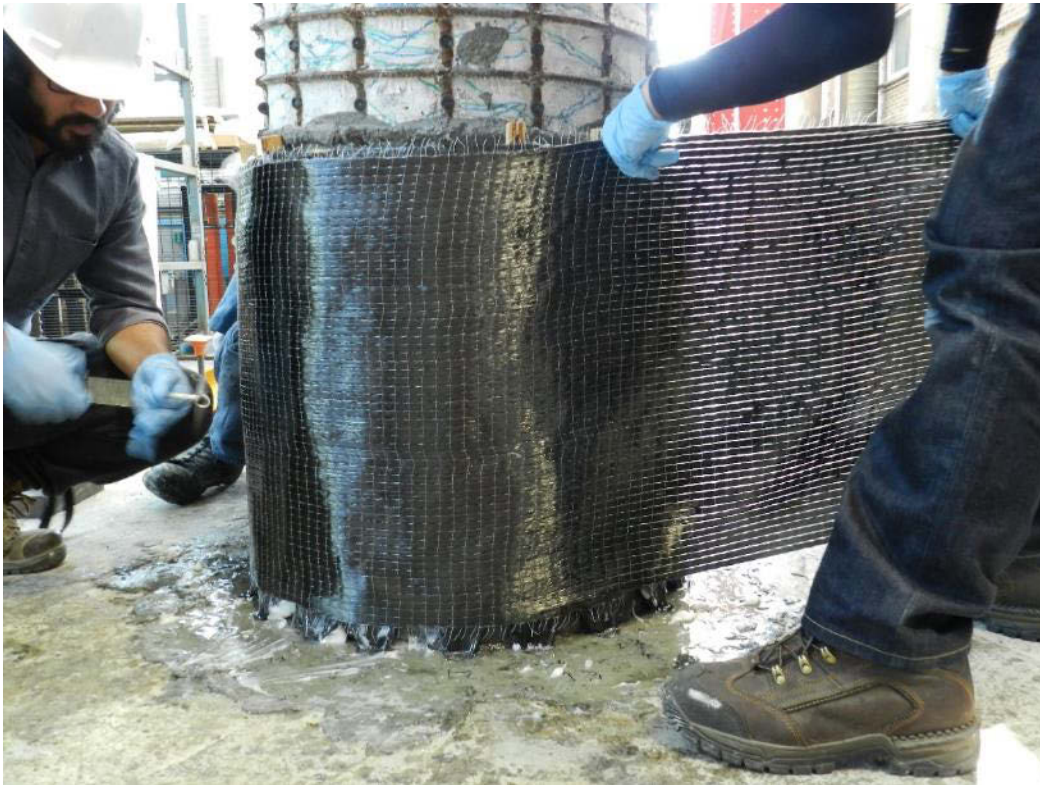
Figure 5.24: Application of Hoop Fiber for C1 Column Specimen
