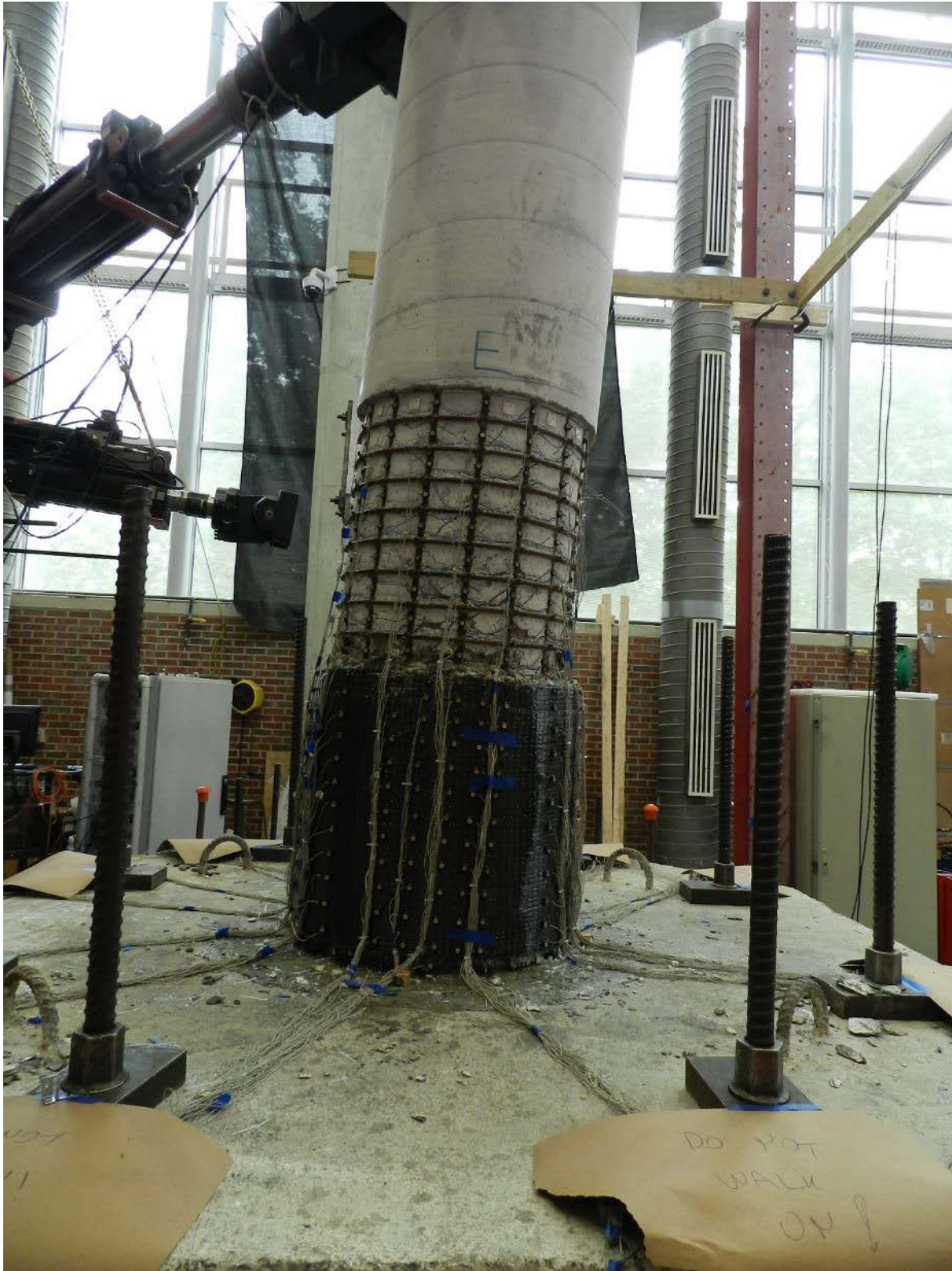
Figure 5.38 : Column Rotation about its Bottom End
