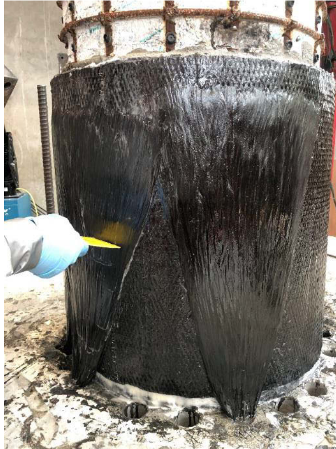
Figure 5.23: Splayed Anchor Fan Fibers
