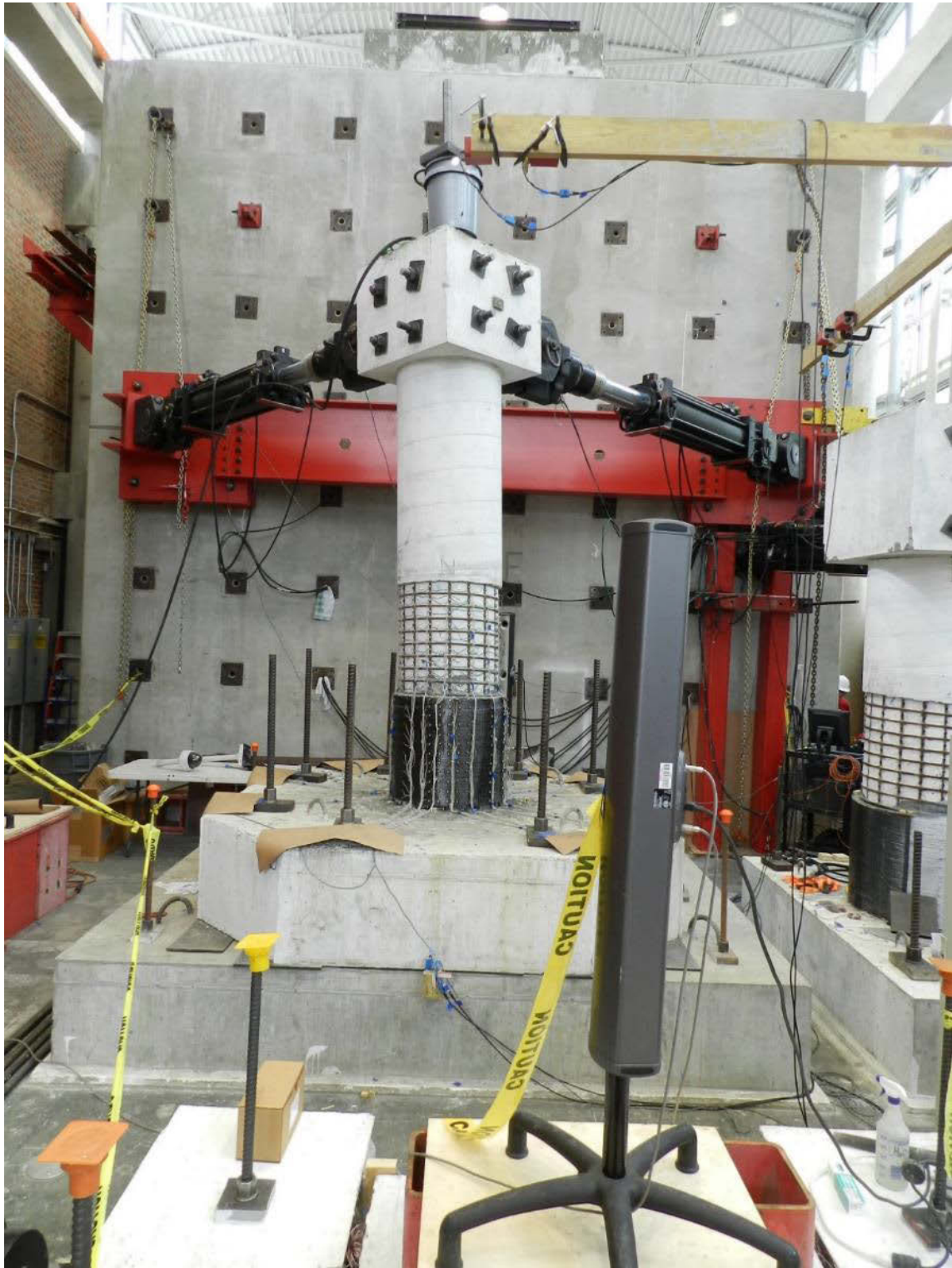
Figure 5.37 : Plastic Hinge Formation above Repair
