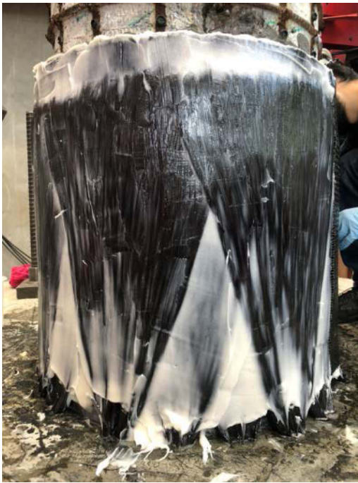
Figure 5.52 : Detail of CFRP Anchor for C2 Column Specimen
