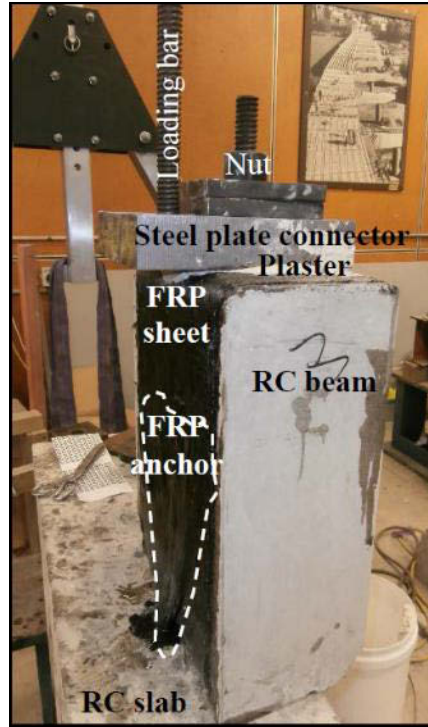
Figure 2.13: Test Setup and Specimen [9]
