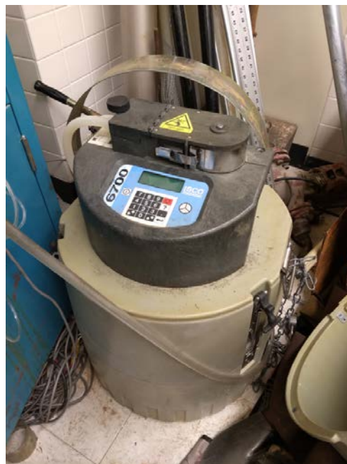
Figure 4- 9: Teledyne ISCO 6700 Autosampler used in turbidity and TSS characterization of samples taken from Soapstone Branch during rain events.
