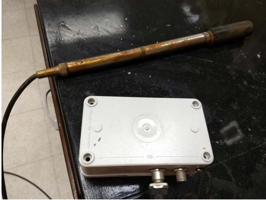
Figure 4- 10: INW Turbo turbidity sensor, with logger box, that was used in the Soapstone Branch sediment characterization. Sediment loading covered the sensor head (black), preventing the correct sensor operation.
