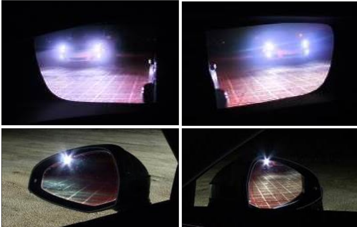
Figure 17. Sedan Positioned 16.4 Feet (5 m) Aft of Rear Bumper at Night Time, as Viewed With Side CMS (top) and Mirrors (bottom) on Driver (left) and Passenger Side (right)
