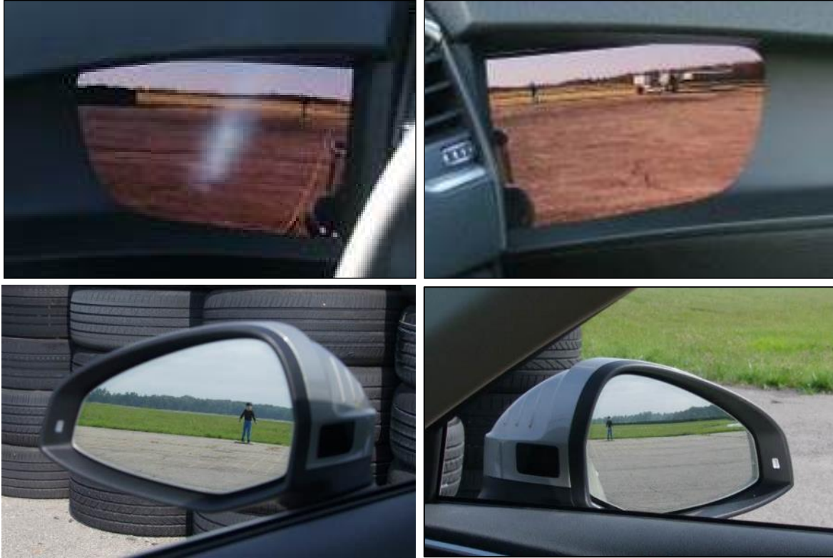
Figure 53. Child Mannequin Positioned 82.0 Feet (25 m) Aft of Rear Bumper, as Viewed With Side CMS (top) and Mirrors (bottom) on Driver (left) and Passenger Side (right)
