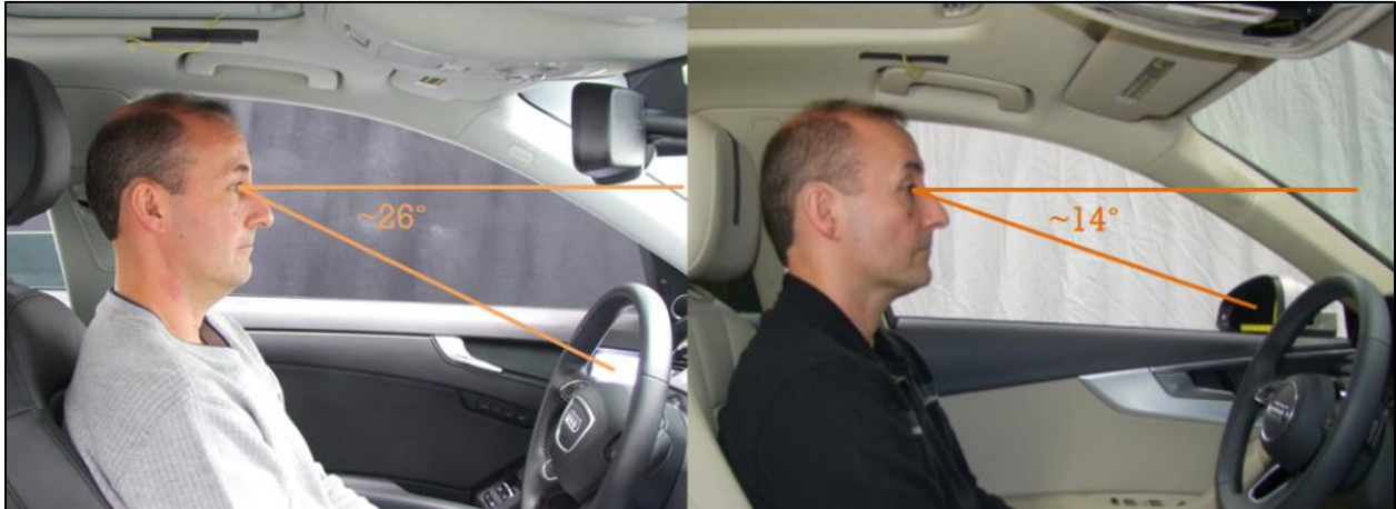
Figure 28. Downward Viewing Angle, CMS Display Versus Mirror
