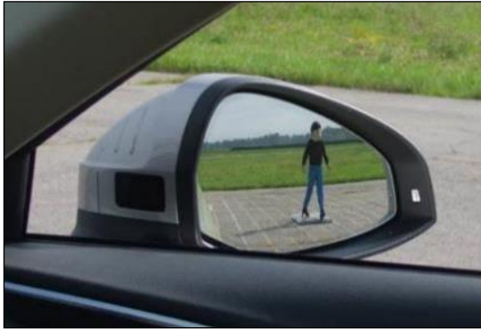
Figure 51. Child Mannequin Positioned 16.4 Feet (5 m) Aft of Rear Bumper, as Viewed With Side CMS (top) and Mirrors (bottom) on Driver (left) and Passenger Side (right)
