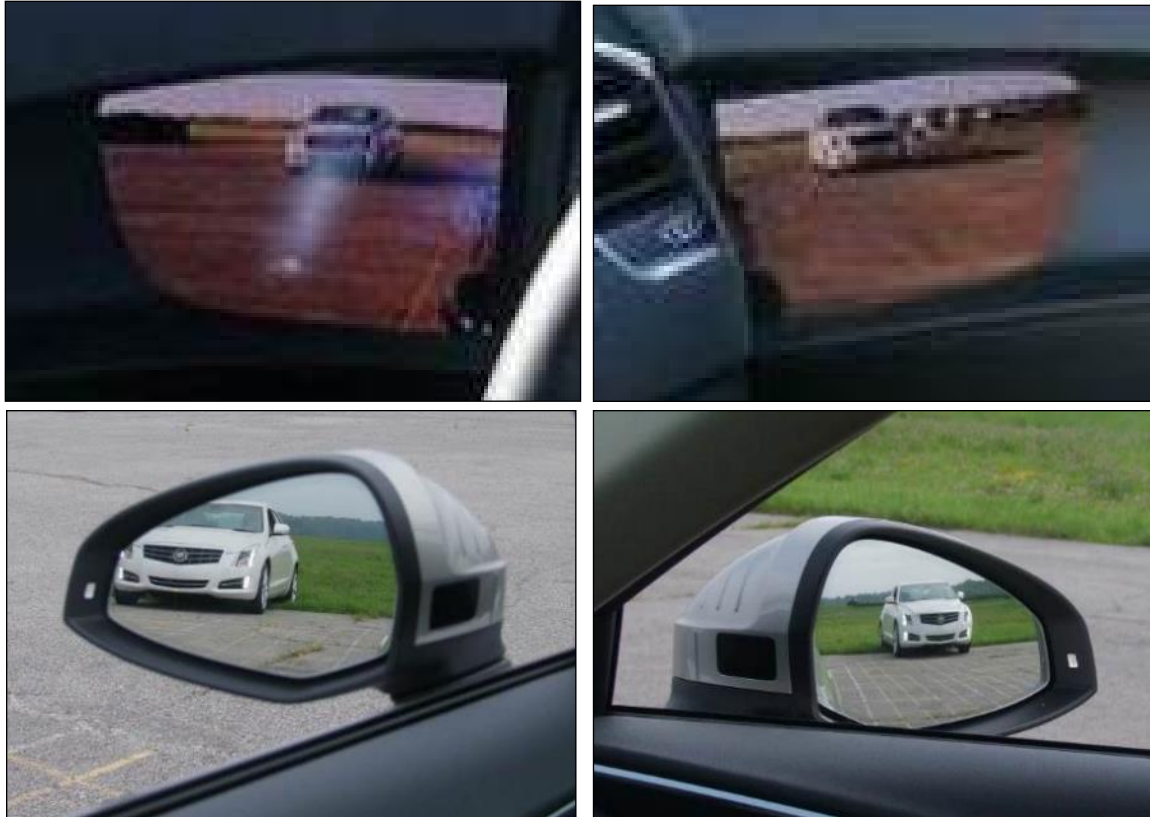
Figure 48. Sedan Positioned 32.8 Feet (10 m) Aft of Rear Bumper, as Viewed With Side CMS (top) and Mirrors (bottom) on Driver (left) and Passenger Side (right)
