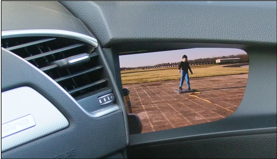
Figure 21. Posable Child Mannequin in Sunny Test Conditions, Minimal Glare/Reflection in CMS Display
