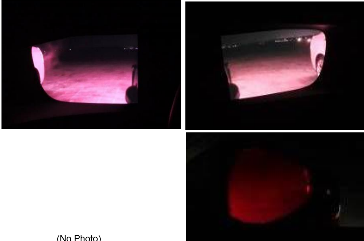
Figure 54. Sedan Positioned 5 Feet (1.52 m) Aft of Front Bumper at Night Time, as Viewed With Side CMS (left) and Mirrors (right) on Passenger Side
