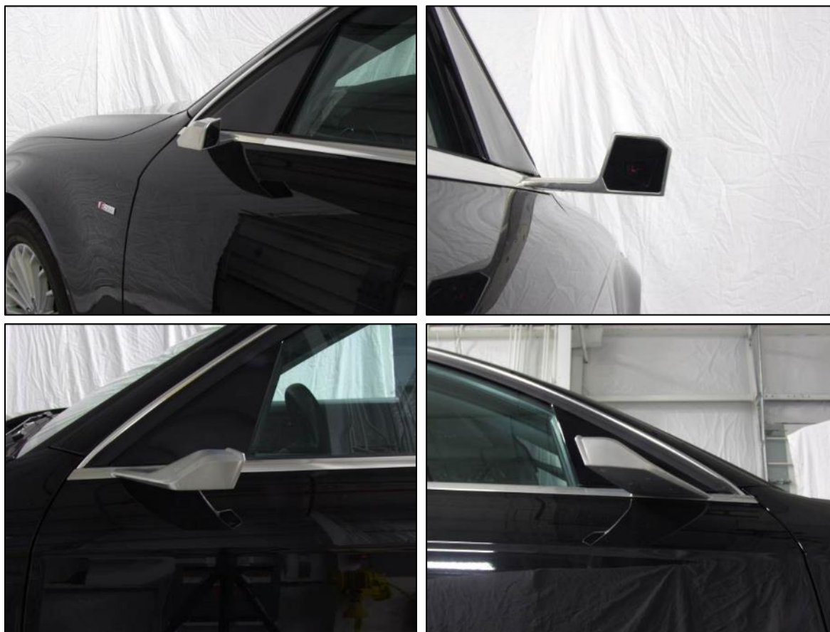
Figure 1. Photos Showing Cameras of the Prototype Side Camera Monitor System
