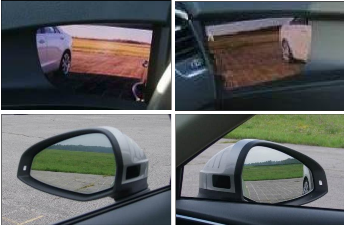
Figure 44. Sedan Positioned 10 Feet (3.05 m) Aft of Front Bumper, as Viewed With Side CMS (top) and Mirrors (bottom) on Driver (left) and Passenger Side (right)
