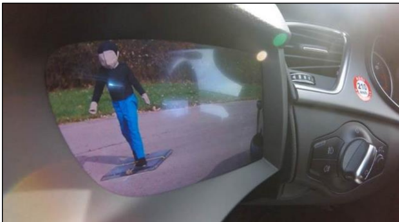
Figure 19. Posable Child Mannequin in Sunny Test Conditions, Glare/Reflection in CMS Display
