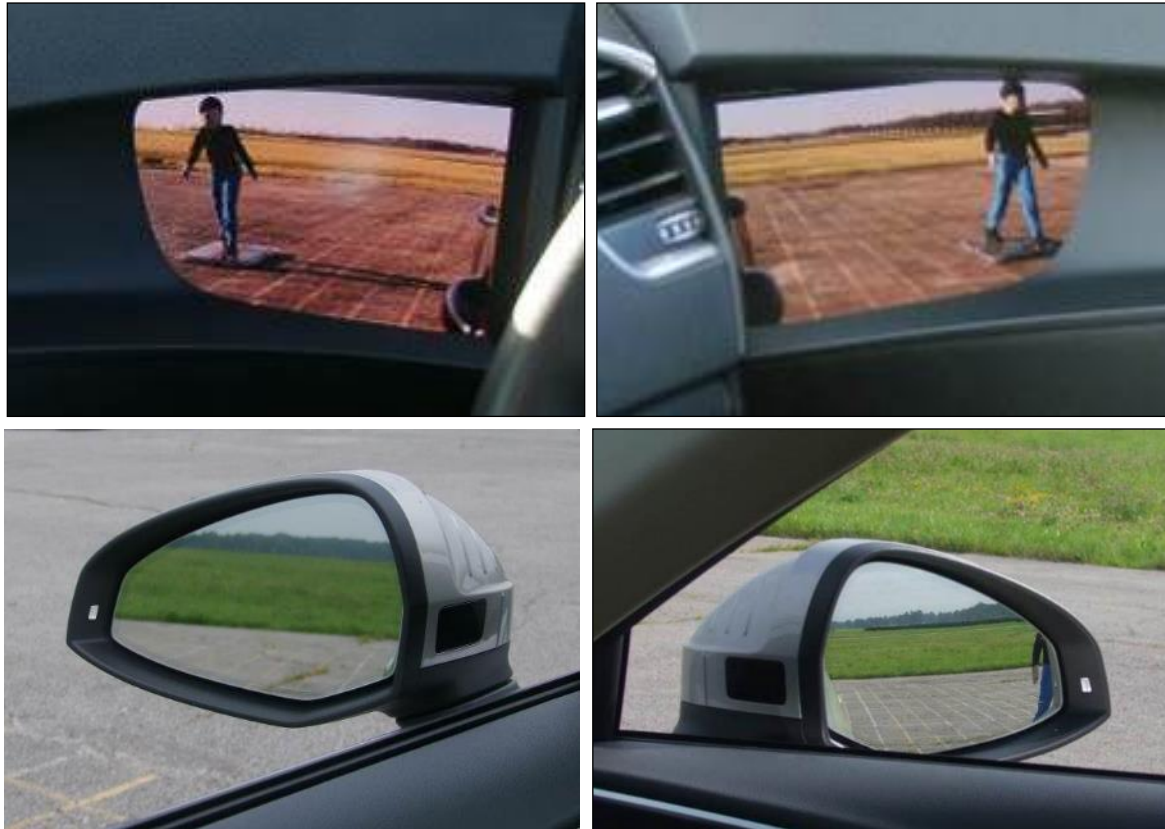
Figure 50. Child Mannequin Positioned 5 Feet (1.52 m) Aft of Rear Bumper, as Viewed With Side CMS (left) and Mirrors (right) on Passenger Side
