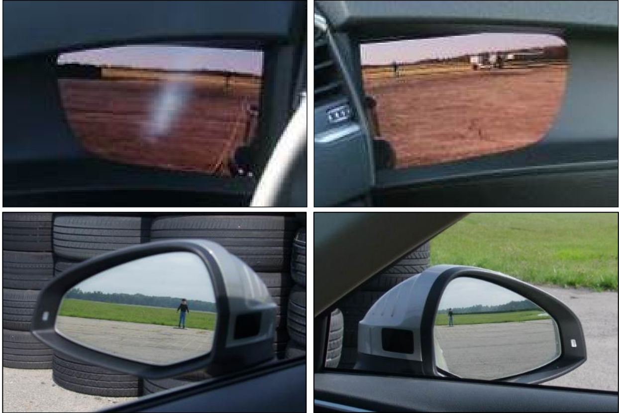
Figure 16. Child Mannequin Positioned 82.0 Feet (25 m) Aft of Rear Bumper, as Viewed With Side CMS (top) and Mirrors (bottom) on Driver (left) and Passenger Side (right)
