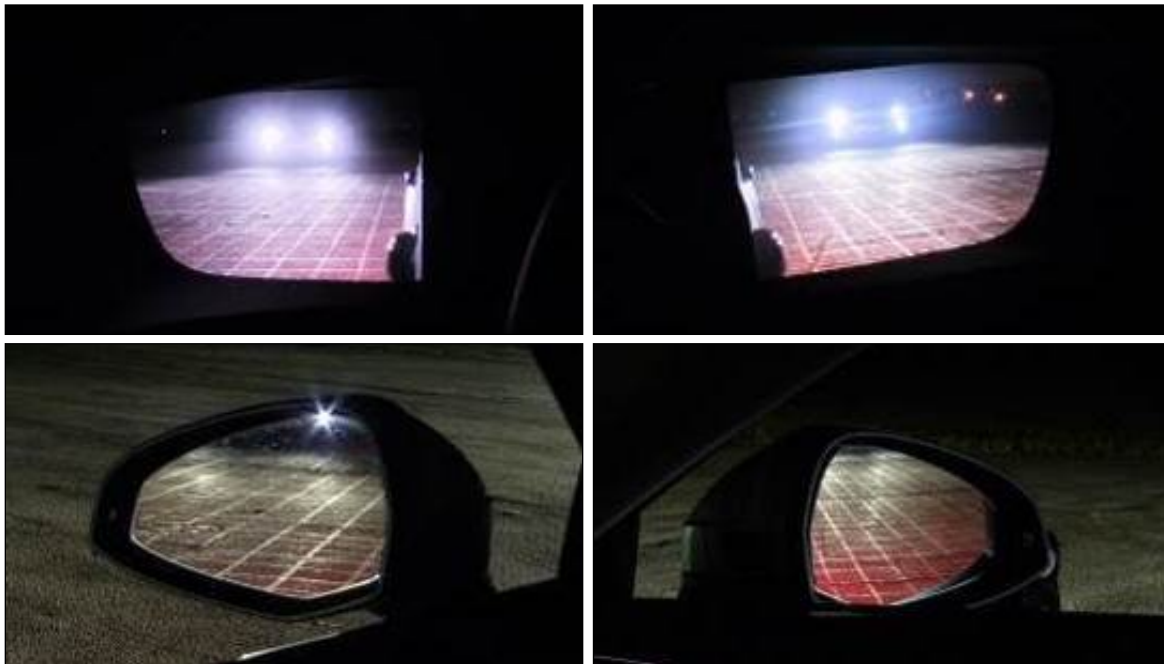
Figure 59. Sedan Positioned 32.8 Feet (10 m) Aft of Rear Bumper at Night Time, as Viewed With Side CMS (top) and Mirrors (bottom) on Driver (left) and Passenger Side (right)
