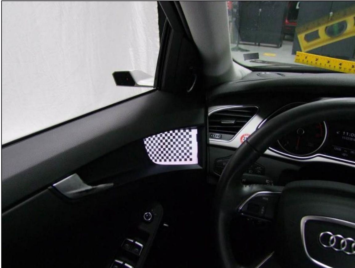
Figure 6. Driver-Side Interior Display, Driver's Viewpoint, ISO Grid in View
