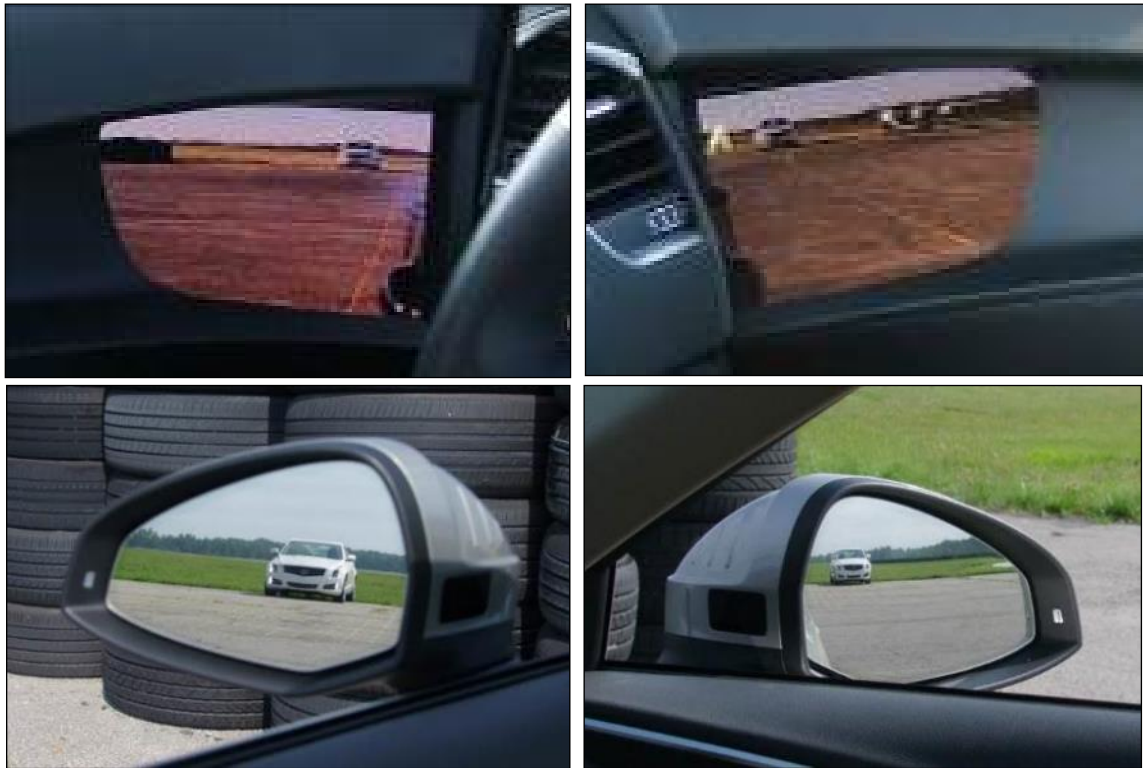
Figure 49. Sedan Positioned 82.0 Feet (25 m) Aft of Rear Bumper, as Viewed With Side CMS (top) and Mirrors (bottom) on Driver (left) and Passenger Side (right)
