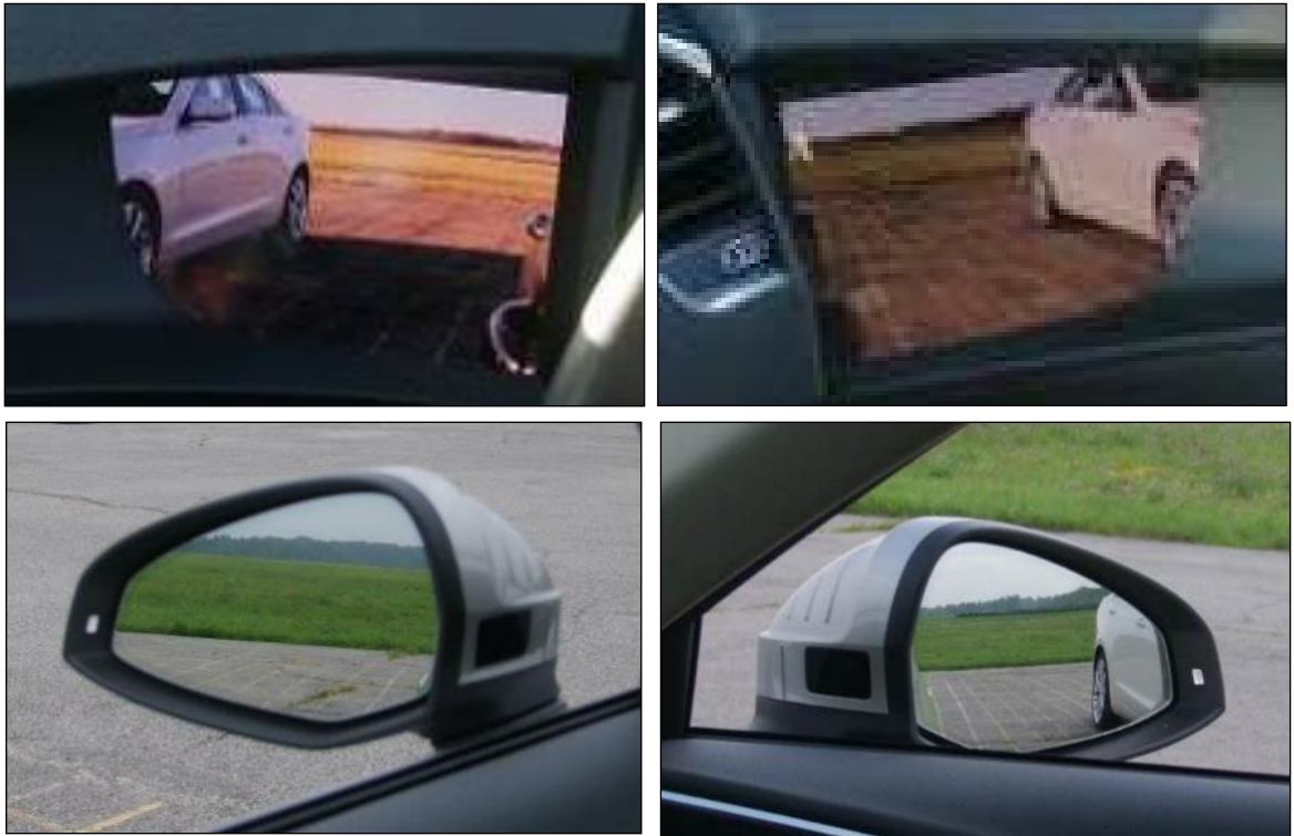
Figure 45. Sedan Positioned 15 Feet (4.57 m) Aft of Front Bumper, as Viewed With Side CMS (top) and Mirrors (bottom) on Driver (left) and Passenger Side (right)
