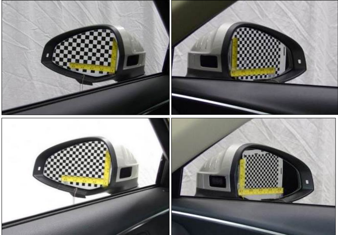
Figure 26. Near and Far Chessboard in Lighted Environment as Viewed With Driver (left) and Passenger Side (right) Mirrors
