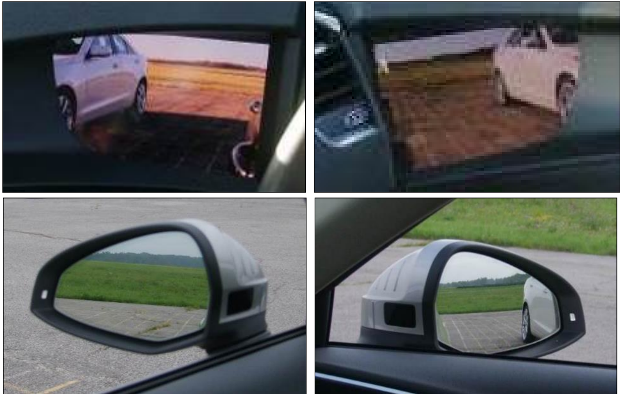
Figure 15. Sedan Positioned 15 Feet (4.57 m) Aft of Front Bumper, as Viewed With Side CMS (top) and Mirrors (bottom) on Driver (left) and Passenger Side (right)
