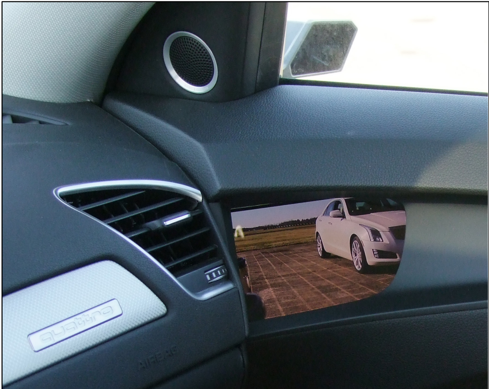
Figure 22. Sedan Test Object in Sunny Test Conditions, Minimal Glare/Reflection in CMS Display
