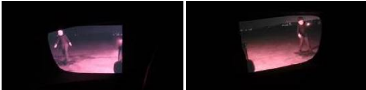
Figure 61. Child Mannequin Positioned 5 Feet (1.52 m) Aft of Rear Bumper, at Night Time as Viewed With Side CMS on Driver (left) and Passenger Side (right)
