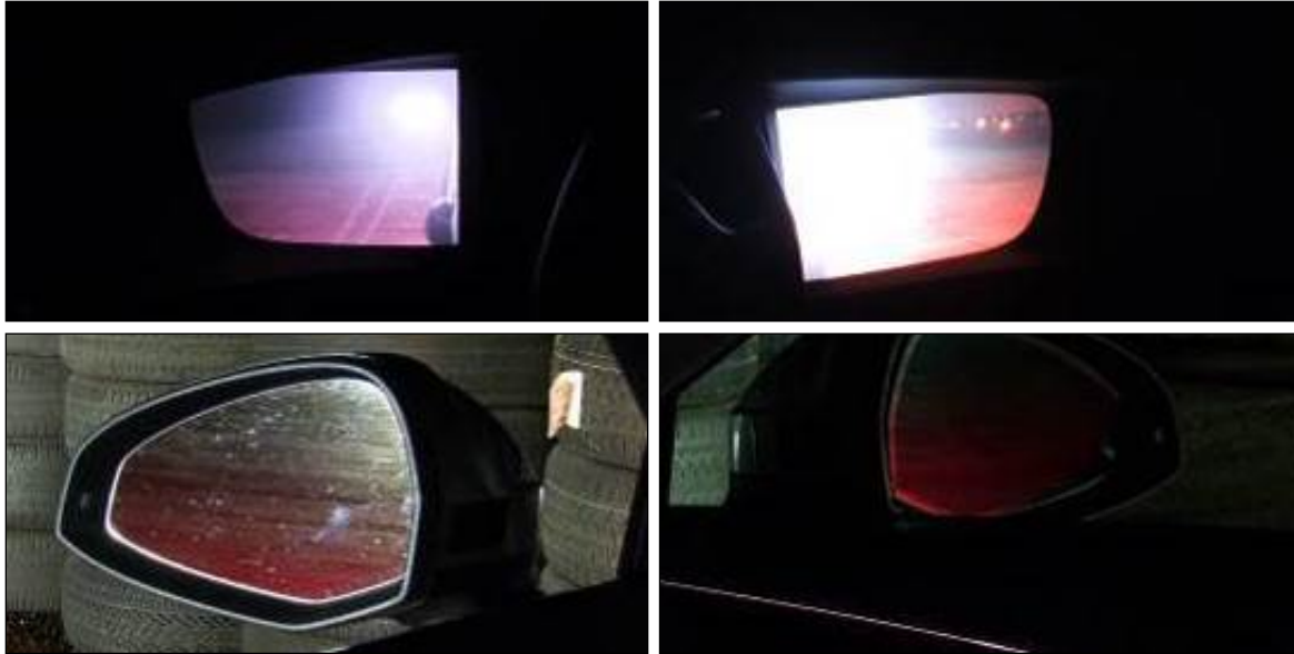
Figure 60. Sedan Positioned 82.0 Feet (25 m) Aft of Rear Bumper at Night Time, as Viewed With Side CMS (top) and Mirrors (bottom) on Driver (left) and Passenger Side (right)
