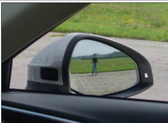
Figure 52. Child Mannequin Positioned 32.8 Feet (10 m) Aft of Rear Bumper, as Viewed With Side CMS (top) and Mirrors (bottom) on Driver (left) and Passenger Side (right)
