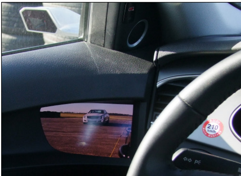
Figure 20. Sedan Test Object in Sunny Test Conditions, Glare/Reflection in CMS Display
