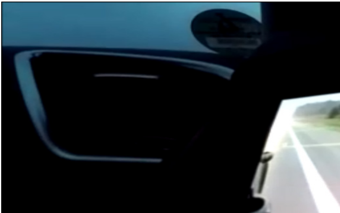
Figure 31. Photo of Passenger-Side CMS Display and Portion of Forward Windshield View, Highlighting the Disparity in Apparent Ambient Illumination at Dusk
