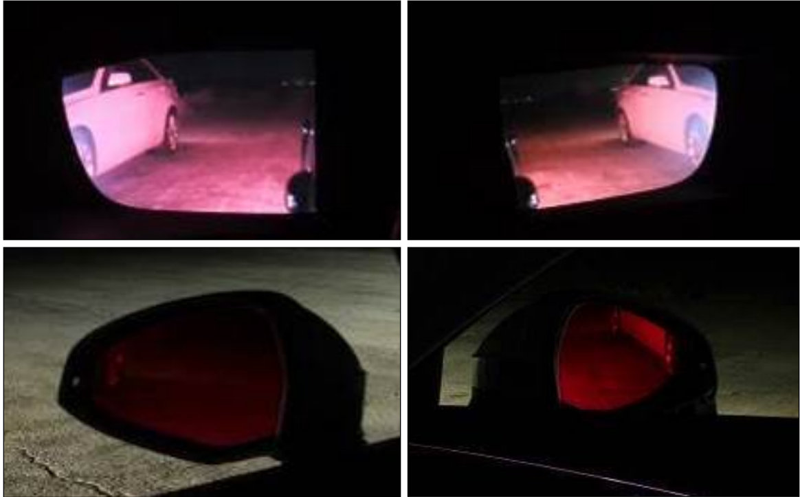
Figure 56. Sedan Positioned 15 Feet (4.57 m) Aft of Front Bumper at Night Time, as Viewed With Side CMS (top) and Mirrors (bottom) on Driver (left) and Passenger Side (right)
