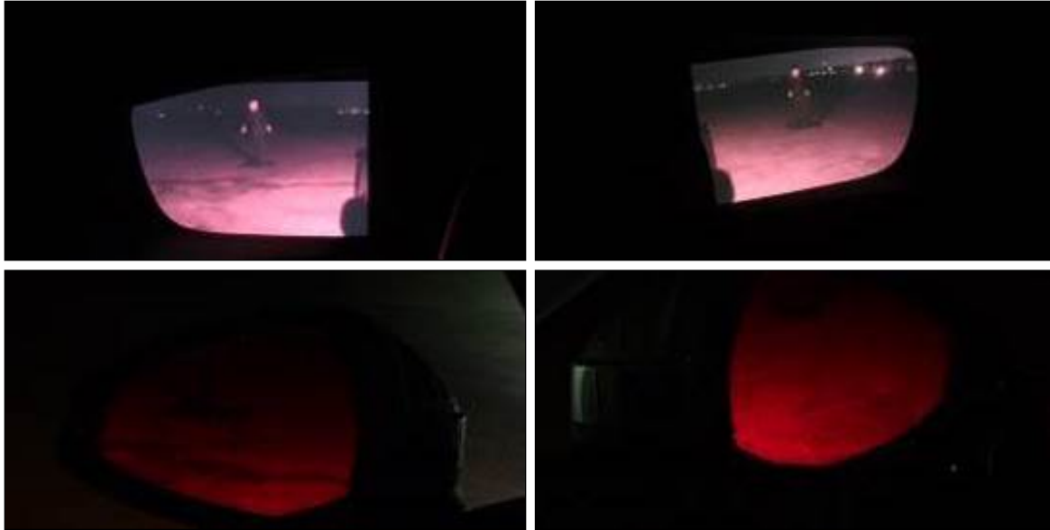
Figure 62. Child Mannequin Positioned 16.4 Feet (5 m) Aft of Rear Bumper, at Night Time as Viewed With Side CMS (top) and Mirrors (bottom) on Driver (left) and Passenger Side (right)
