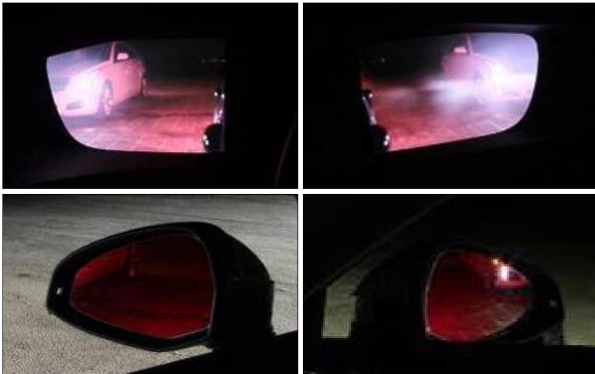
Figure 57. Sedan Positioned 5 Feet (1.52 m) Aft of Rear Bumper at Night Time, as Viewed With Side CMS (top) and Mirrors (bottom) on Driver (left) and Passenger Side (right)
