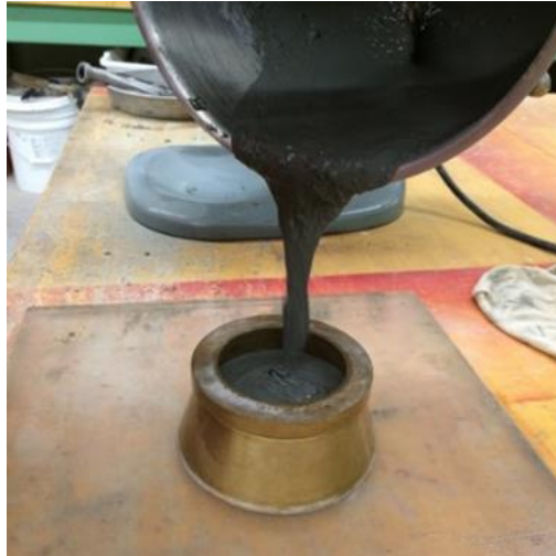
Figure 6. Filling of mold with rapid repair mixture
