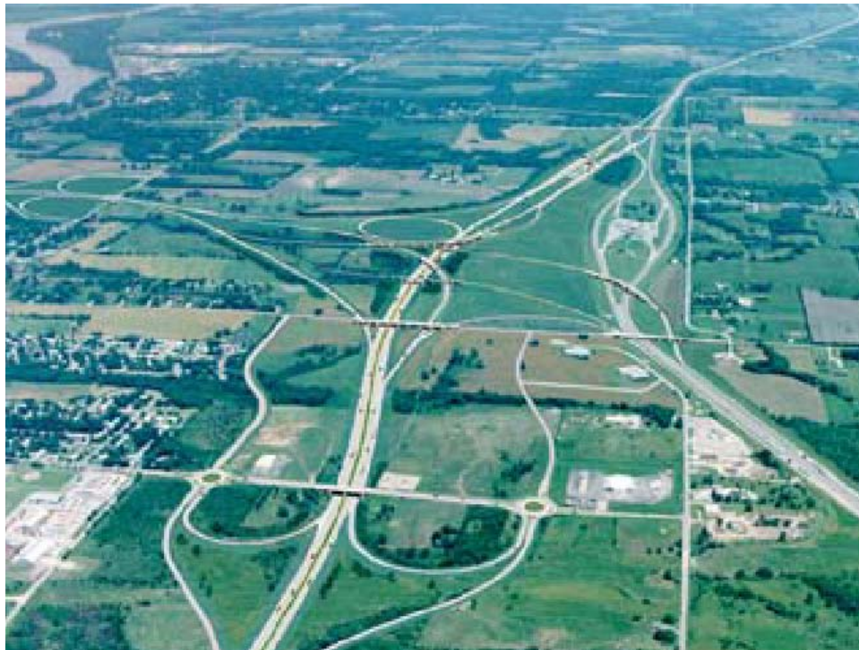
FIGURE 6.38: Aerial View of the Realigned Interstate 70 (I-70) and Rice Road Intersection Roundabouts (Source KDOT)
