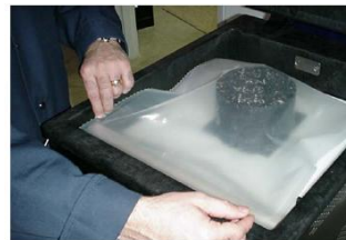
Placing plastic inside sealing chamber
