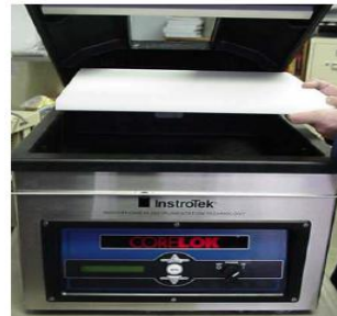
Placing filler plate
