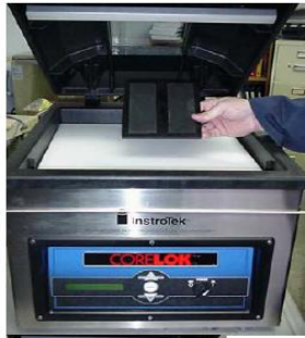
Placing sliding plate
