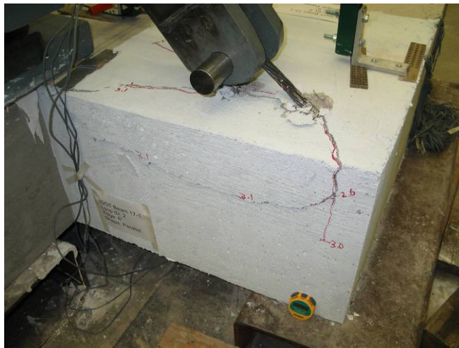
Figure 2: Triangle Wedge Cracking (Stage 2)
