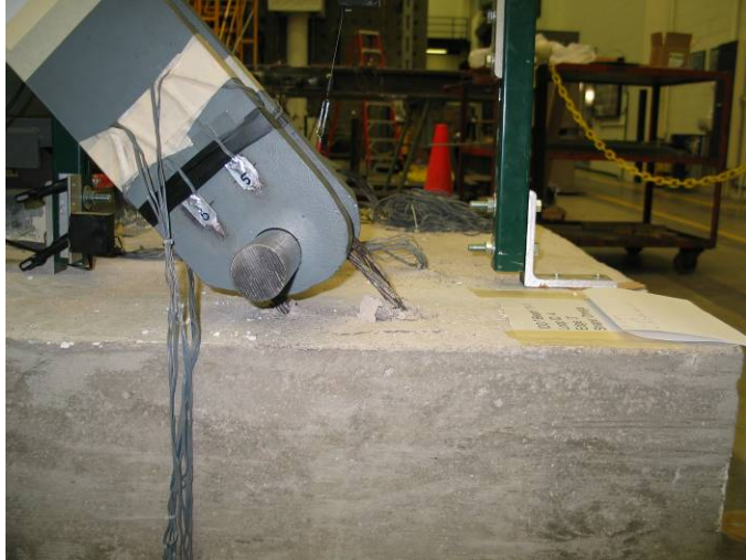
Figure 1: First Cracking (Stage 1)
