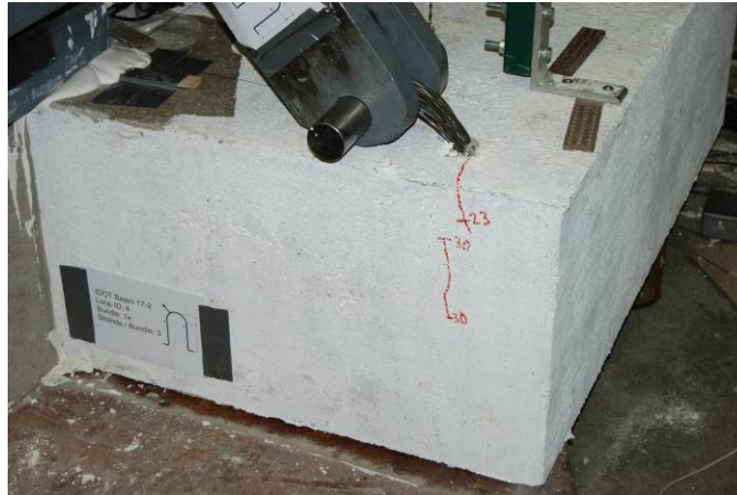
Figure 1: First Cracking (Stage 1)
