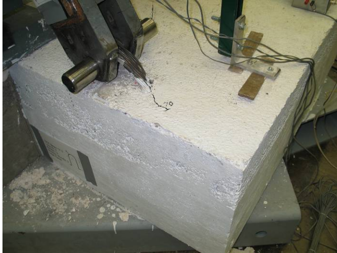
Figure 1: First Cracking (Stage 1)
