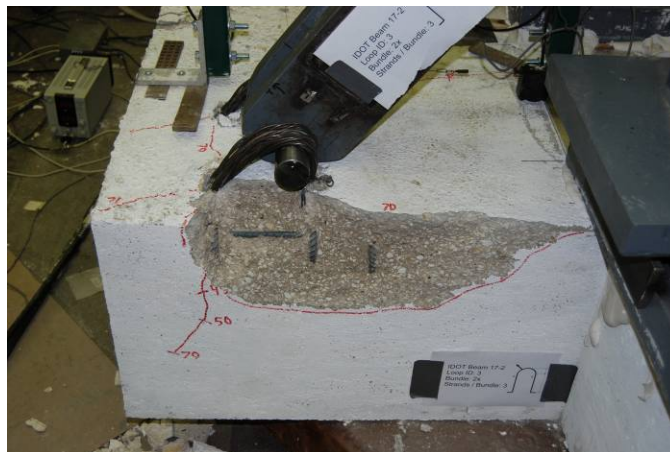
Figure 2: Triangle Wedge Cracking (Stage 2)
