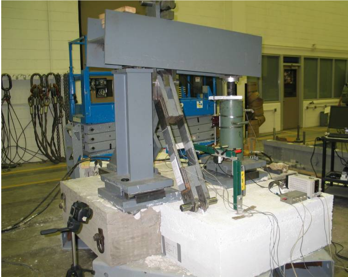
Figure 15. Deck beam testing apparatus.
