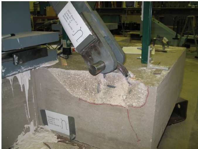
Figure 2: Triangle Wedge Cracking (Stage 2)
