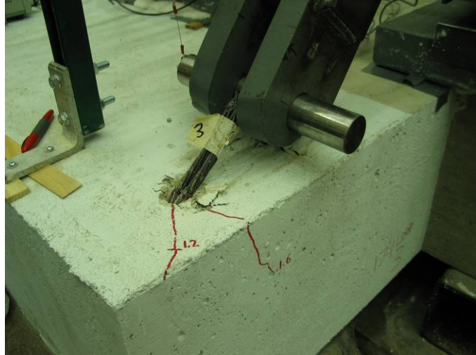
Figure 1: First Cracking (Stage 1)
