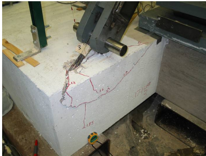
Figure 2: Triangle Wedge Cracking (Stage 2)
