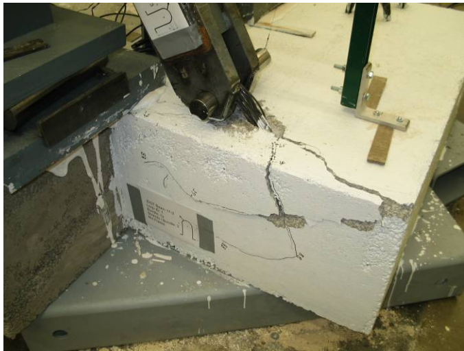
Figure 2: Triangle Wedge Cracking (Stage 2)
