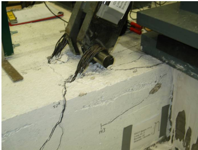
Figure 2: Triangle Wedge Cracking (Stage 2)
