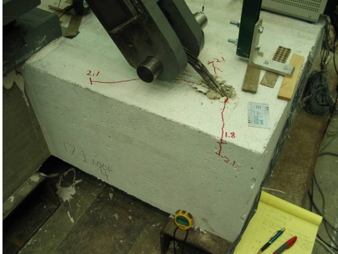
Figure 1: First Cracking (Stage 1)
