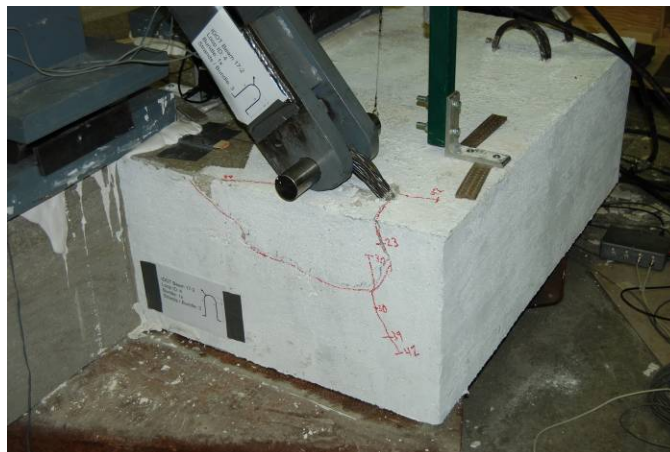
Figure 2: Triangle Wedge Cracking (Stage 2)
