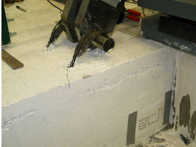
Figure 1: First Cracking (Stage 1)
