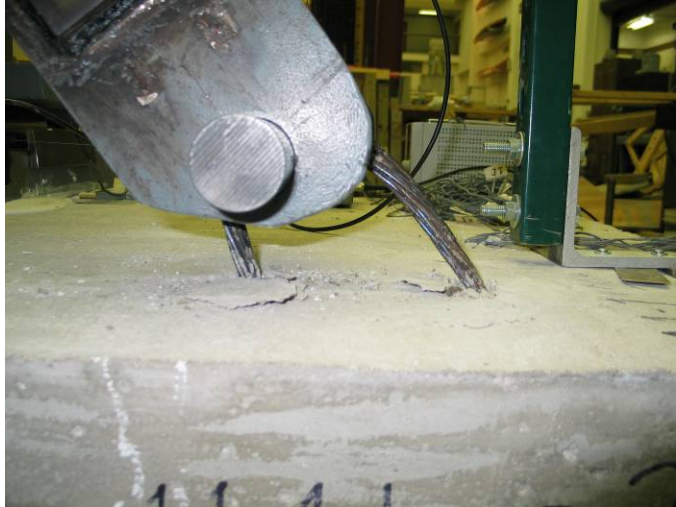
Figure 1: First Cracking (Stage 1)
