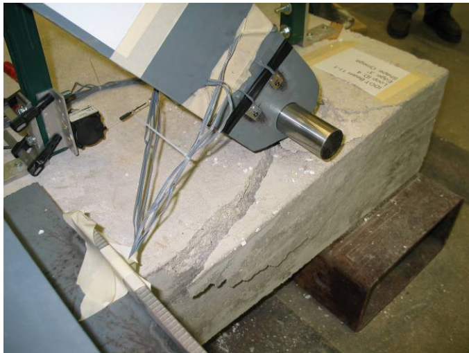
Figure 2: Triangle Wedge Cracking (Stage 2)
