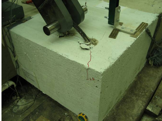
Figure 1: First Cracking (Stage 1)
