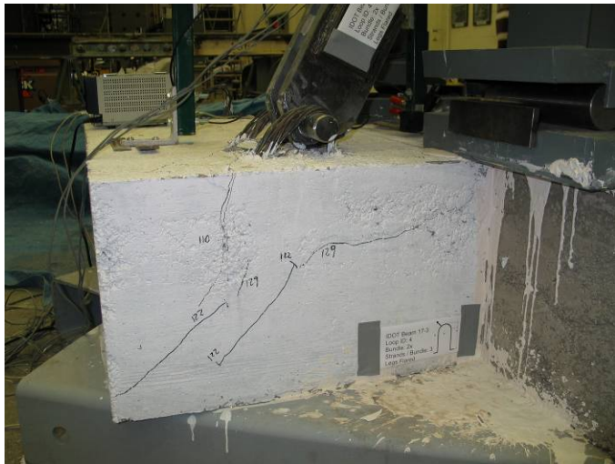
Figure 2: Triangle Wedge Cracking (Stage 2)
