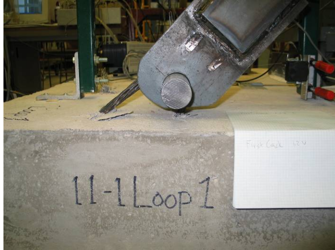
Figure 1: First Cracking (Stage 1)
