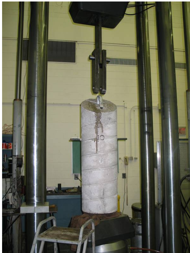
Figure 16. Strand rupture test setup.
