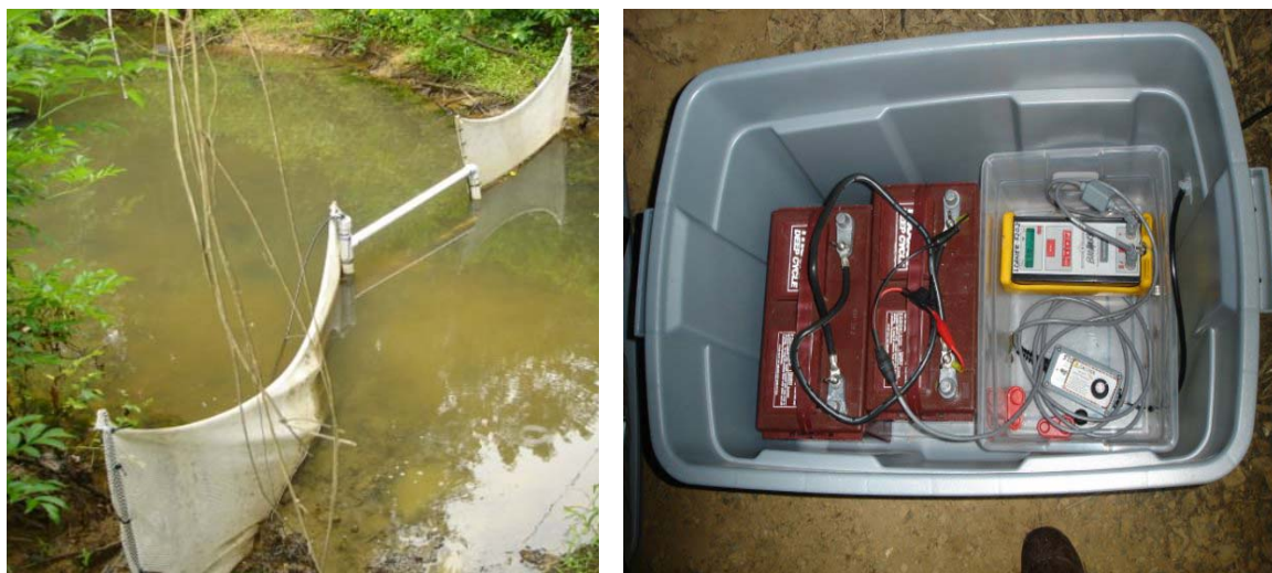
Figure 4.2: Remote antenna array complete with net weirs, shielded cable, FS2001 reader, tuning box, and batteries in place downstream of the box culvert in Mary's Creek (Photographs by Jenny Vander Pluym).
