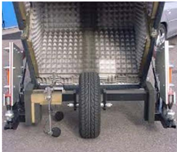
Figure 4.4: CPX Microphone Placement and Trailer Interior
