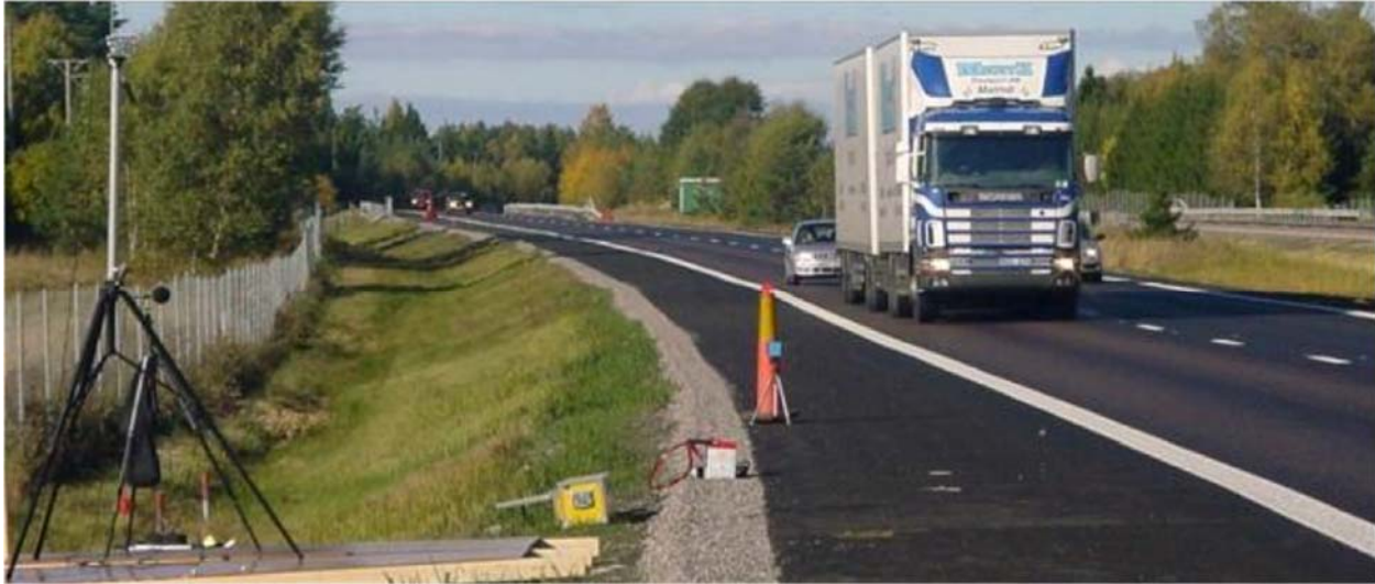
Figure 4.7: SPB Roadside Setup
