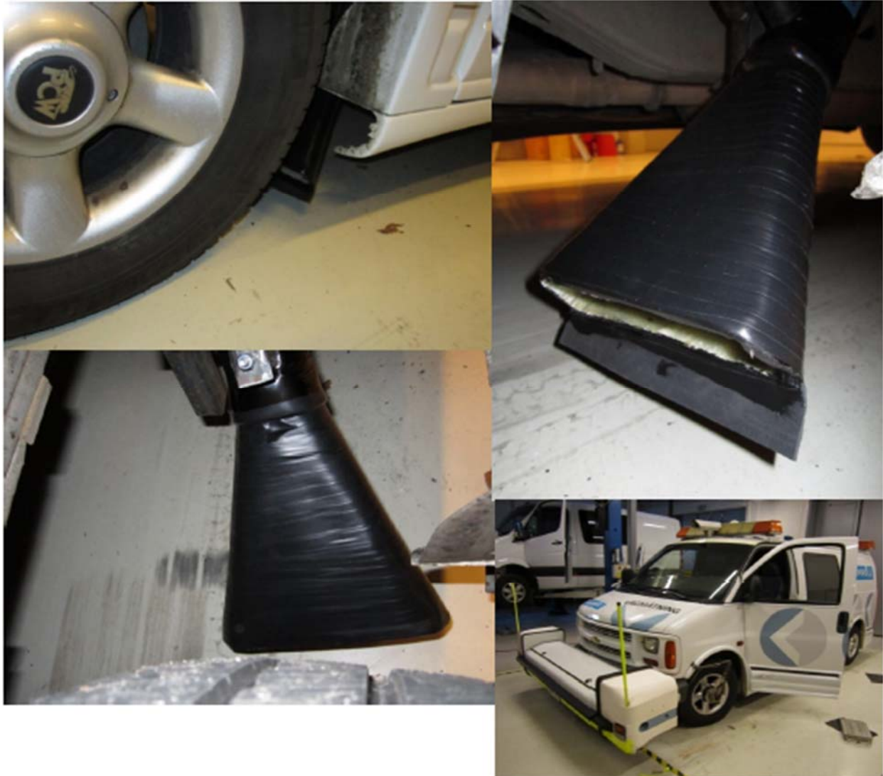
Figure 4.6: Clockwise from top-left: CPX Tube Mounted on Vehicle; Close-Up of CPX Tube; Test Vehicle; Second Angle of Mounted CPX Tube
