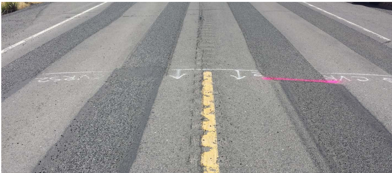
Figure 30. Formula 2 chip seal in the foreground, with conventional chip seal in the background. Note the loss of aggregate at the edges of the wheel paths on the Formula 2 test section.
