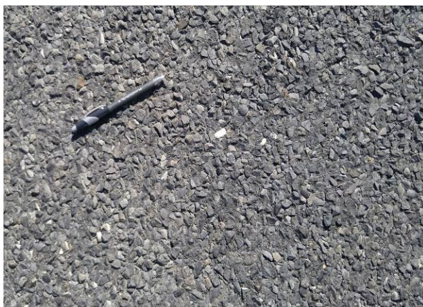
Figure 51. Choke filling areas between chips. Formula 3 test section after 1 month.
