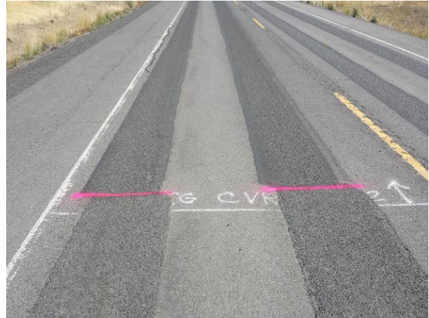
Figure 29. Break line between Formula 1 CVRS-2P and CRS-2P binders. CVRS-2P in the background, CRS-2P in the foreground.
