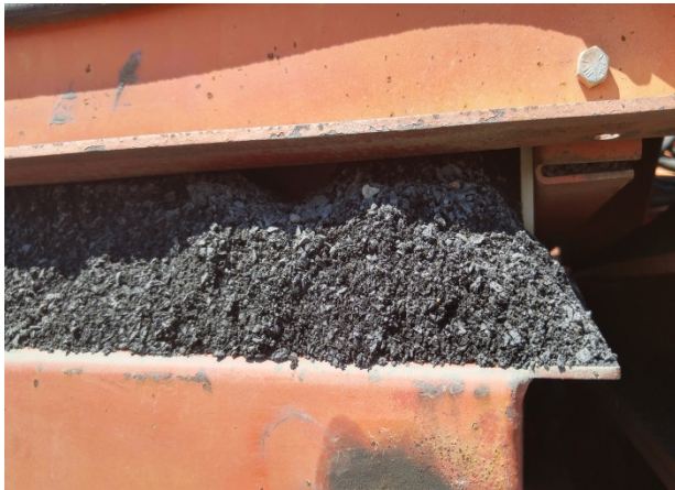
Figure 65. Choke stone in the chip spreader.
