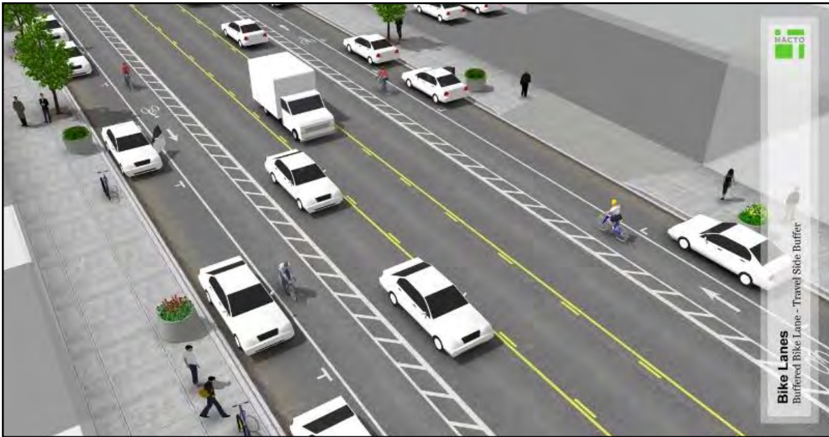
Figure 2. Buffered Bike Lane: A Standard 8-Foot Bike Lane with 3-Foot Buffers on a Minor Roadway (Collector Street)
