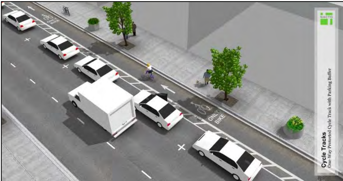
Figure 3. Buffered from Traffic by Parking: A Standard Bike Lane, with 3-Foot Buffers, on a Minor Roadway (Collector Street)
