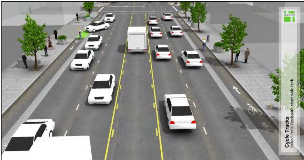
Figure 5. Physical Separation Involves a Raised Bike Lane with Mountable Curb Separation from Traffic
