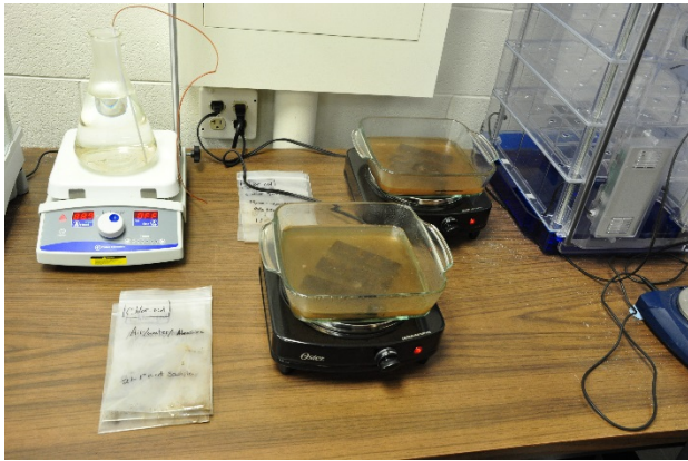
Figure 8. Boiling extraction to measure chloride of three panel segments.
