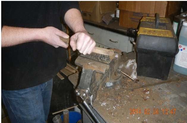
Figure 6. SSPC SP2 cleaning of panels with wire brush.
