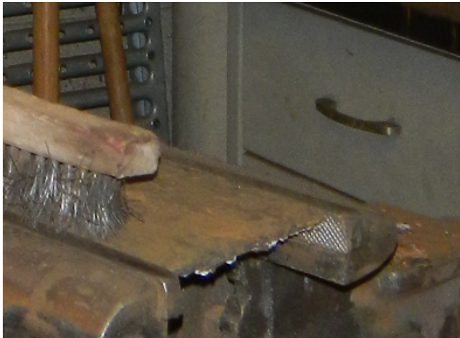
Figure 7. SSPC SP2 D condition prior to surface preparation.
