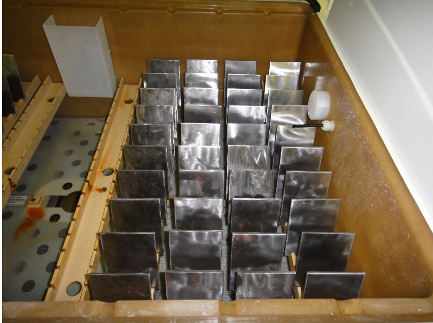
Figure 3. Steel panels with mill scale removed by grinding prior to preconditioning.
