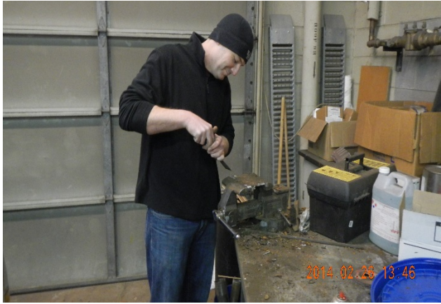
Figure 5. SSPC SP2 cleaning of panels with dull scraper.
