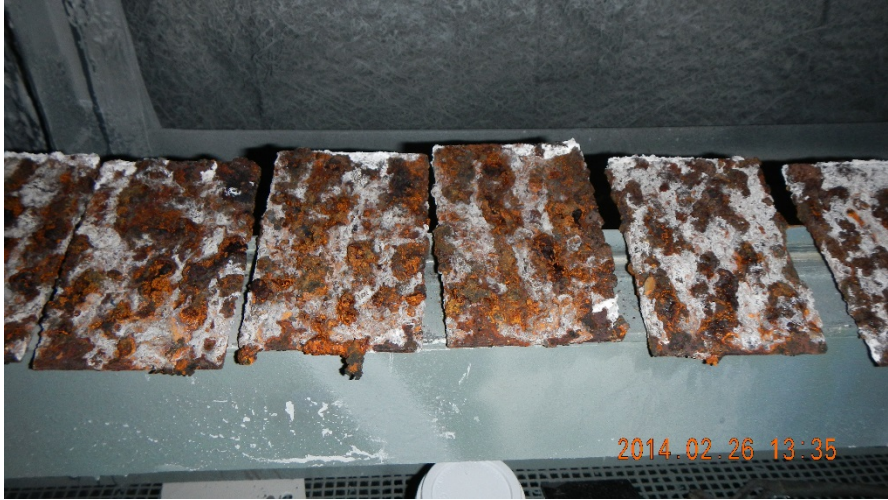
Figure 4. Panels with rust and chloride contamination after preconditioning.
