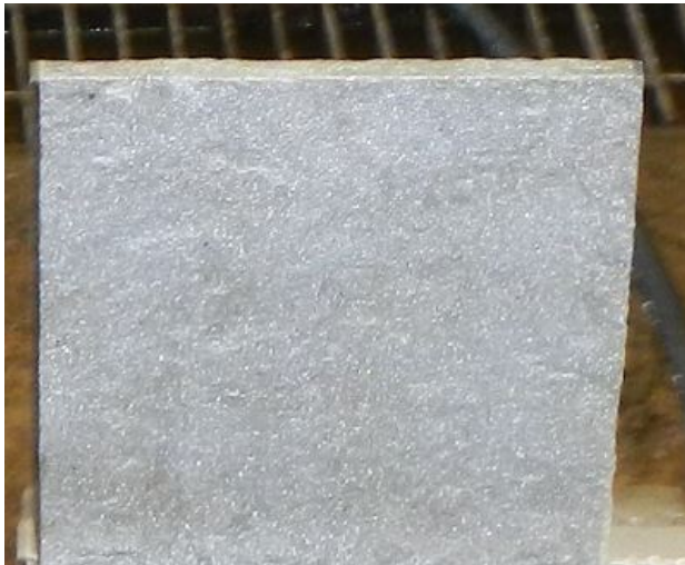
Figure 11. Cleanliness condition SSPC VIS4 WJ-1 after wet surface preparation methods.
