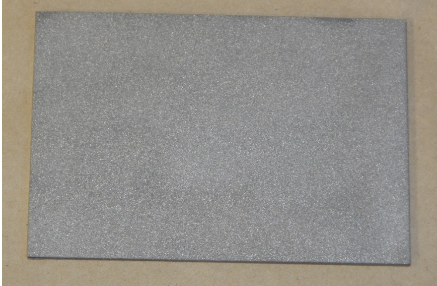
Figure 10. Cleanliness condition SSPC SP 10 after dry surface preparation methods.
