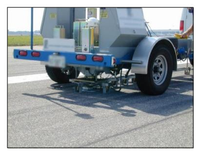
Figure 4. Photo. Impulse loading or FWD device.
