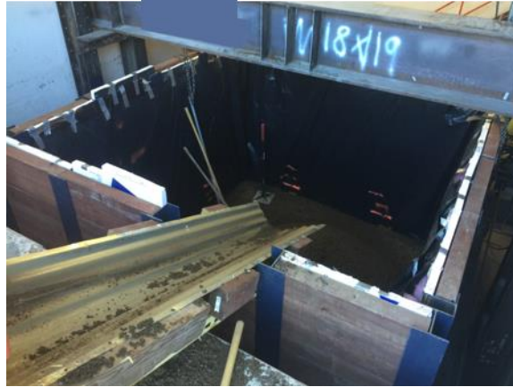
Figure 26. Photo. Placement of conditioned SG soil into the large-scale box via a material discharge chute in 4-inch lifts.
