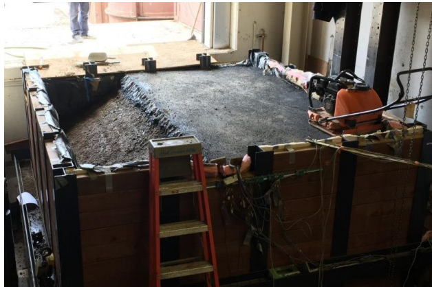
Figure 35. Photo. Slope construction in experiment No. 4: finished slope.
