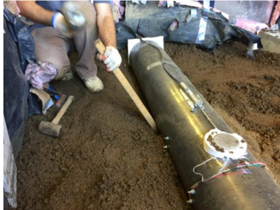
Figure 41. Photo. Manually compacting SG soil around the steel pipe.
