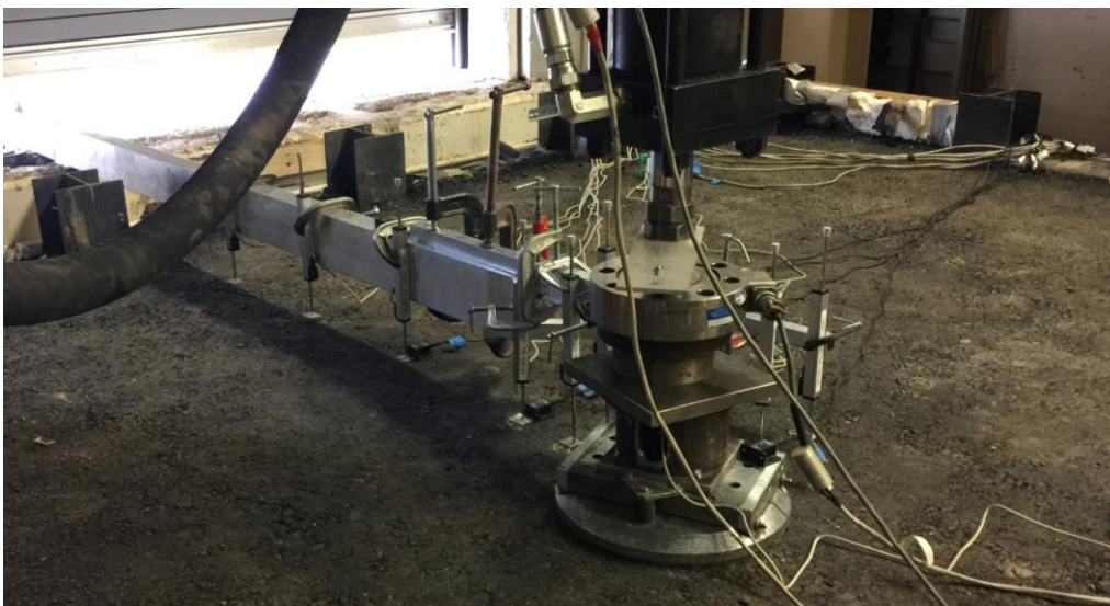
Figure 85. Photo. Completed large-scale-box test setup for experiment No. 5—loading location C (top of box culvert).
