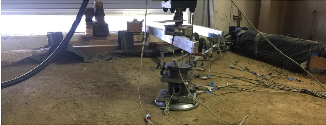
Figure 57. Photo. Completed large-scale-box test setup for experiment No. 2.
