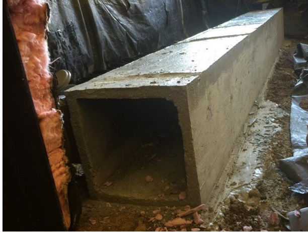
Figure 81. Photo. Cast-in-place monolithic rigid box culvert in the large-scale box.
