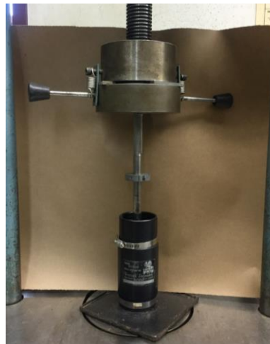
Figure 21. Photo. Static compaction of triaxial test specimen.
