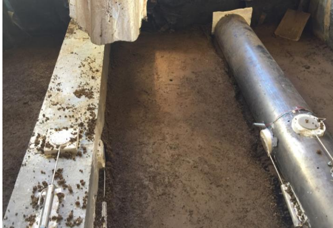
Figure 56. Photo. Buried flexible steel pipe and rigid concrete box culvert in experiment No. 5.
