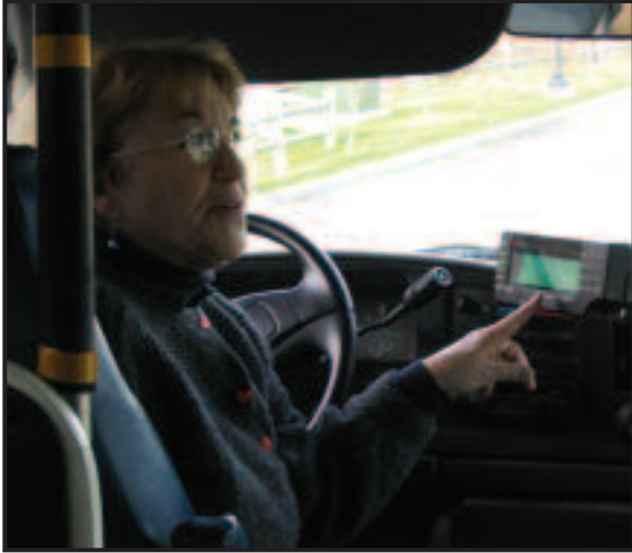
On-board communication equipment allows drivers to receive and react to scheduling changes more quickly
