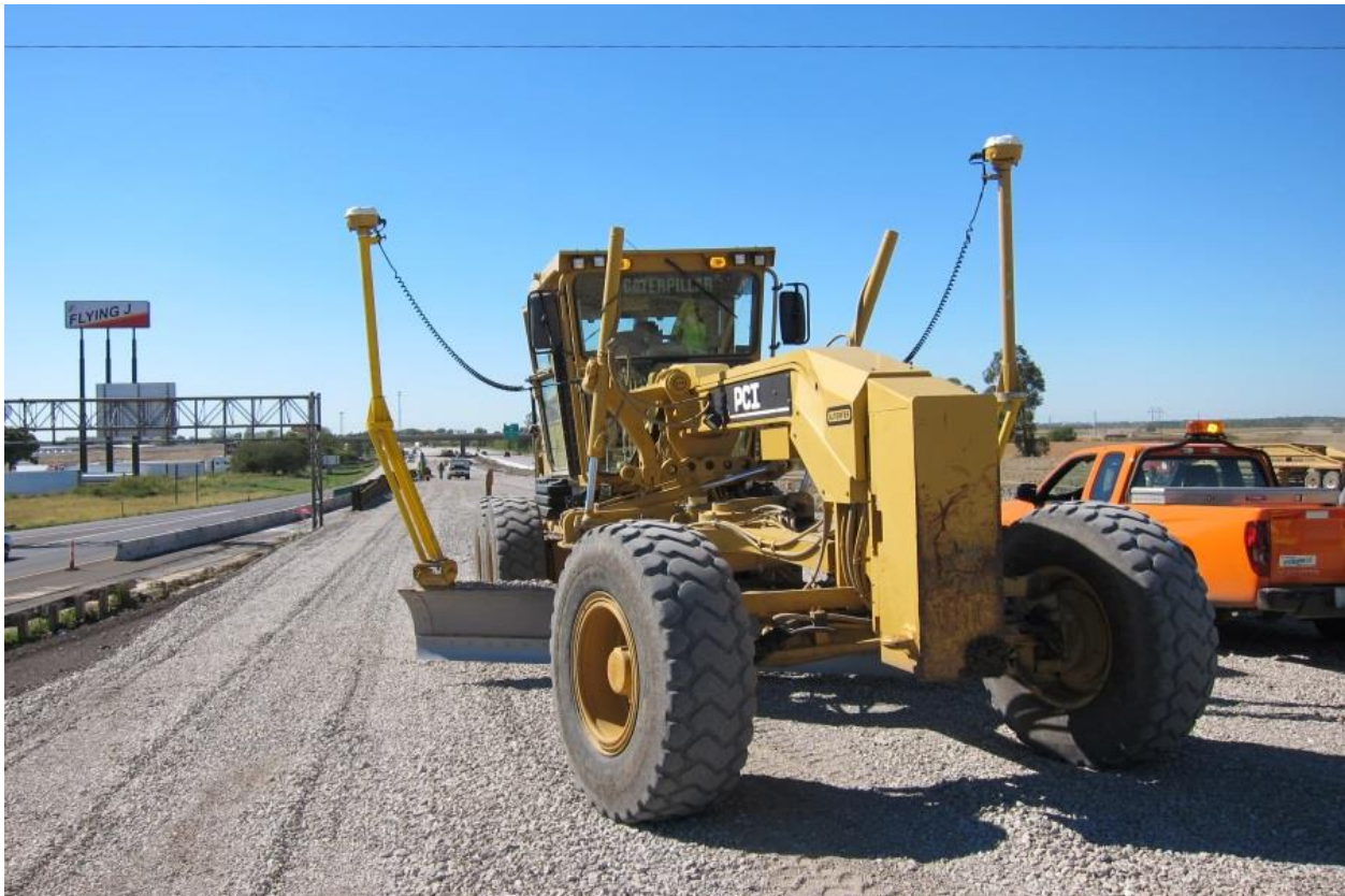
Figure 51. Photo. Construction equipment with AMG capabilities.
