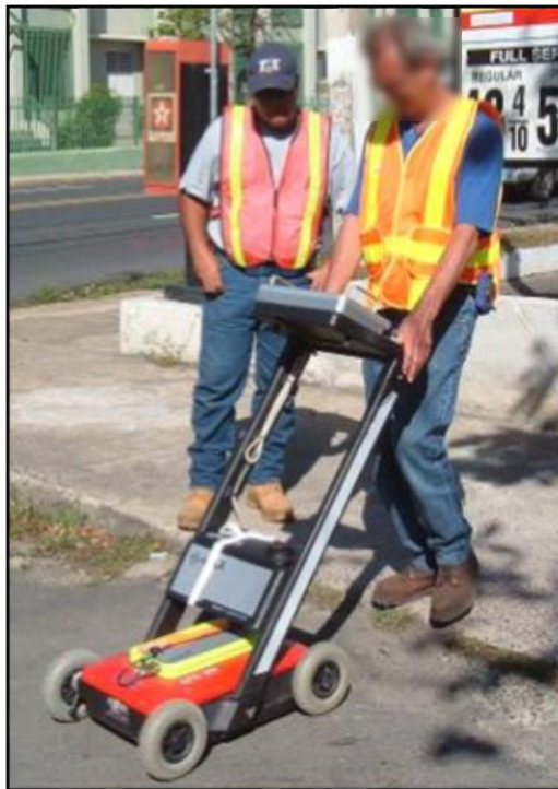
Figure 7. Photo. GPR equipment to detect underground facilities.
