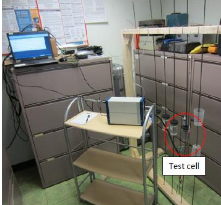
Figure 4. Photo. Multiple unstressed single-wire specimens and test cells. (1)
