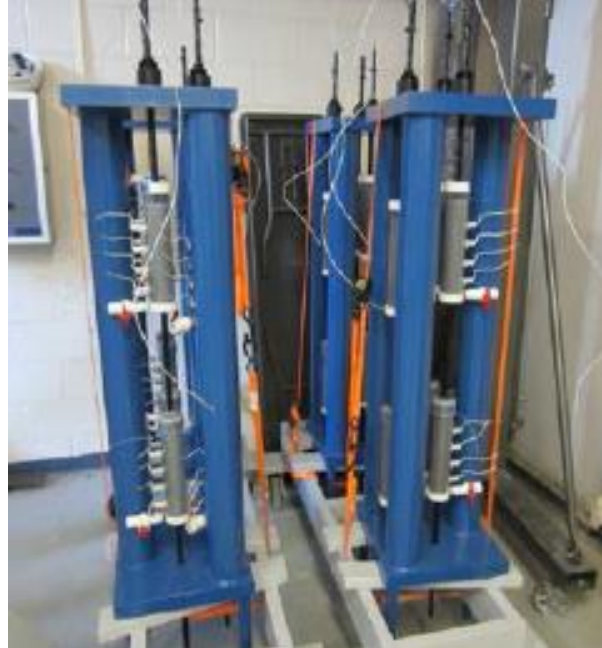
Figure 7. Photo. Grouted single-strand specimens in loading frames. (1)
