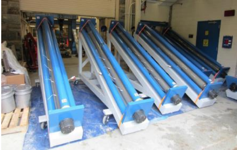
Figure 9. Photo. Multistrand specimens in loading frames under test. (1)
