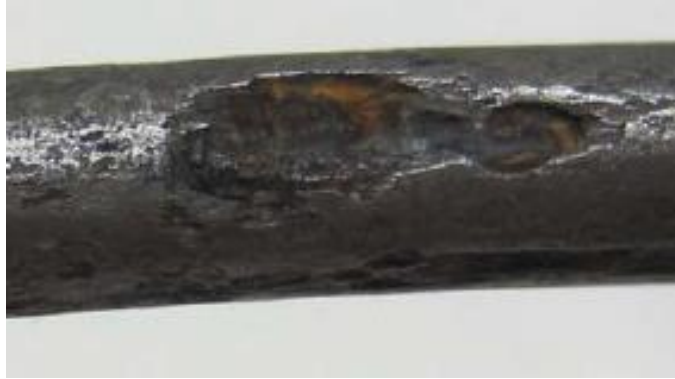
Figure 20. Photo. Example of a more advanced attack on a wire from a single-strand specimen with a grout void from the phase 1 study (figure 243) for which grout chloride concentration was 2.00 wt% (pit depth is 18 mils). (1)
