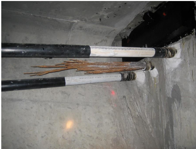
Figure 137. Photo. Photograph of a failed tendon on the Varina-Enon Bridge.
