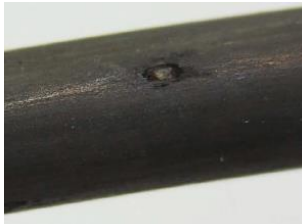
Figure 19. Photo. Example of initial localized corrosion on a wire from a fully grouted single-strand specimen of the phase 1 study (figure 239) for which grout chloride concentration was 0.80 wt% (pit depth is 4.7 mils). (1)
