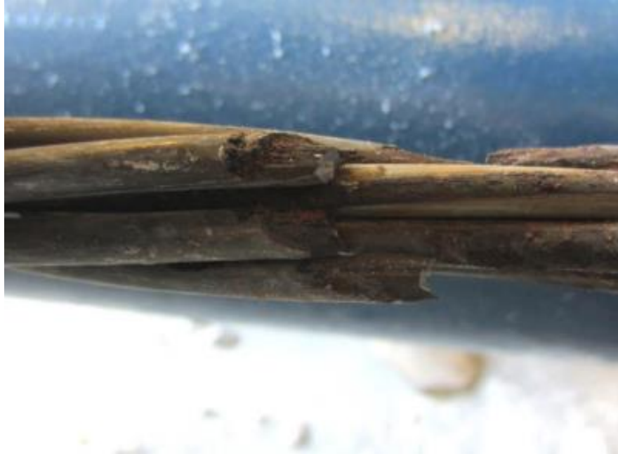
Figure 88. Photo. Closeup view of the strand in figure 87 showing fractured wires. (1)
