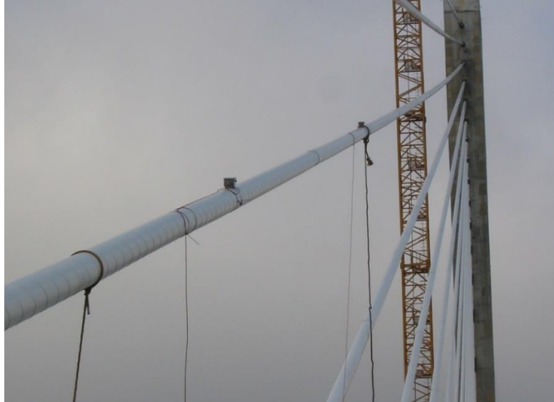
Figure 19. Photo. Accelerometers mounted on cable with pull rope attached.
