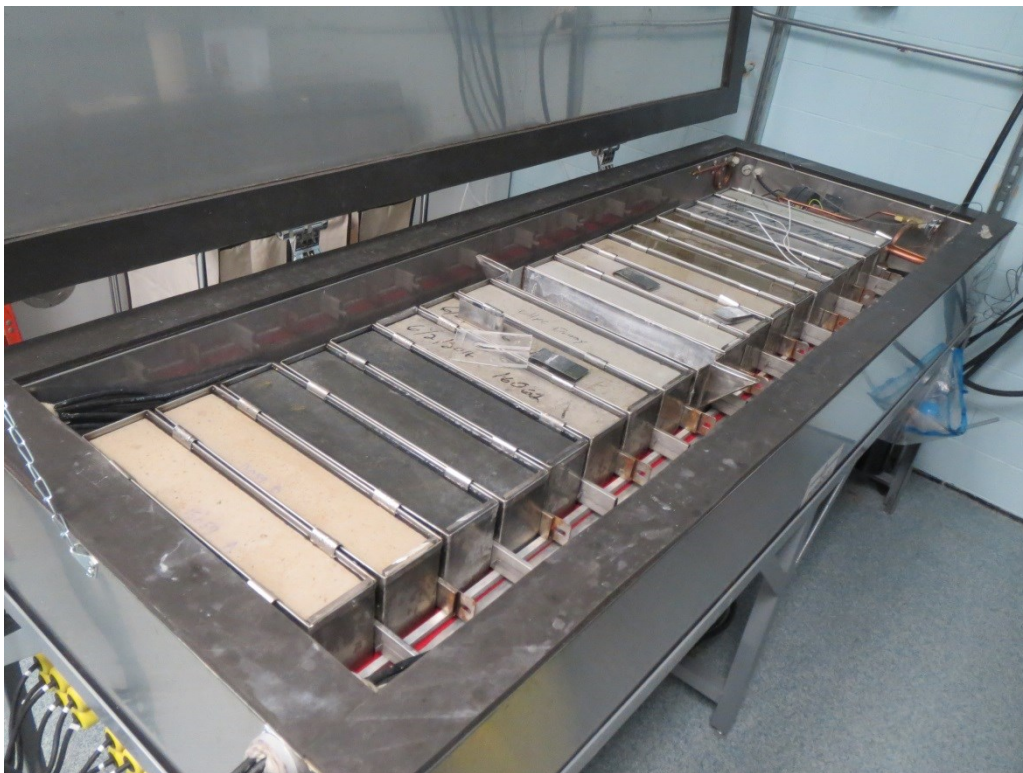
Figure 131. Photo. Environmental chamber for producing freeze-thaw cycles via ASTM C666 (Procedure A).
