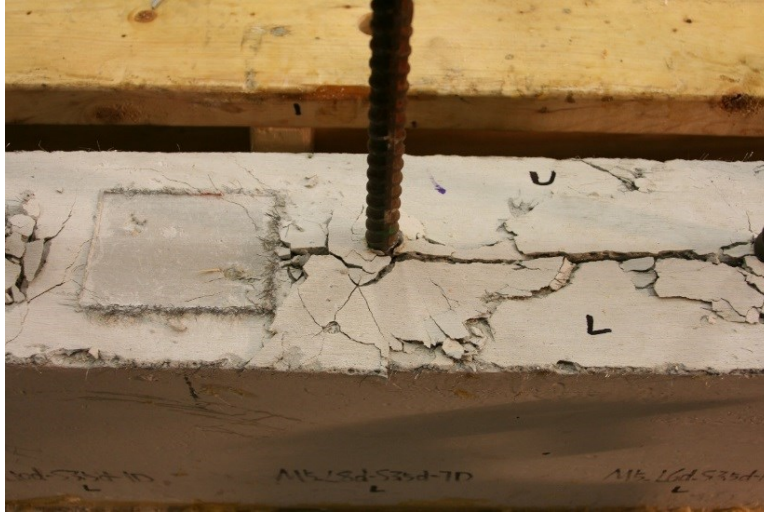
Figure 143. Photo. Bond test failure due to longitudinal splitting.
