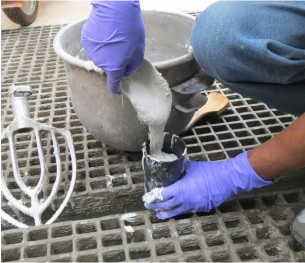
Figure 22. Photo. Placement of UHPC in a cylindrical specimen.
