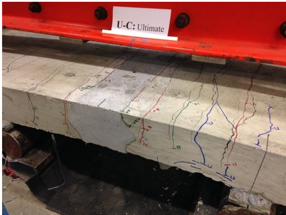
Figure 182. Photo. Specimen U-C after ultimate loading.
