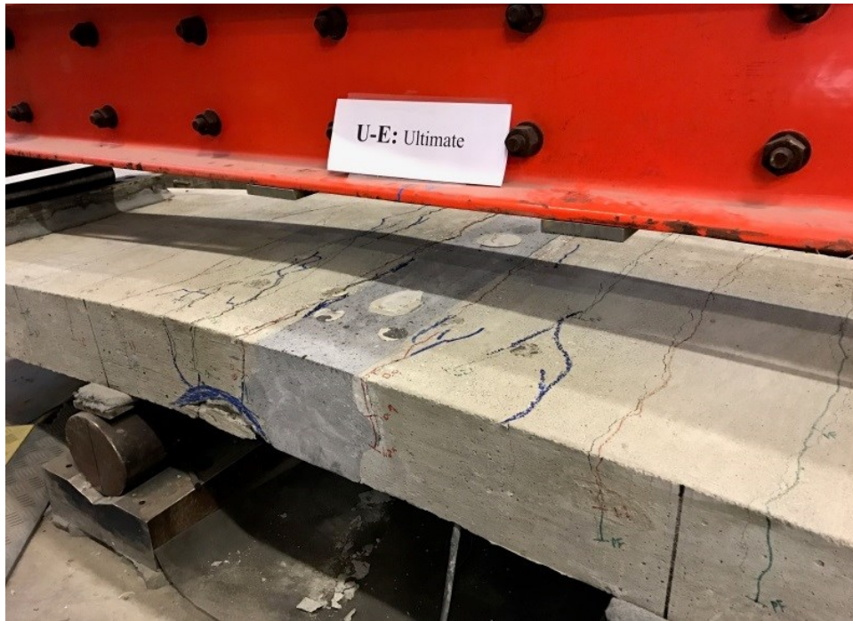
Figure 184. Photo. Specimen U-E after ultimate loading.
