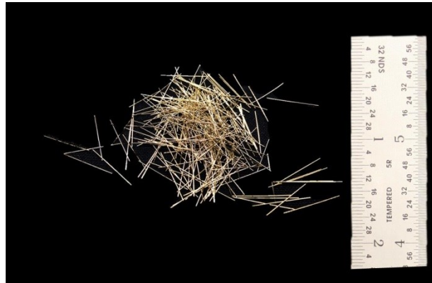
Figure 14. Photo. of the steel fiber reinforcement used in U-C.
