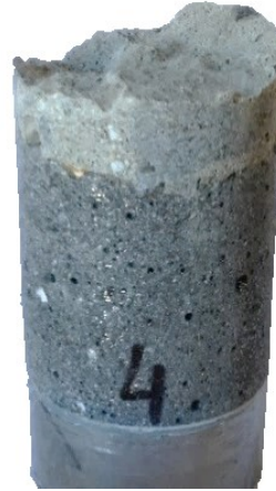
Figure 109. Photo. Substrate failure mode in direct tension pull-off tests.
