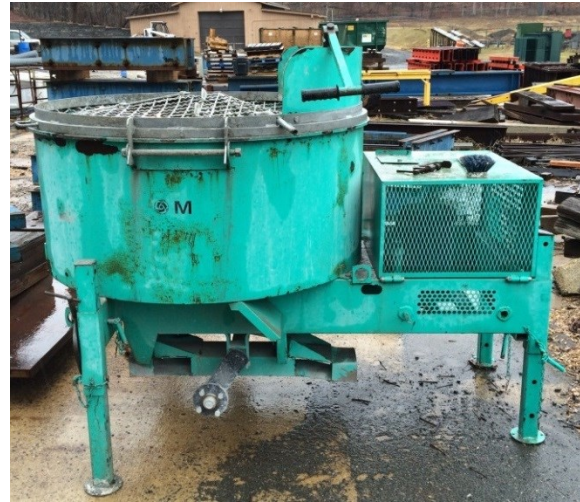
Figure 20. Photo. Large pan-style mixer with orbital mixing action for UHPC batches up to 4.0 ft 3 (0.11 m 3 ).
