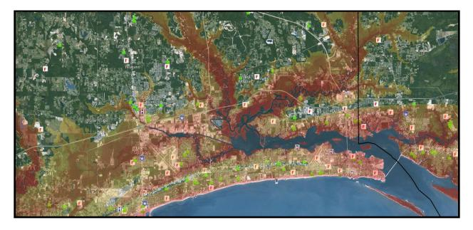
Figure 11: Vulnerability of critical facility under combined effect of Sea Level Rise and Storm Surge (Developed using NOAA Digital Coast Tool)
