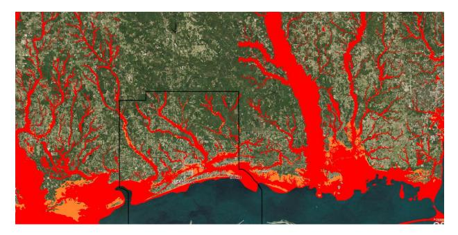
Figure 7(a): Existing FEMA Flood Zone with 1% probability (100 year return period) without Sea Level Rise [Map developed using NOAA web based software)
