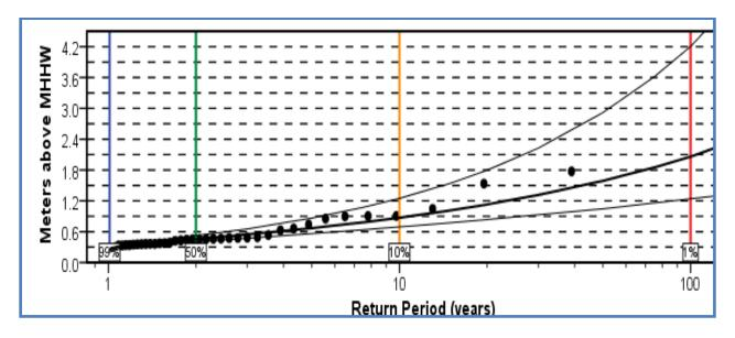
Figure 6: Projection of MHHW for different return period at Bay Waveland (Station No. 87437) [Extracted from NOAA Tides and Currents]
