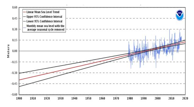
Figure 5: Mean Sea Level Trend for the tide station at Bay Waveland (Station No. 87437) [Extracted from NOAA Tides and Currents Website]
