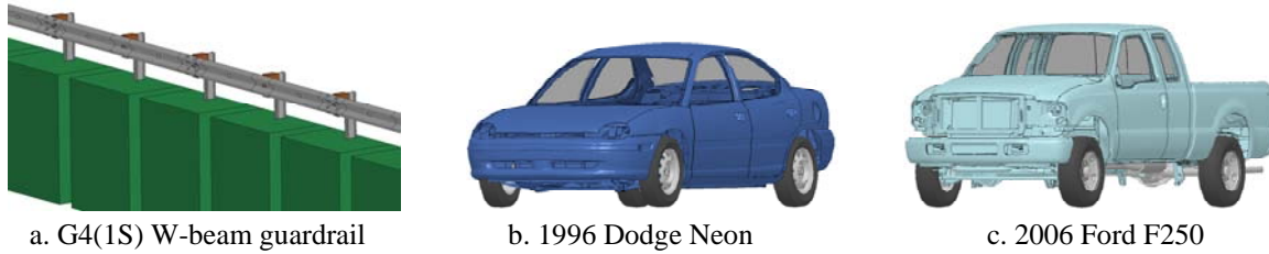
Fig. 1.4: FE models of a G4(1S) guardrail, a small passenger car, and a large pickup truck.
