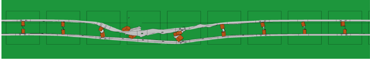
Fig. 4.91: Maximum dynamic deflection of the backside of the lowered backside 29-inch guardrail on a 2.5H:1V slope at 62 mph (100 km/hour) and 25° and impacted by a Ford F250.
