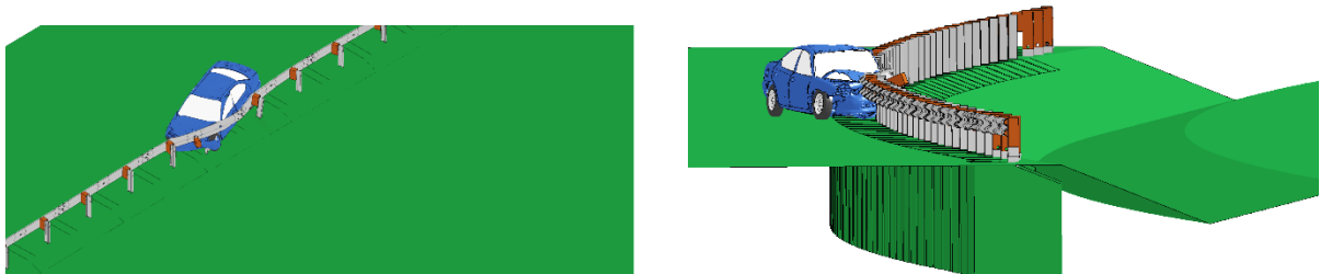
Fig. 4.117: Simulations of Dodge Neon impacting the front-side, convex horizontal curvature, 31-inch guardrail on a 2.5H:1V slope at 62 mph (100 km/hour) and 25°.
