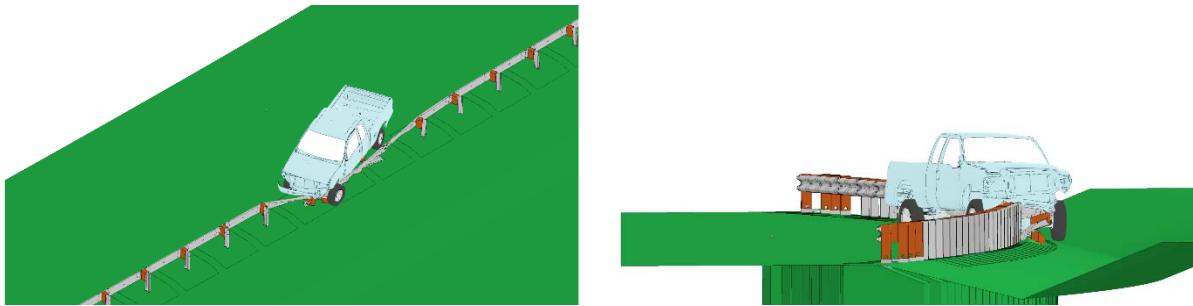
Fig. 4.132: Simulations of Ford F250 impacting the front-side, concave horizontal curvature, 29-inch guardrail on a 2.5H:1V slope at 62 mph (100 km/hour) and 25°.
