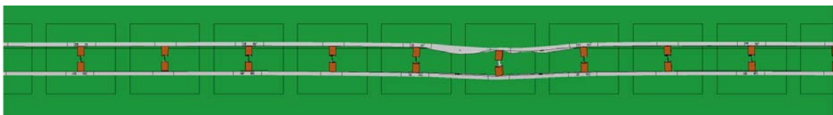
Fig. 4.86: Maximum dynamic deflection of the backside of the lowered backside 29-inch guardrail on a 2.5H:1V slope at 62 mph (100 km/hour) and 25° and impacted by a Dodge Neon.
