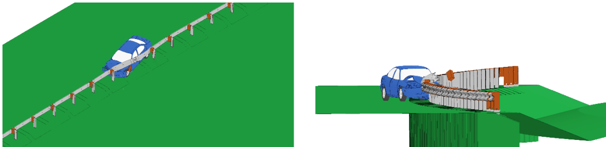
Fig. 4.107: Simulations of Dodge Neon impacting the front-side, convex horizontal curvature 29-inch guardrail on a 2.5H:1V slope at 62 mph (100 km/hour) and 25°.
