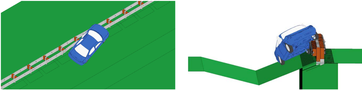
Fig. 4.87: Simulations of the Dodge Neon impacting the backside of the lowered backside 29-inch guardrail on a 2.5H:1V slope at 62 mph (100 km/hour) and 25°.
