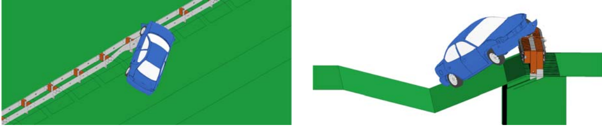
Fig. 4.47: Simulations of Dodge Neon impacting the backside 29-inch double-faced guardrail on a 2.5H:1V slope at 62 mph (100 km/hour) and 25°.
