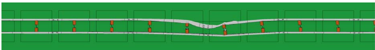
Fig. 4.96: Maximum dynamic deflection of the backside of the lowered backside 31-inch guardrail on a 2.5H:1V slope at 62 mph (100 km/hour) and 25^\circ and impacted by a Dodge Neon.
