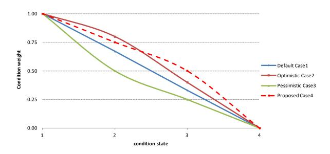
Figure 2.2. Cases for assignment of element condition weights
