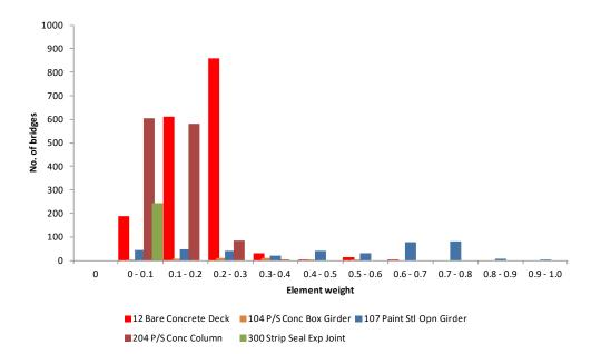
Figure 2.4. Variation in the weights based on element long-term cost for sample bridge elements.
