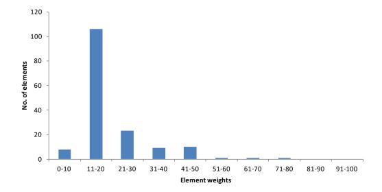
Figure 2.5. Variation in the weights (0-99) based on replacement cost, long-term cost, and hazard risk for bridge elements.
