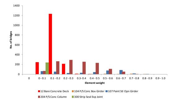
Figure 2.3. Variation in the weights based on element replacement cost for sample bridge elements.
