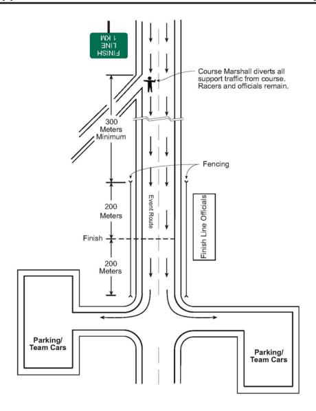
The race course is closed to public travel. Non-race traffic is detoured around the closed highway section using standard detour signing per the MUTCD.
