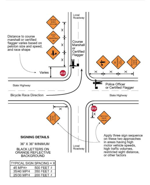
Race Turns Left Off State Highway and Onto Local Roadway With Stop-Controlled Approaches
