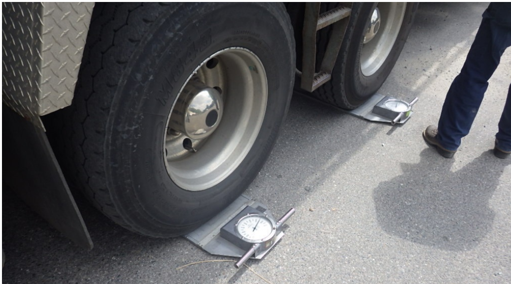
Figure 5: State highway patrol certified portable crane scales used to verify vehicle weight for each test
