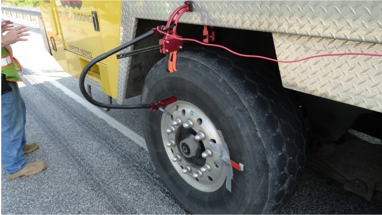
Figure 6: Autoclicker setup to measure wheel rotations for data analysis
