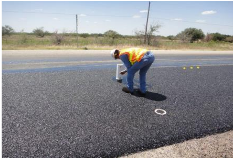
Figure 29. Water Flow Testing on US 183 Fine PFC.
