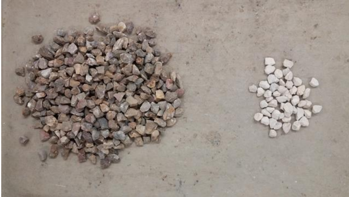
Figure 10. Remaining \frac{3}{8} -Inch Materials after ACV Test from Original 50/50 Blend of Fordyce Gravel and Beckman Limestone.
