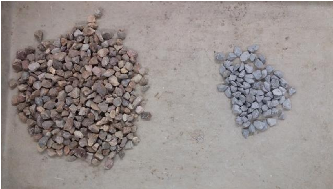
Figure 11. Remaining \frac{3}{8} -Inch Materials after ACV Test from Original 50/50 Blend of Fordyce Gravel and Beckman Limestone.
