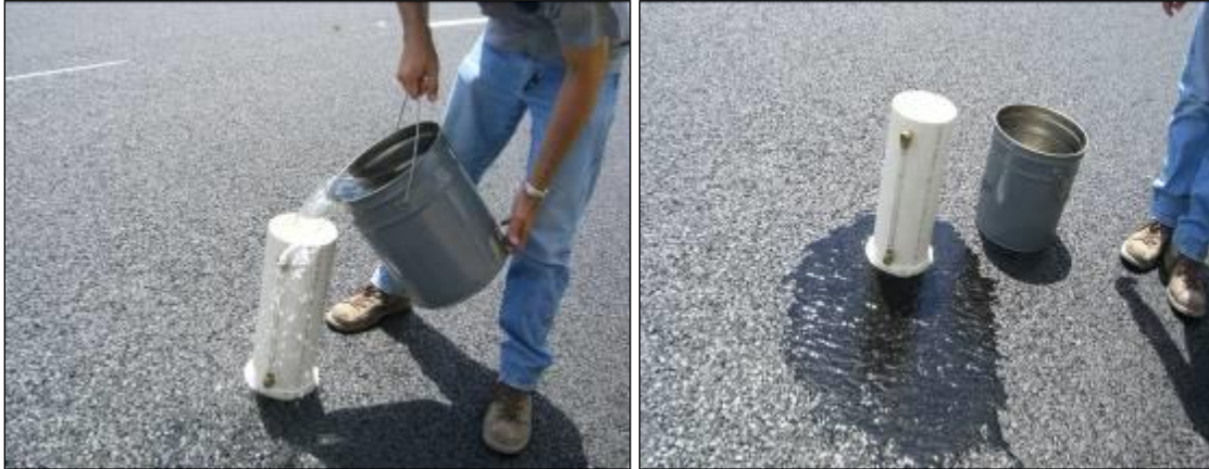
Figure 25. Test Method Tex-246-F, Field Water Flow Test.
