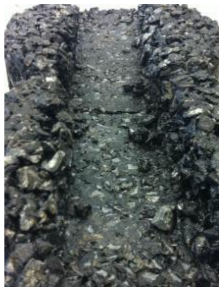
Figure 37. HWTT Specimen Showing Excessive Rutting and Minimal Stripping.
