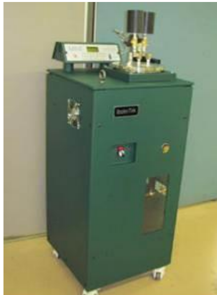
Figure 12. Moisture-Induced Stress Tester Equipment.
