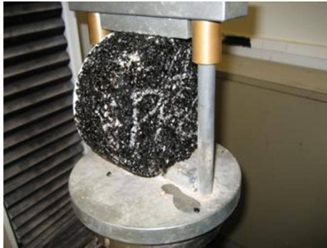
Figure 17. IDT Strength Test Setup.
