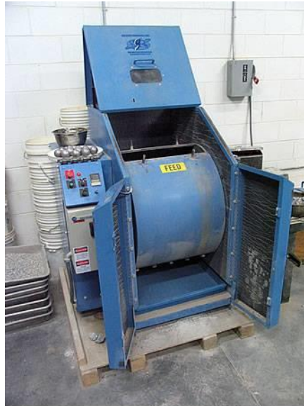
Figure 13. Los Angeles Abrasion Testing Equipment ( www.pavementinteractive.org ).
