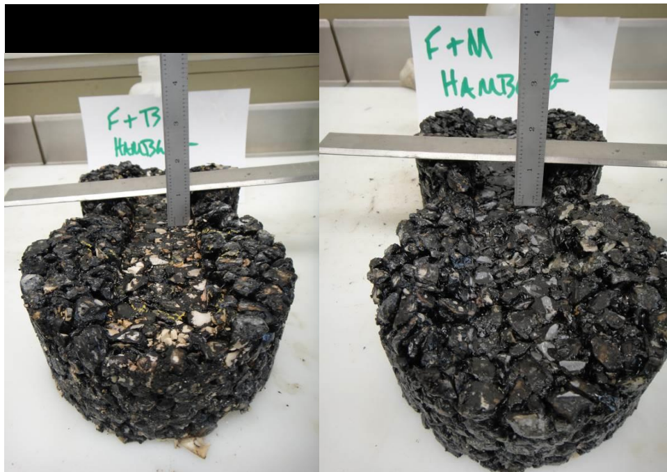
(a) Failed at 13,750 cycles
