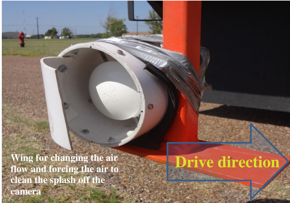
Figure 52. Splash Protect Cover's Back View (Extra Wing Will Force the Air to Clean the Lens).
