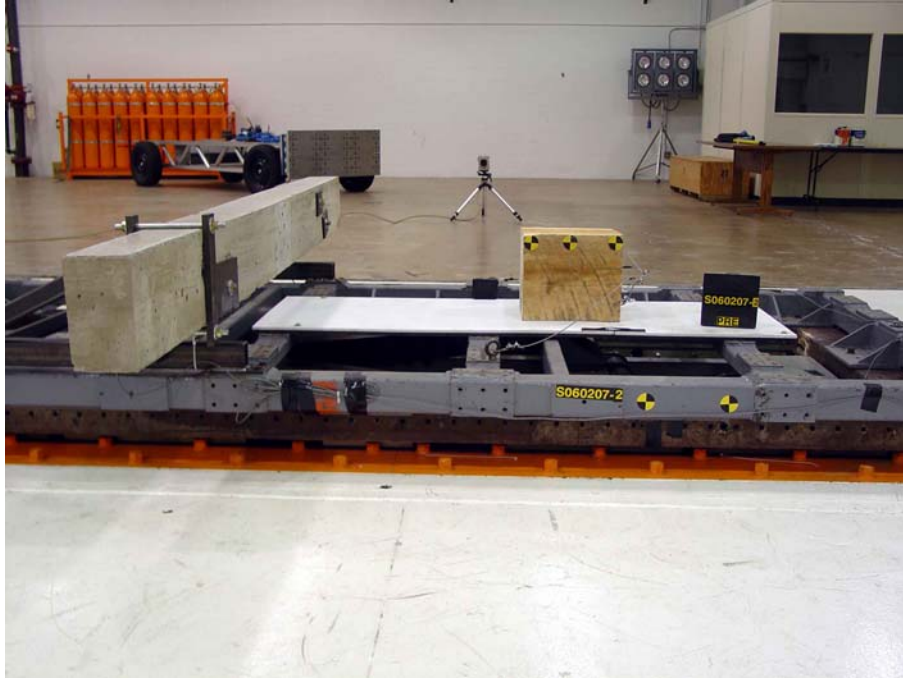
Figure 56 Impact test set-up for concrete beam without I-Lam panel protection (Concrete Beam)
