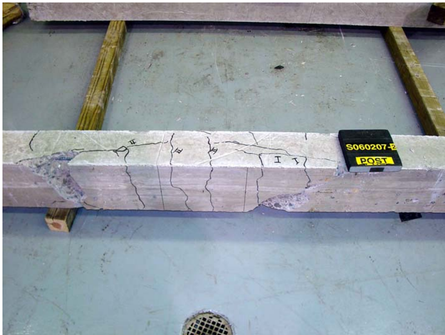
(b) Marked crack and/or damage
