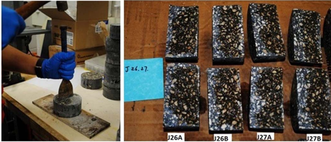
Figure 5.3: Illustration of splitting slices and spraying 0.1N AgNO 3 at the cross section as indication of chloride ion penetration depth
