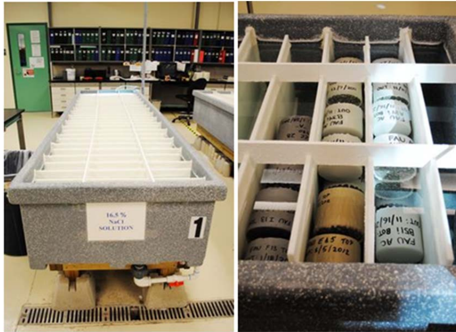
Figure 4.3: Exposure tank for bulk diffusion test at FDOT
