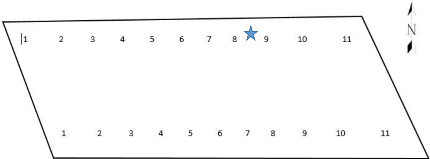
Figure 4 location of shaker (star) on bridge – 26.4 ft from east side of bridge, mode 4 of MIDAS model.
