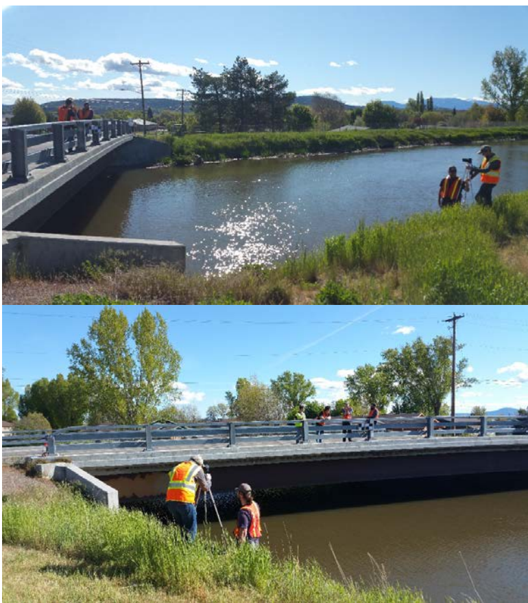
Figure 12. Visual sensor placed northeast of bridge, perpendicular to the antinode and target.
