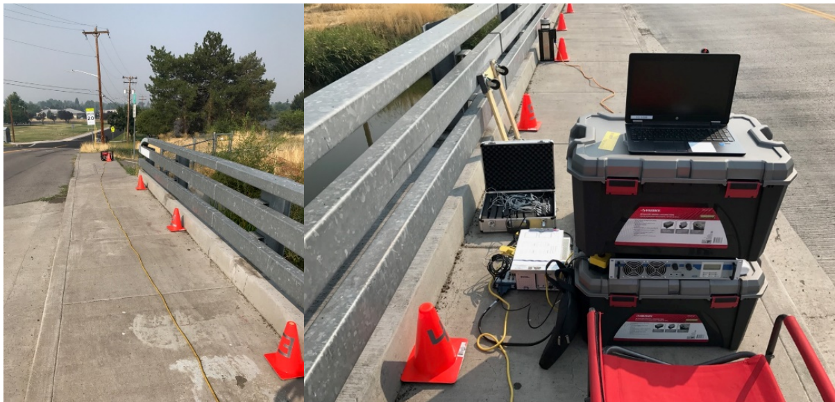
Figure 3.2: Generator located off of structure and storage totes used as workstation.
