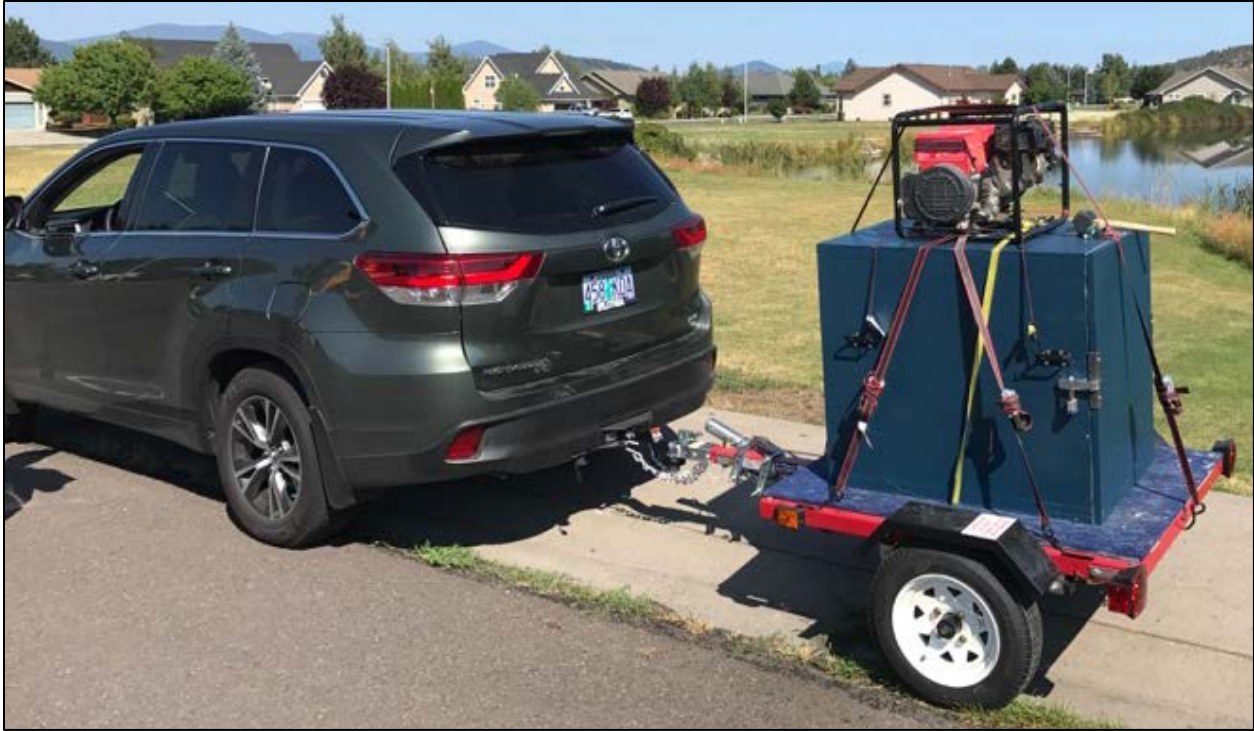
Figure 2.6: RDSETGO Iteration 3 with equipment box on 3.5'x4' trailer.
