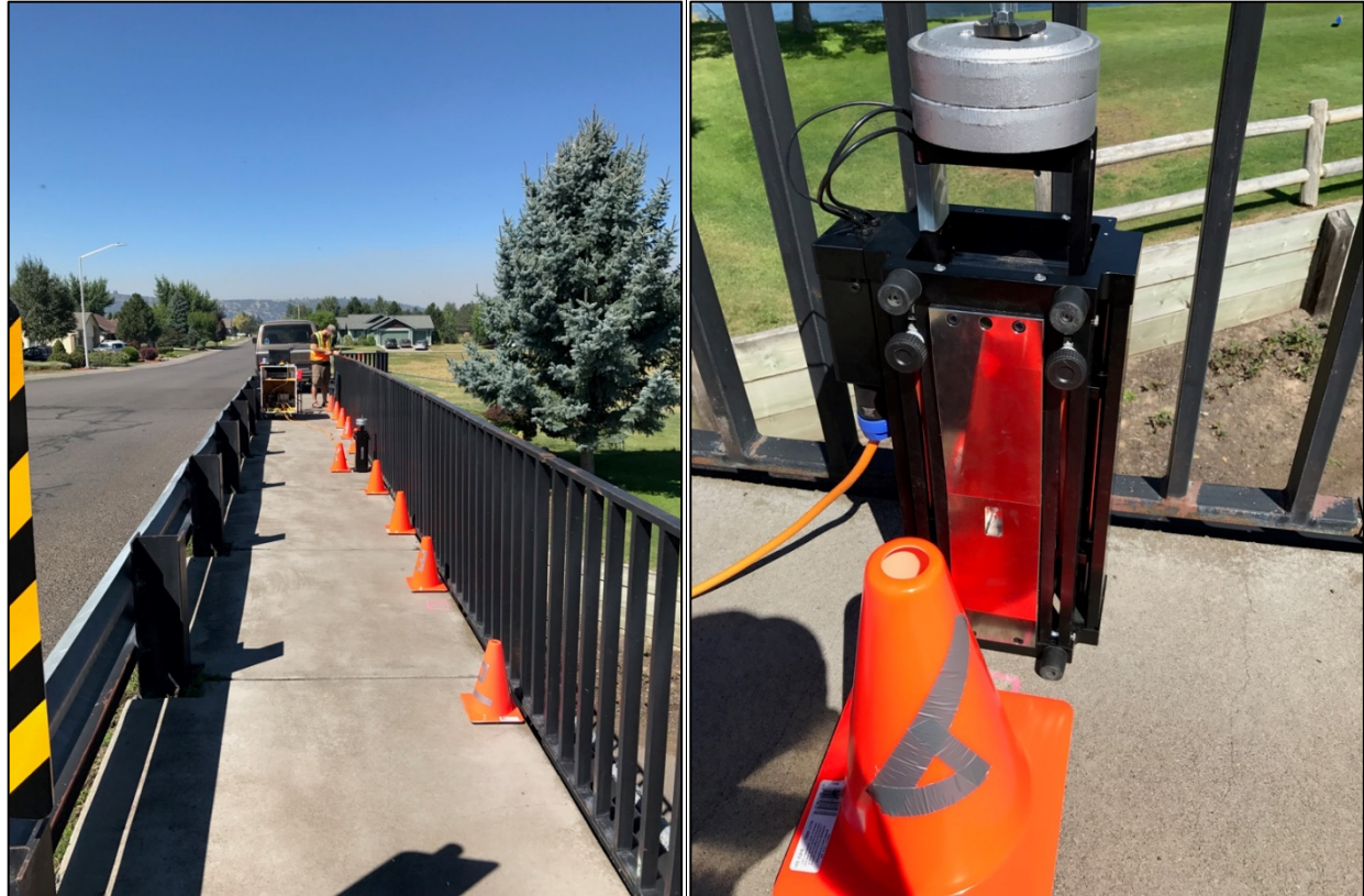
Figure 2.7: RDSETGO Iteration 3 with equipment box on carpet dolly and shaker in fixed-body mode.
