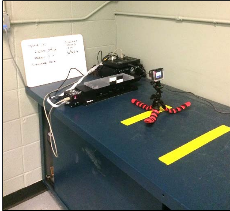
Fig.1 Testing setup for VVS testing using the shake table.
