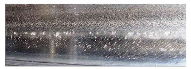
Figure 1. Wheel Tread Surface with RCF Cracks
