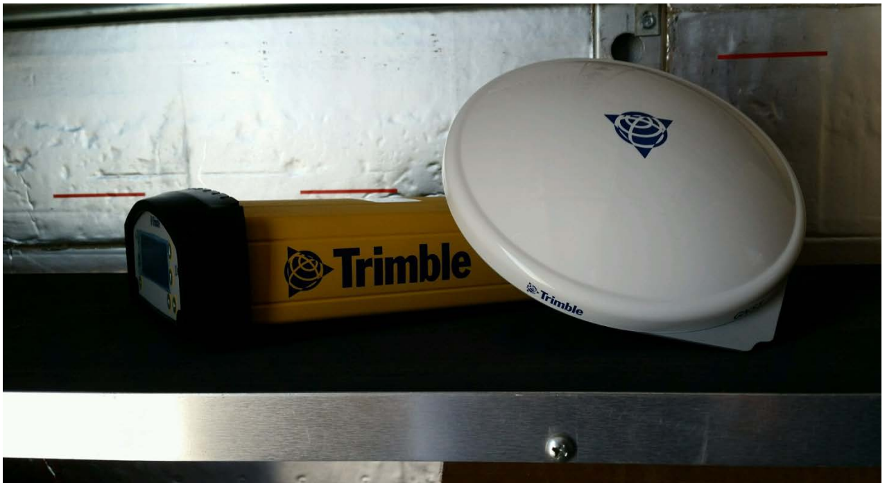
Figure 6. Zephyr Model 2 GPS Antenna/SPS555H GPS Receiver
