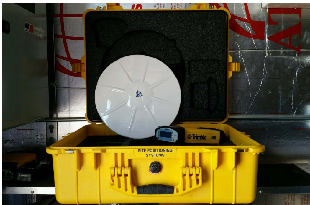
Figure 7. Zephyr Geodetic Model 2 GPS Antenna/SPS855 GPS Receiver
