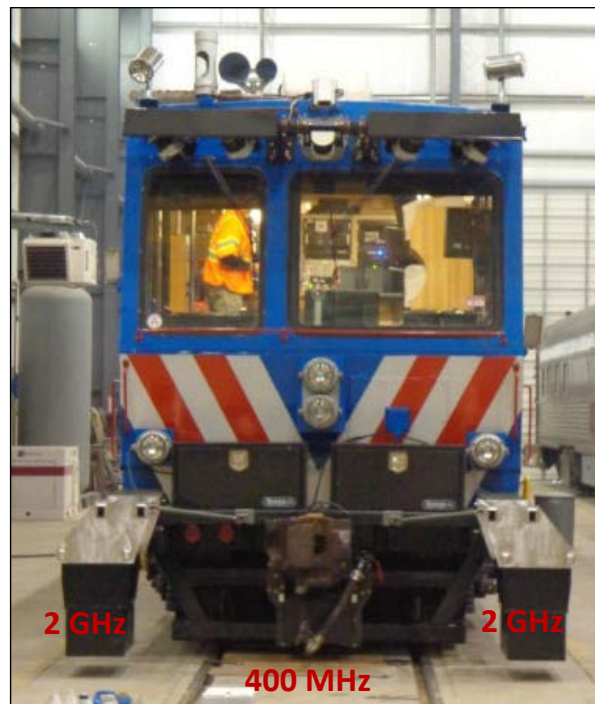
Figure 20. Antenna Deployment and Shielded Housings on the Rear of the T18 Vehicle
