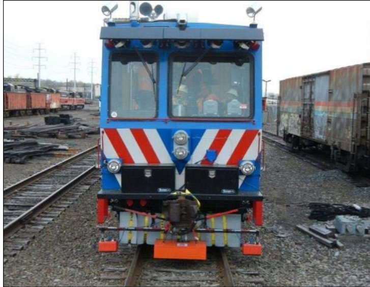
Figure 24. System 3 Installation on Rear of T18 Vehicle Showing Antennas at Track Center and Shoulders and Foam Barrier
