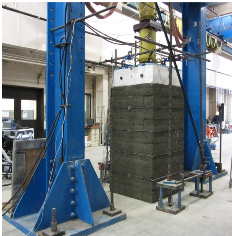
Figure 21. Photo. TF-10 PT setup with reaction frame.
