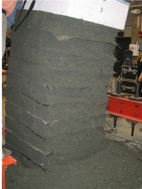
Figure 28. Photo. Tilting of the footing during TF-4 testing.
