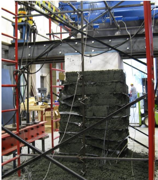
Figure 35. Photo. TF-3 at failure with S_v = 7\frac{5}{8} inches, T_f = 2,400 lb/ft, and 21A material.
