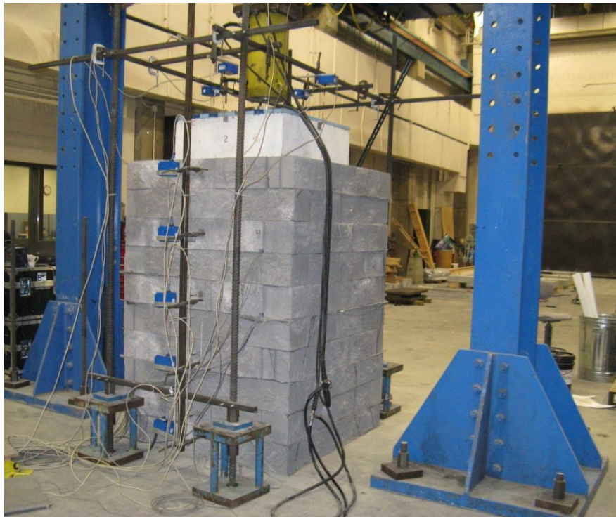
Figure 20. Photo. TF-6 PT setup with reaction frame.
