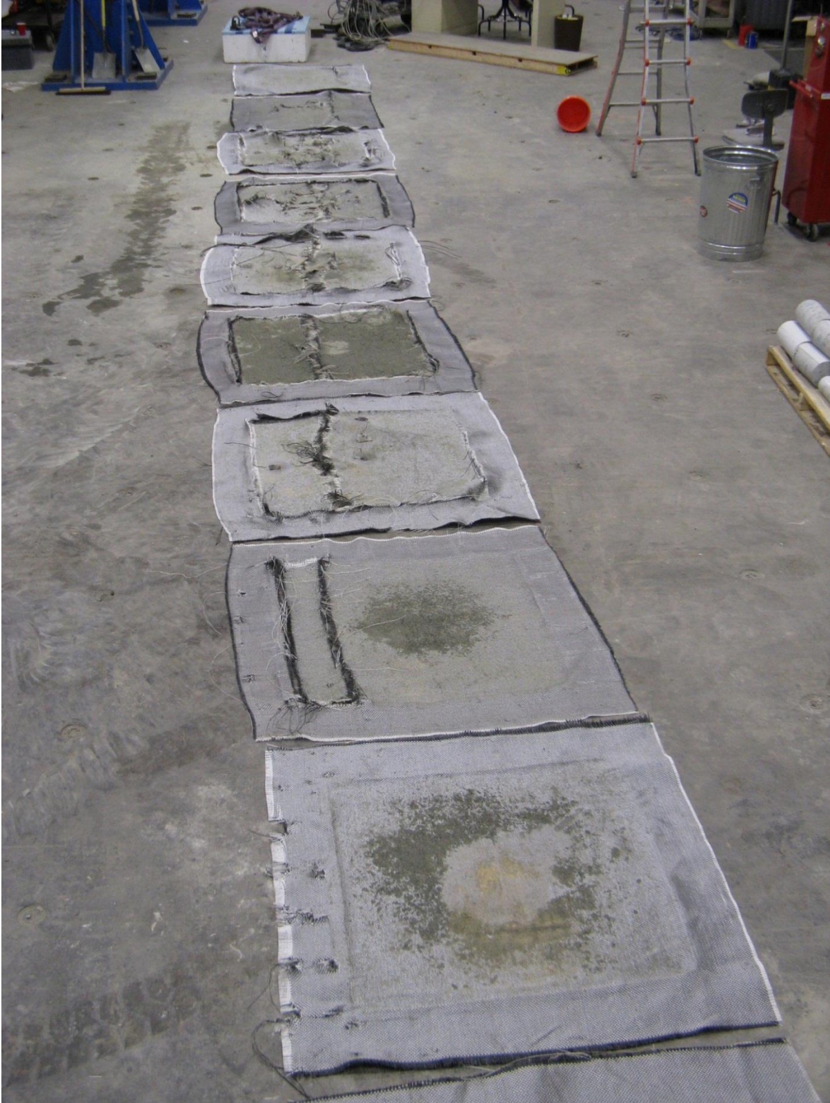
Figure 38. Photo. Rupture pattern for geotextiles in TF-6 ( q_{ult,emp} = 43,828 psf); the lowest layer of reinforcement is the closet fabric in the picture.
