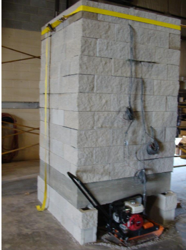
Figure 16. Photo. DC-1 GRS PT (before testing).
