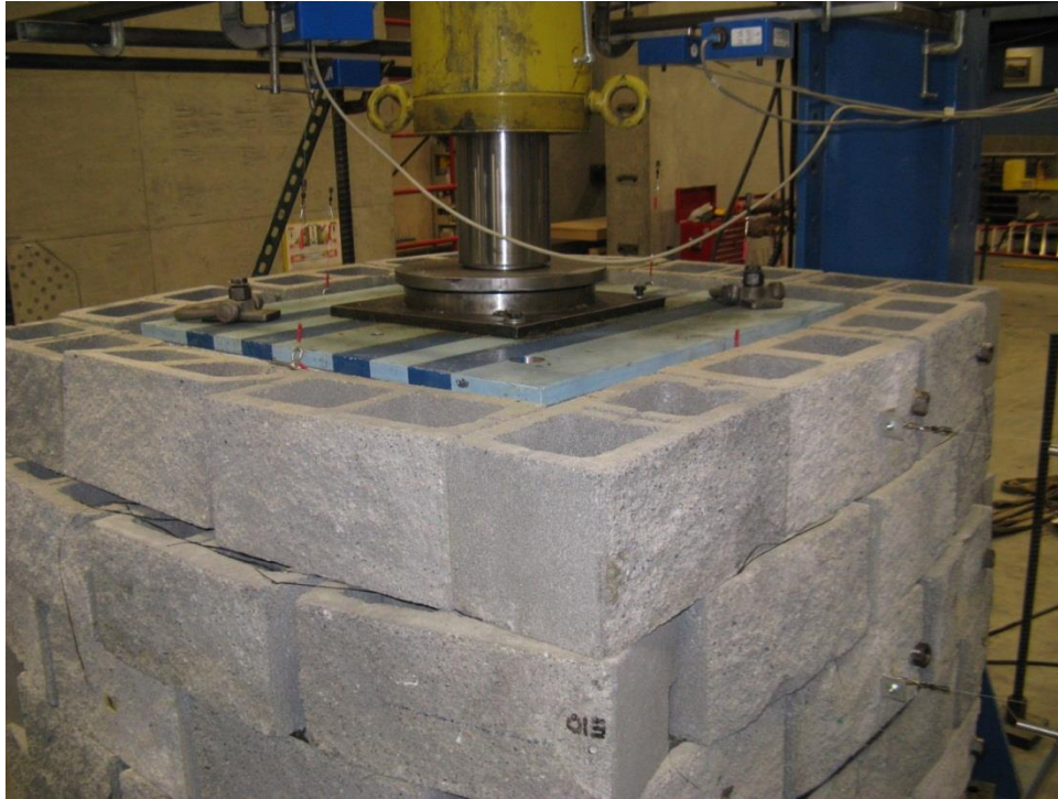
Figure 23. Photo. Spherical bearing to apply load to the footing on the GRS composite.
