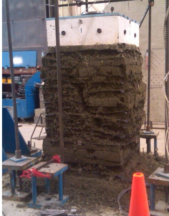
Figure 34. Photo. TF-11 at failure with S_v = 3\text{-}13/16 inches, T_f = 1,400 lb/ft, and 21A material.
