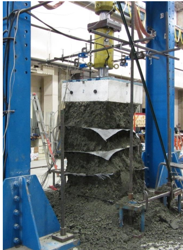
Figure 37. Photo. TF-10 at failure with S_v = 15\frac{1}{4} inches, T_f = 4,800 lb/ft, and 21A material.
