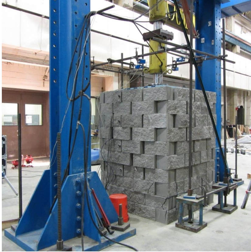
Figure 22. Photo. TF-9 at failure with reaction frame.
