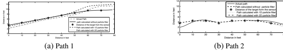
Fig. 7. Comparing the actual path of a target across the sensor array, and the trajectory we computed. We drove our target along two different paths, and tested the three versions of trajectory mapping to approximate the target's path.
