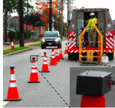
Fig. 2. Our sensornet system deployed in a work zone. The motes are mounted on safety cones, which are placed as per the MUTCD.
