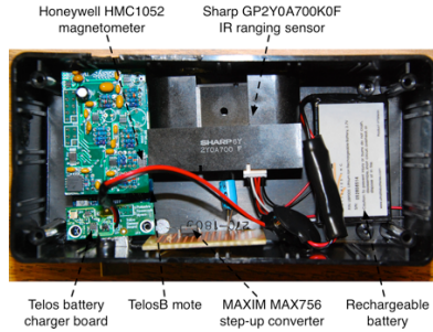
Fig. 3. Our sensor node includes a TelosB mote with a ranging sensor and a magnetometer
